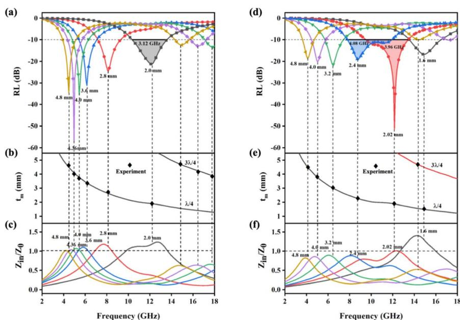
Fig. 6 2D schematic of the EMW absorption performance of (a) PIC/rGO and (d) PIC/CNT at 2–18 GHz. Simulated thickness *versus* peak frequency of (b) PIC/rGO and (e) PIC/CNT at 2–18 GHz. Relationship between EMW frequencies of (c) PIC/rGO and (f) PIC/CNT at 2–18 GHz and  $Z_{\text{in}}/Z_0$ .
