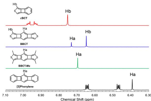
Fig. 6 <sup>1</sup>H NMR spectra of cBCT (red), BBCT (blue), BBCT-Me (green), and [3]phenylene (black) in acetone-*d*<sub>6</sub> at 25 °C.
