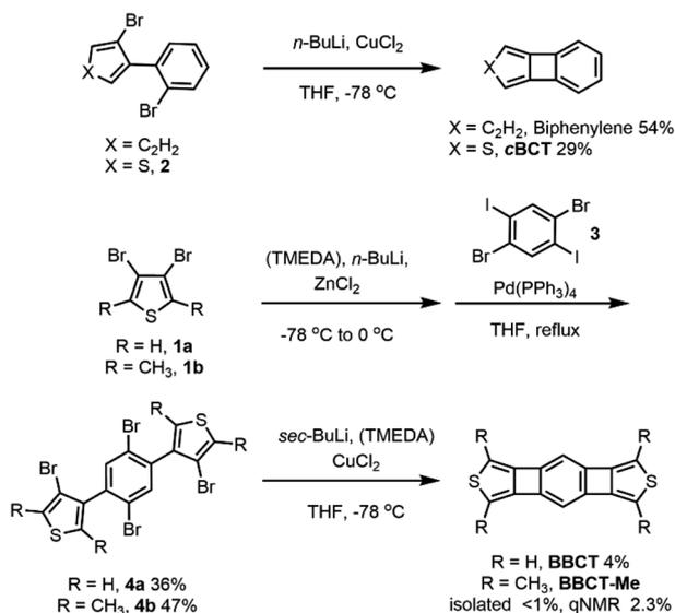
Scheme 1 Synthesis of biphenylene, **cBCT**, **BBCT**, and **BBCT-Me**.
