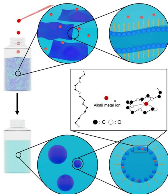
**Fig. 1** Schematic illustration of the present detection method with the deformation of the HL phase. The metal ions (red dots) bind with the oligo ethylene glycol moieties (blue parts) of the amphiphiles. The complexation breaks the bilayers, and the birefringence disappears.
