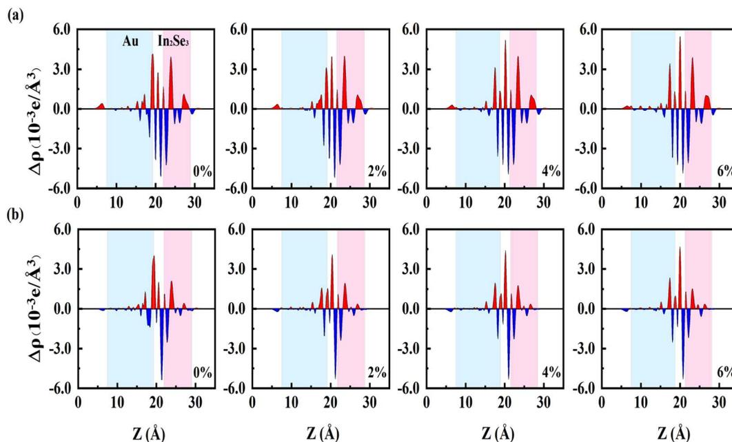
Fig. 2 Planar average charge density difference  $\Delta\rho$  along the  $z$ -direction of (a) Up- $\text{In}_2\text{Se}_3/\text{Au}$  and (b) Dw- $\text{In}_2\text{Se}_3/\text{Au}$  heterostructures under biaxial strain. Red and blue represent the accumulation and depletion of electrons, respectively.
