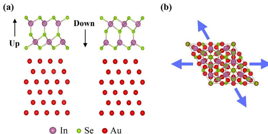
Fig. 1 (a) The initial configuration of the monolayer  $\text{In}_2\text{Se}_3$ /metal heterostructure system in both the upward and downward directions of  $\text{In}_2\text{Se}_3$  (Up- $\text{In}_2\text{Se}_3$ /Au and Dw- $\text{In}_2\text{Se}_3$ /Au). (b) In-plane biaxial tensile strain is depicted.
