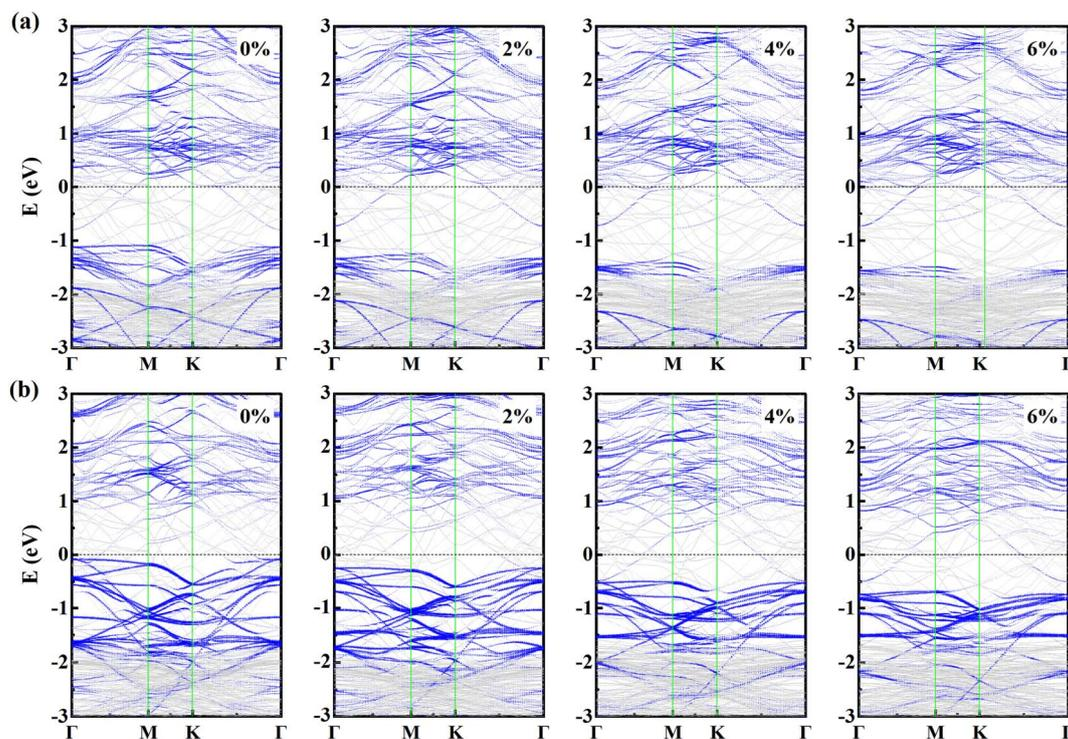
Fig. 4 Band structure of  $\text{In}_2\text{Se}_3$  in (a) Up- $\text{In}_2\text{Se}_3/\text{Au}$  and (b) Dw- $\text{In}_2\text{Se}_3/\text{Au}$  contact systems under biaxial tensile strain. The gray line indicates the energy band structure of the interfacial system. The blue line indicates the energy band structure of the ML  $\text{In}_2\text{Se}_3$  projection, whose weight is represented by the size of the dot. The Fermi level is set to zero energy and is denoted by the dashed line.
