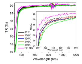
Fig. 5 Transmittance rate (TR) of the PC and Al<sub>2</sub>O<sub>3</sub>/PC films.
