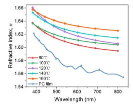
Fig. 6 Refractive index of  $A_2O_3$  films deposited at different temperature and the PC film.
