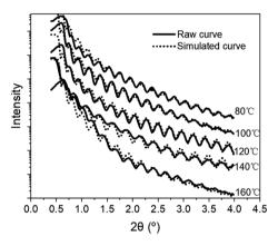
Fig. 4 Experimental and simulated XRR curves for samples deposited between 80 and 160  $^{\circ}$ C.
