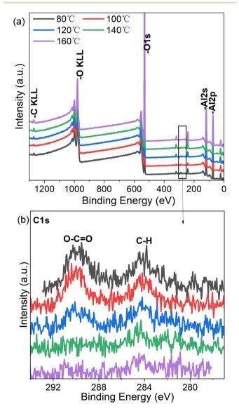
Fig. 3 XPS spectra of  $\mathrm{Al_2O_3}$  deposited on Si substrate at different temperatures.
