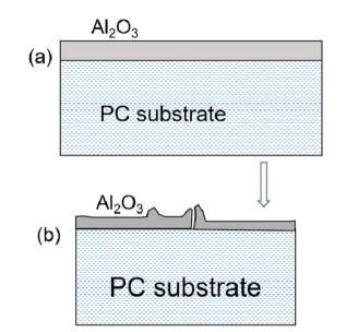
Fig. 8 (a)  $Al_2O_3$  ALD film deposited at elevated temperature on PC substrate. (b)  $Al_2O_3$  film buckles upon cooling from deposition temperature to room temperature.
