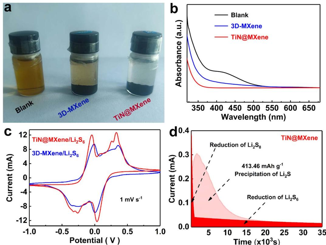
Fig. 4 (a) Photograph of  $\text{Li}_2\text{S}_6$  adsorption test with 3D-MXene and TiN@MXene composites. (b) Ultraviolet-visible absorption spectra of  $\text{Li}_2\text{S}_6$  solution and ones after adding 3D-MXene and TiN@MXene. (c) CV curves of symmetrical batteries using 3D-MXene and TiN@MXene electrodes. (d) Constant potential discharge curve of the  $\text{Li}_2\text{S}$  deposition tests using TiN@MXene as substrate.
