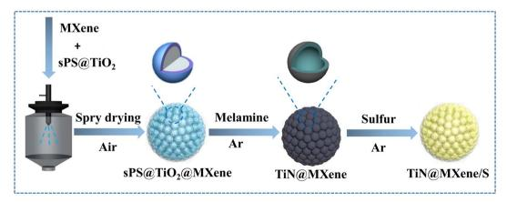
Fig. 1 Schematic illustration of the synthesis process of TiN@MXene/S.
