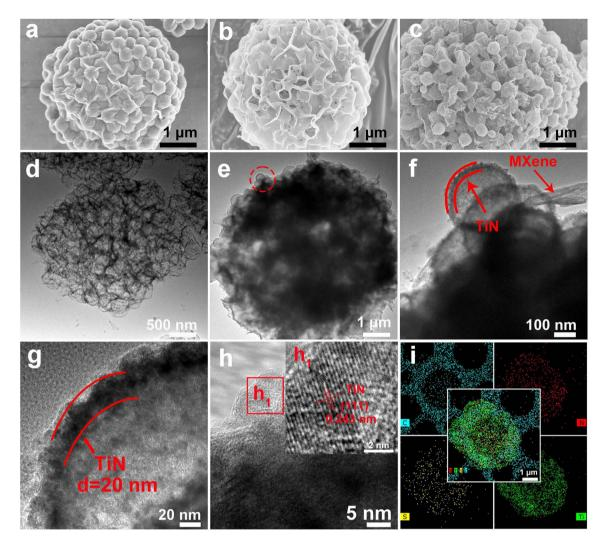
Fig. 2 SEM images of (a) sPS@MXene, (b) 3D-MXene, (c) TiN@MXene. (d) TEM image of 3D-MXene. (e)–(g) TEM images and (h), ( $h_1$ ) high-resolution TEM image of TiN@MXene. (i) Mapping image of TiN@MXene/S and the corresponding elemental mappings of C, Ti, N, and S.
