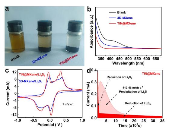
Fig. 4 (a) Photograph of  $\text{Li}_2S_6$  adsorption test with 3D-MXene and TiN@MXene composites. (b) Ultraviolet-visible absorption spectra of  $\text{Li}_2S_6$  solution and ones after adding 3D-MXene and TiN@MXene. (c) CV curves of symmetrical batteries using 3D-MXene and TiN@MXene electrodes. (d) Constant potential discharge curve of the  $\text{Li}_2S$  deposition tests using TiN@MXene as substrate.
