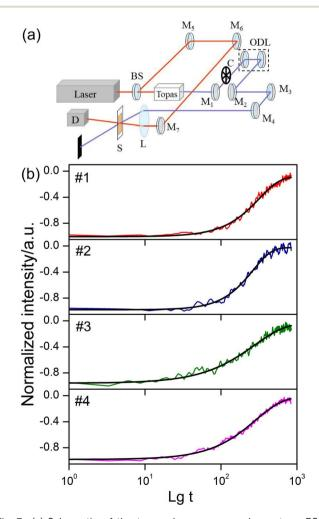
Fig. 7 (a) Schematic of the two-colour pump-probe system. BS is beam splitter;  $M_1-M_7$  are mirrors; C is chopper; L is convex len; S is sample; and D is photodiode detector; (b) two-color pump-probe dynamics for sample solutions at excitation of 410 nm.
