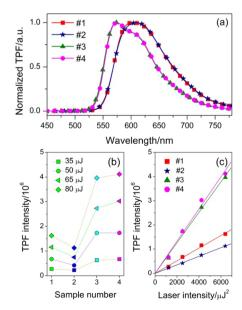
Fig. 5 (a) Normalized TPF spectra of #1–#4 (5  $\times$  10<sup>-4</sup> M); (b) TPF intensity of #1–#4 at different laser intensities over a range of 35–80  $\mu$ J; (c) TPF intensity as a function of the square of laser intensity.
