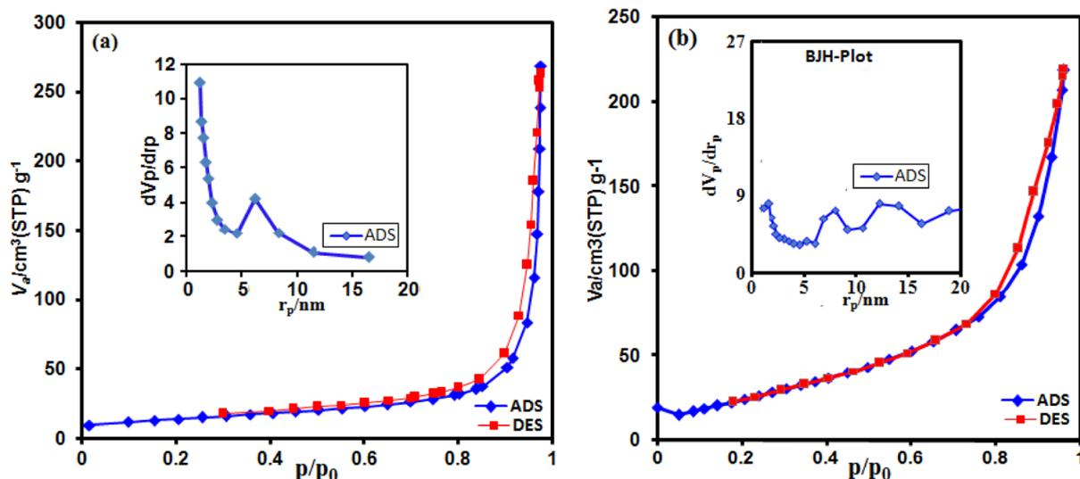
Fig. 9  $\text{N}_2$  adsorption-desorption isotherms of (a)  $\text{C}_3\text{N}_4$  and (b)  $\text{g-C}_3\text{N}_4/\text{CoFe}_2\text{O}_4$  nanocomposite. The insets are the pore size distribution curves.
