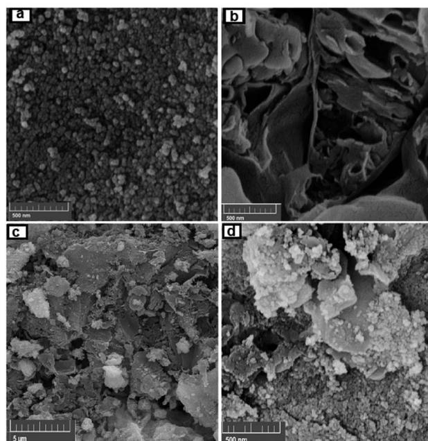
Fig. 3 FE-SEM images of (a) CoFe<sub>2</sub>O<sub>4</sub>, (b) g-C<sub>3</sub>N<sub>4</sub>, and (c and d) the g-C<sub>3</sub>N<sub>4</sub>/CoFe<sub>2</sub>O<sub>4</sub> hybrid nanocomposite.
