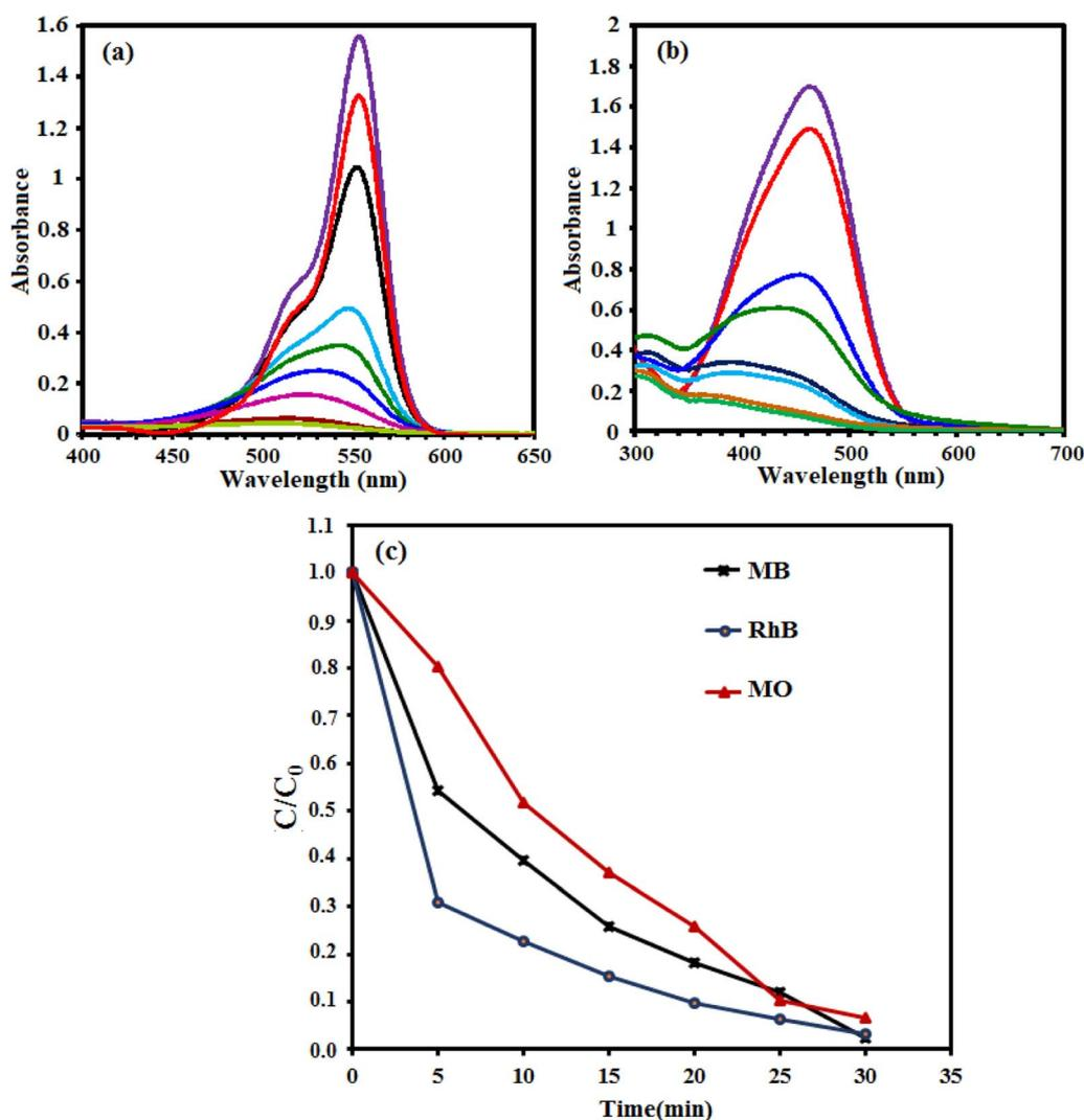
Fig. 12 The UV-vis absorption spectra changes of (a) rhodamine B (RhB), (b) methyl orange (MO), and (c) comparison of sonodegradation efficiency of dyes as a function of time over the g-C<sub>3</sub>N<sub>4</sub>/CoFe<sub>2</sub>O<sub>4</sub> nanocomposite. Conditions: [dye] = 25 mg L<sup>-1</sup>, 50 mL; [cat.] = 0.66 g L<sup>-1</sup>; [H<sub>2</sub>O<sub>2</sub>] = 0.1 mol L<sup>-1</sup>, 1 mL; at room temperature and natural pH = 7.
