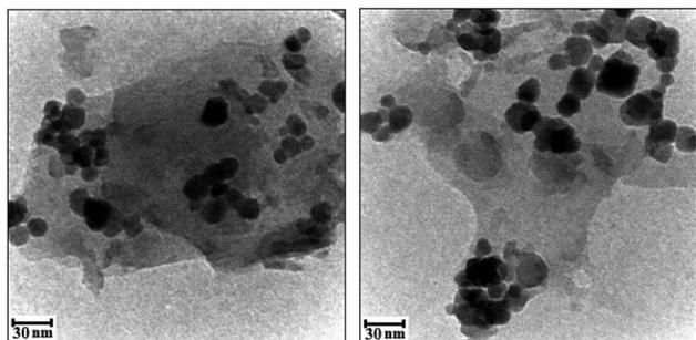
Fig. 5 The TEM images of the  $g\text{-C}_3\text{N}_4/\text{CoFe}_2\text{O}_4$  nanocomposite.
