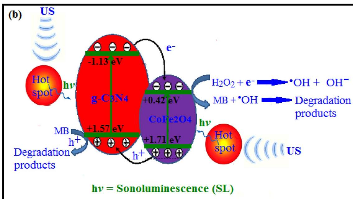
Fig. 13 (a) Effects of different scavengers on the sonocatalytic degradation of MB. Conditions: [MB] = 25 mg L<sup>-1</sup>, 50 mL; [cat.] = 0.66 g L<sup>-1</sup>; [H<sub>2</sub>O<sub>2</sub>] = 0.1 mol L<sup>-1</sup>, 1 mL; [scavenger] = 0.1 mol L; at room temperature and natural pH = 7. (b) Schematic illustration of the possible sonocatalytic mechanism of the  $g-C_3N_4/CoFe_2O_4$  nanocomposite under ultrasound irradiation.
