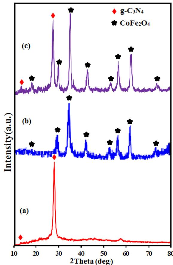
Fig. 2 XRD patterns of (a) g-C<sub>3</sub>N<sub>4</sub>, (b) CoFe<sub>2</sub>O<sub>4</sub> and (c) g-C<sub>3</sub>N<sub>4</sub>/CoFe<sub>2</sub>O<sub>4</sub> samples.
