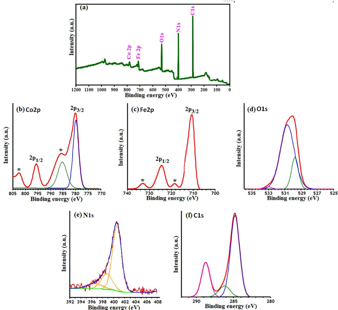
Fig. 6 XPS of the  $g\text{-C}_3\text{N}_4/\text{CoFe}_2\text{O}_4$  nanocomposite: (a) survey spectrum, (b) Co 2p spectrum, (c) Fe 2p spectrum, (d) O 1s spectrum, (e) N 1s spectrum and (f) C 1s spectrum.
