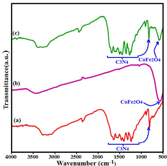
Fig. 1 FT-IR spectra of (a) C<sub>3</sub>N<sub>4</sub>, (b) CoFe<sub>2</sub>O<sub>4</sub> and (c) g-C<sub>3</sub>N<sub>4</sub>/CoFe<sub>2</sub>O<sub>4</sub> hybrid nanocomposite.
