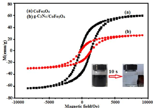
Fig. 8 Room-temperature magnetization curves of (a)  $\text{CoFe}_2\text{O}_4$  and (b)  $\text{g-C}_3\text{N}_4/\text{CoFe}_2\text{O}_4$  nanocomposite (inset: the magnetic separation of  $\text{g-C}_3\text{N}_4/\text{CoFe}_2\text{O}_4$  nanocomposite by a magnet).
