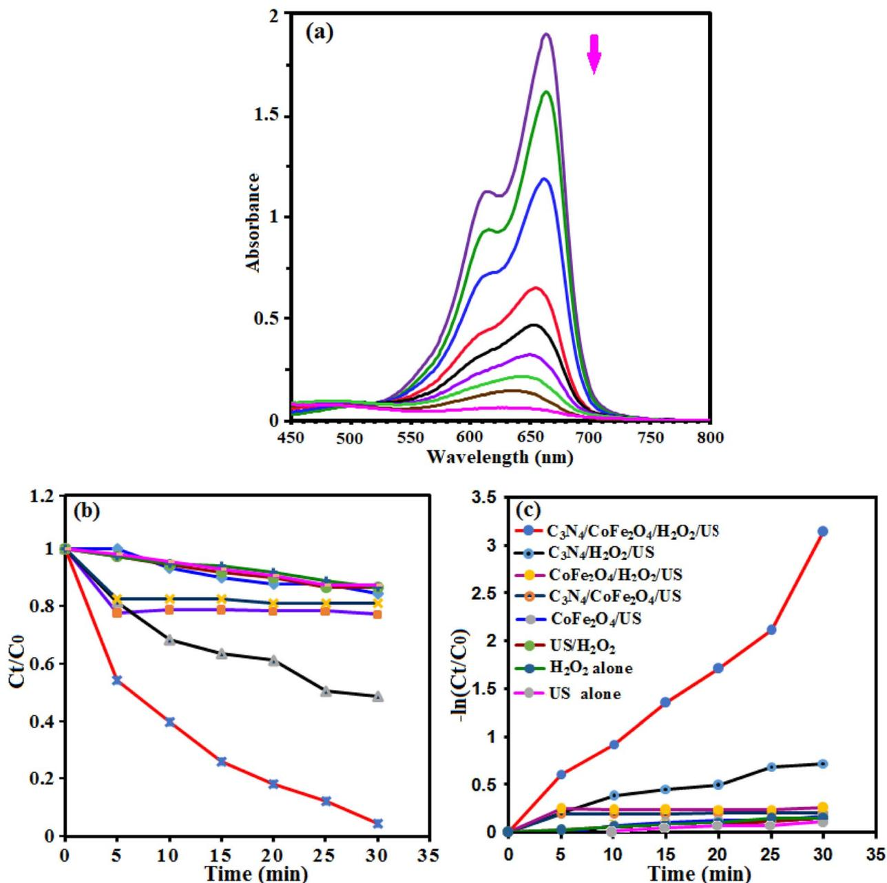
Fig. 10 (a) The UV-vis absorption changes, (b) concentration changes ( $C_t/C_0$ ), and (c) the pseudo-first-order plots of  $-\ln(C_t/C_0)$  as a function of irradiation time for MB sonodegradation in the presence of  $g\text{-C}_3\text{N}_4/\text{CoFe}_2\text{O}_4$  nanocomposite. Conditions:  $[\text{MB}]_0 = 25 \text{ mg L}^{-1}$ , 50 mL;  $[\text{H}_2\text{O}_2] = 0.1 \text{ mol L}^{-1}$ , 1 mL;  $[\text{cat.}] = 0.66 \text{ g L}^{-1}$  at room temperature and natural pH = 7.
