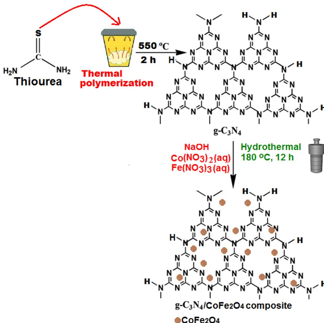
Scheme 1 The preparation process of the g-C<sub>3</sub>N<sub>4</sub>/CoFe<sub>2</sub>O<sub>4</sub> nanocomposite.
