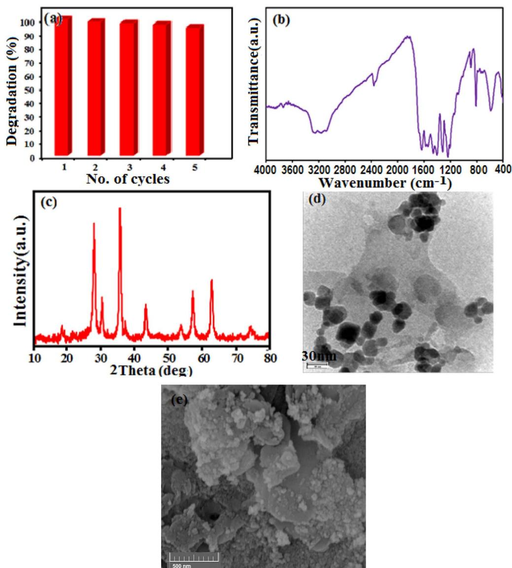
Fig. 15 (a) Cycling runs of  $\text{g-C}_3\text{N}_4/\text{CoFe}_2\text{O}_4$  nanocomposite in the sonodegradation of MB. Each run of photocatalytic reactions lasted for 30 min. (b) FT-IR spectrum, (c) XRD pattern and (d) TEM image (e) SEM image of the recovered nanocomposite after the 5th run.
