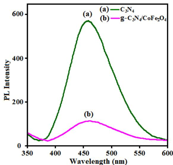
Fig. 14 PL spectra of (a) pure g-C<sub>3</sub>N<sub>4</sub> and (b) g-C<sub>3</sub>N<sub>4</sub>/CoFe<sub>2</sub>O<sub>4</sub> samples.
