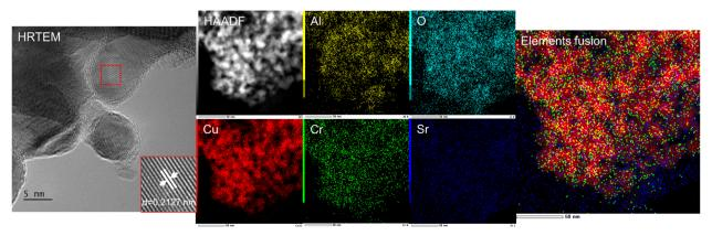
Fig. 3 HRTEM, HAADF, and EDS mapping images of CuCrSr/γ-Al<sub>2</sub>O<sub>3</sub> (elements fusion diagram was composed by Cu, Cr, and Sr).
