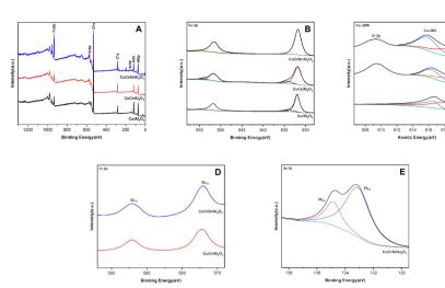
(A) XPS survey, (B) Cu 2p, (C) Cu LMM Auger, (D) Cr 2p, and (E) Sr 3d spectra of Cu-based catalysts after reduction.
