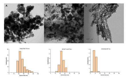
Fig. 2 TEM images of catalysts after reduction. ((A) Cu/Al<sub>2</sub>O<sub>3</sub>; (B) CuCr/Al<sub>2</sub>O<sub>3</sub>; (C) CuCrSr/Al<sub>2</sub>O<sub>3</sub>)
