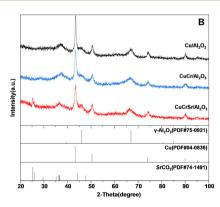
Fig. 1 XRD patterns of Cu/Al<sub>2</sub>O<sub>3</sub>, CuCr/Al<sub>2</sub>O<sub>3</sub> and CuCrSr/Al<sub>2</sub>O<sub>3</sub> after (A) calcination and (B) reduction.
