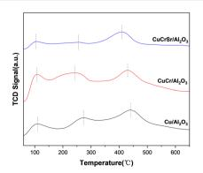
NH<sub>3</sub>-TPD profiles of Cu-based catalysts after reduction.
