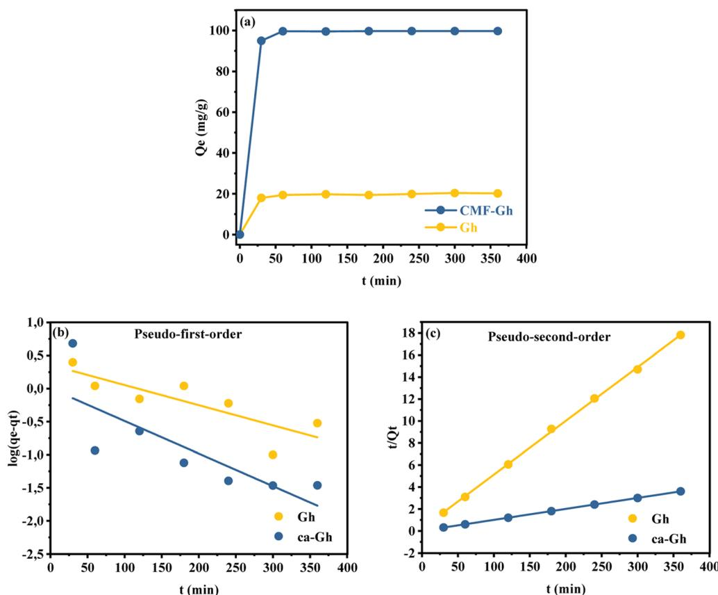
Fig. 7 (a) Experimental and (b and c) fitted data to two kinetic models for the adsorption of Cd<sup>2+</sup> by Gh and ca-Gh.
