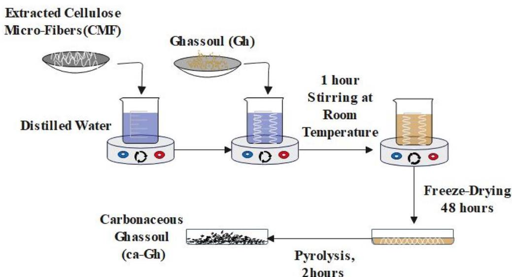
Fig. 1 Schematic representation of the synthesis of ca-Gh.
