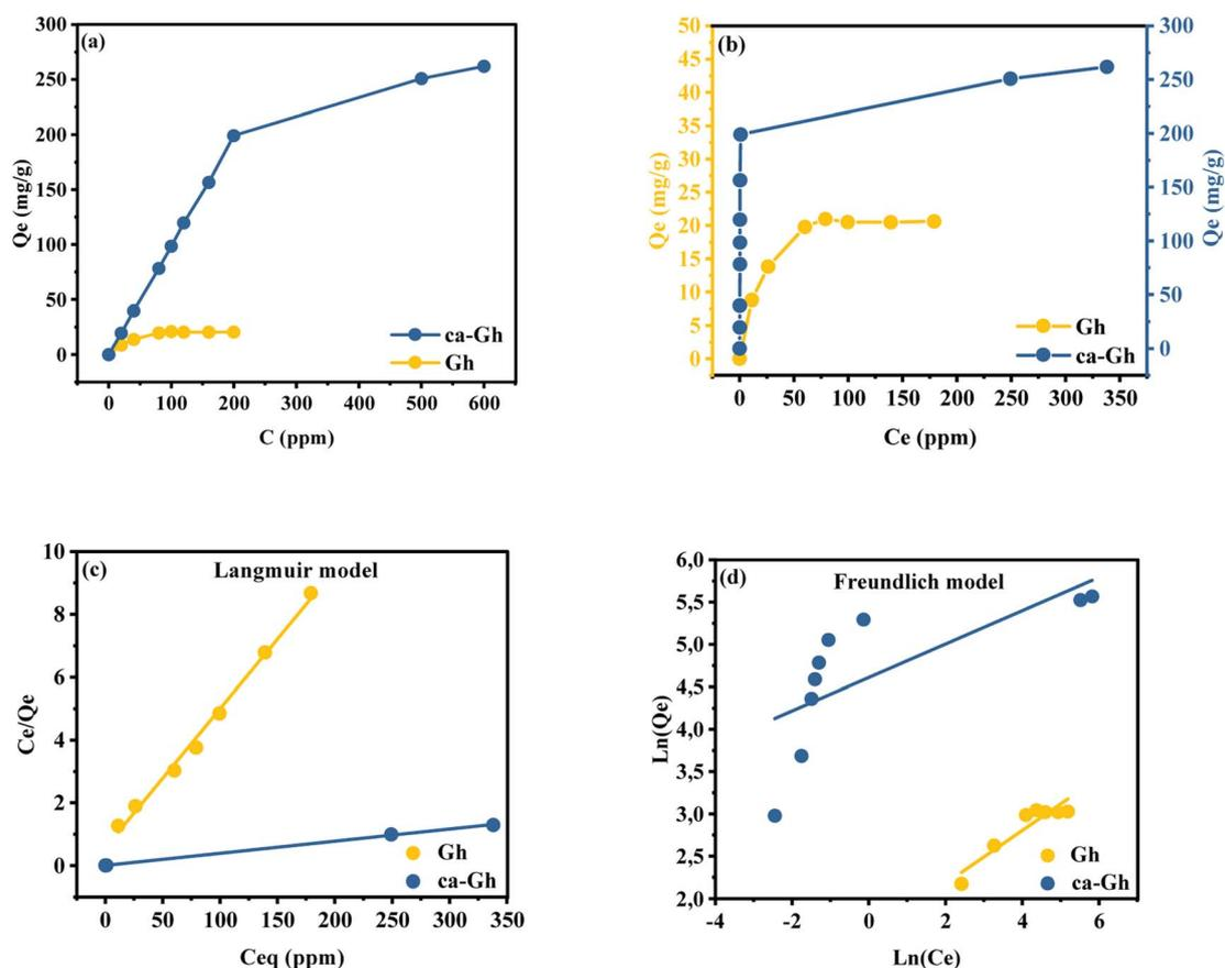
**Fig. 8** (a) Experimental equilibrium, (b) isotherm, (c) linear fitting data to Langmuir and (d) Freundlich isotherm equation of Cd<sup>2+</sup> adsorption of by Gh and ca-Gh.
