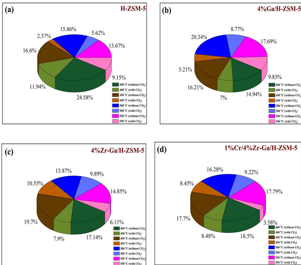
Fig. 8 Deactivation factor of the bare and metal-doped H-ZSM-5 zeolites at (a) 400 °C, (b) 450 °C, (c) 500 °C, and (d) 550 °C. Reaction conditions: pressure, 1 bar; feed gas, C<sub>3</sub>H<sub>8</sub>/N<sub>2</sub> = 2.5/97.5 and C<sub>3</sub>H<sub>8</sub>/CO<sub>2</sub>/N<sub>2</sub> = 2.5/5/92.5; flow rate, 75 mL min<sup>-1</sup>; WHSV, 4 kg<sub>cat</sub> s mol<sub>C<sub>3</sub>H<sub>8</sub></sub><sup>-1</sup>.
