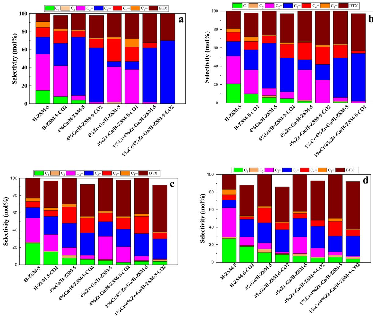
Fig. 7 Product distribution of bare and metal-doped H-ZSM-5 zeolites at (a) 400 °C, (b) 450 °C, (c) 500 °C, and (d) 550 °C. Reaction conditions: pressure, 1 bar; feed gas,  $C_3H_8/N_2 = 2.5/97.5$  and  $C_3H_8/CO_2/N_2 = 2.5/5/92.5$ ; flow rate,  $75 \text{ mL min}^{-1}$ ; WHSV,  $4 \text{ kg}_{\text{cat}} \text{ s mol}_{C_3H_8}^{-1}$ .
