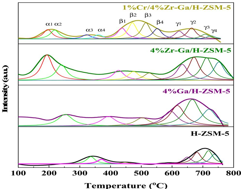
Fig. 3 H<sub>2</sub>-TPR profiles with peak fitting of the bare and Ga-, Zr-Ga-, and Cr/Zr-Ga-doped H-ZSM-5.
