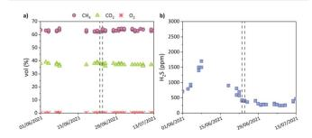
Fig. 7 Concentration of (a)  $CH_4$ ,  $CO_2$  and  $O_2$  and (b)  $H_2S$ , in the biogas produced in the sludge digester at the WWTP. The vertical dotted lines indicate the addition of purified SPA as iron source for hydrogen sulfide suppression.
