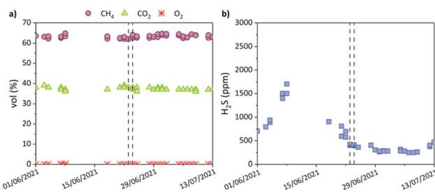
Fig. 7 Concentration of (a)  $\text{CH}_4$ ,  $\text{CO}_2$  and  $\text{O}_2$  and (b)  $\text{H}_2\text{S}$ , in the biogas produced in the sludge digester at the WWTP. The vertical dotted lines indicate the addition of purified SPA as iron source for hydrogen sulfide suppression.
