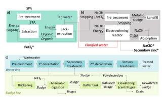
Fig. 1 Pilot plant with two integrated stages of (a) non-dispersive solvent extraction, and (b) electrowinning (\*recovered products); (c) simplified diagram of a WWTP that includes sludge treatment.
