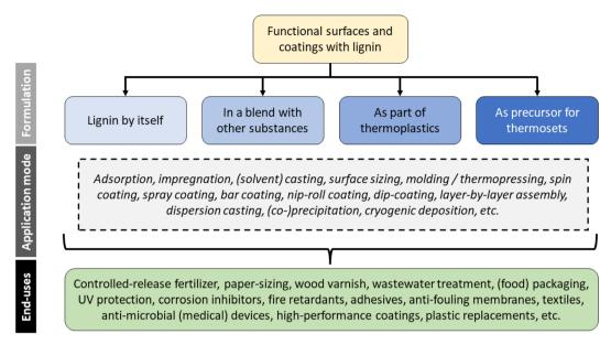
Fig. 7 Overview of different application modes for producing functional surfaces and coatings with lignin.
