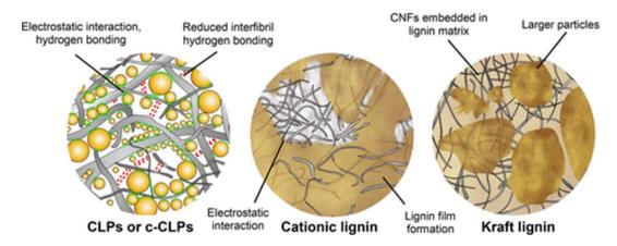
Fig. 10 Schematic illustration of proposed interaction between CNF and different lignin morphologies. $^{107}$
