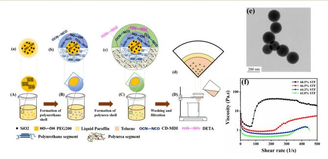
Fig. 1 Schematic illustration of the preparation of STF microcapsules with a PU/PUA double-walled shell by interfacial polymerization. (a) STF droplets dispersed in liquid paraffin; (b) STF microcapsules coated with polyurethane monolayer; (c) STF microcapsules coated with polyurethane polyurea double layer; (d) washing and filtration process; (e) TEM image of silica microspheres contained in STF; (f) variation of shear thickening with shear rate in different silica concentrations of STF.
