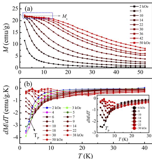
Fig. 3 (a)  $M(T)$  and (b)  $dM(T)/dT$  data of  $\text{LiSm}(\text{PO}_3)_4$  in different applied fields of  $H = 2$ – $50$  kOe. The inset plots an enlarged view of the  $dM(T)/dT$  data for  $H = 6$ – $30$  kOe showing the minima at  $T_p$ .
