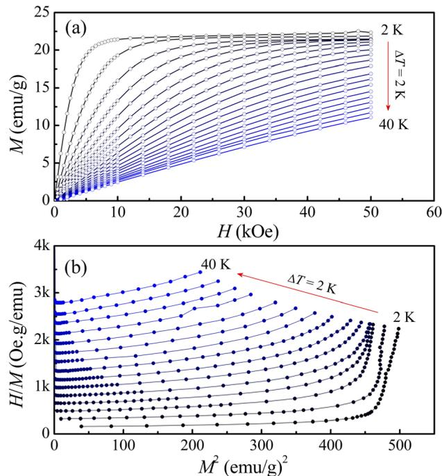
Fig. 6 (a) Representative  $M(H)$  and (b)  $M^2(H/M)$  data of  $\text{LiSm}(\text{PO}_3)_4$  at temperatures  $T = 2$ – $40$  K, where temperature increments are maintained at  $2$  K.
