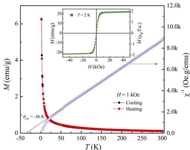
Fig. 2  $M(T)$  and  $\chi^{-1}(T)$  curves of  $\text{LiSm}(\text{PO}_3)_4$  in the field  $H = 1$  kOe, and the straight line is plotted according to the CW law. The inset is an  $M(H)$  loop recorded at  $T = 2$  K.
