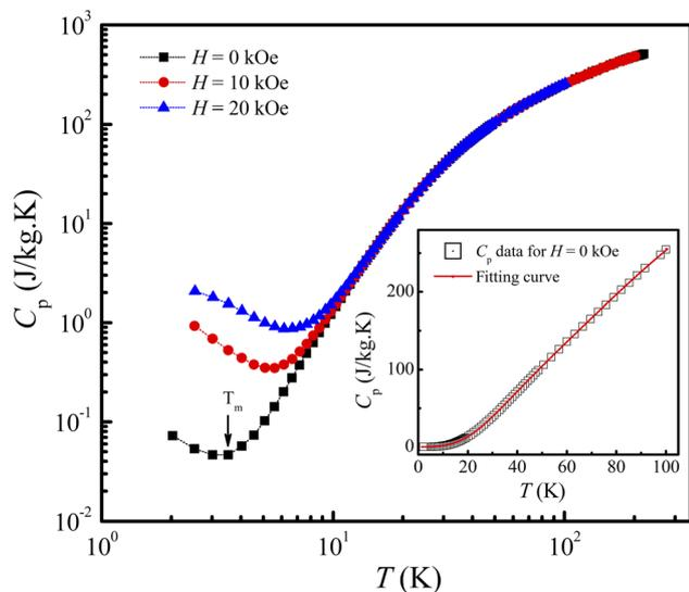
Fig. 5  $C_p(T)$  data of  $\text{LiSm}(\text{PO}_3)_4$  in the log–log scale for  $H = 0, 10,$  and  $20$  kOe. The insets plots  $C_p(T)$  data for  $H = 0$  fitted to a combination of Debye–Einstein functions, eqn (1).
