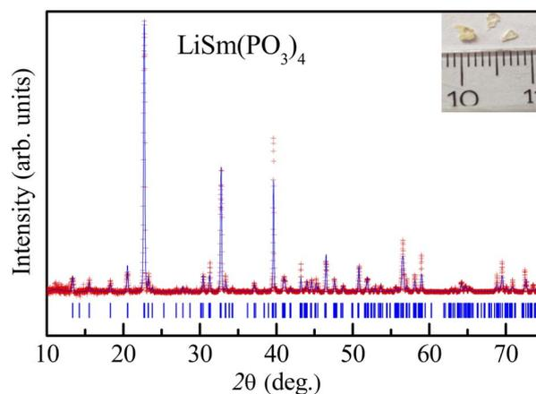
Fig. 1 Room-temperature XRD pattern of LiSm(PO<sub>3</sub>)<sub>4</sub>. Experimental data (red symbols) and calculated profile (blue lines) are shown. Vertical blue ticks denote the nuclear reflections of the monoclinic  $C2/c$  phase. The inset shows an image of LiSm(PO<sub>3</sub>)<sub>4</sub> single crystals studied in this work.
