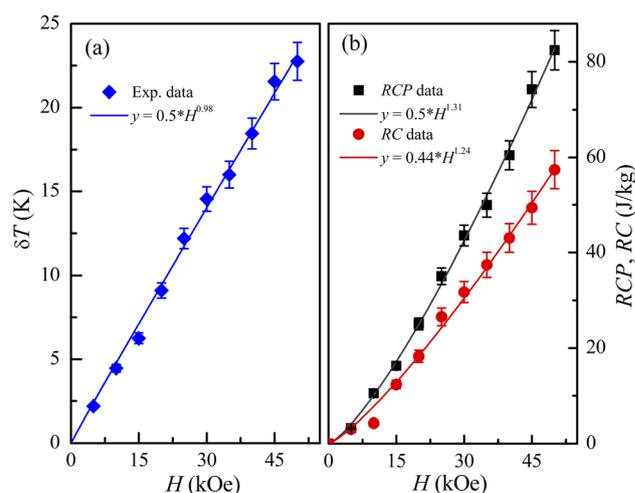
Fig. 10 (a)  $\delta T(H)$  and (b) RCP( $H$ ) and RC( $H$ ) data of  $\text{LiSm}(\text{PO}_3)_4$  for  $H = 0$ –50 kOe fitted to a power law of  $y = b \times H^m$ , with the values of  $b$  and  $m$  labeled in the figures.
