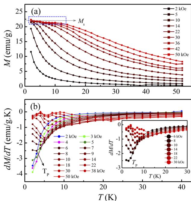
Fig. 3 (a)  $M(T)$  and (b)  $dM(T)/dT$  data of  $\text{LiSm}(\text{PO}_3)_4$  in different applied fields of  $H = 2\text{--}50$  kOe. The inset plots an enlarged view of the  $dM(T)/dT$  data for  $H = 6\text{--}30$  kOe showing the minima at  $T_p$ .
