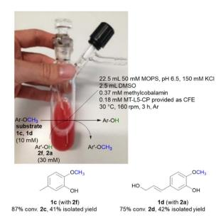
Scheme 3 Semi-preparative demethylation of  ${\bf 1c}$  and  ${\bf 1d}$  catalyzed by MT-L5-CP using Schlenk technique.
