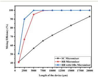
Fig. 23 Mixing efficiency across the micromixer devices at 5  $\mu$ L min<sup>-1</sup> with a diffusion co-efficient of 15.3  $\times$  10<sup>-10</sup> m<sup>2</sup> s<sup>-1</sup>.
