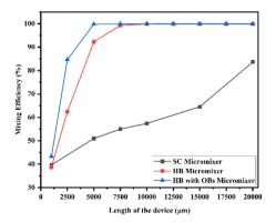
Fig. 27 Mixing efficiency across the micromixer devices at 10  $\mu$ L min<sup>-1</sup> with a diffusion co-efficient of 15.3  $\times$  10<sup>-11</sup> m<sup>2</sup> s<sup>-1</sup>.
