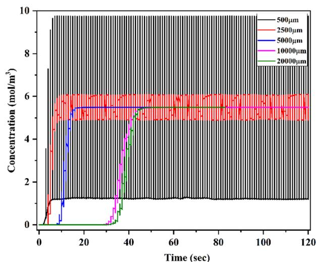
Fig. 33 Time domain study of Y-shaped herringbone serpentine channel micromixer with obstacles at  $1 \mu\text{L min}^{-1}$  with a diffusion co-efficient of  $15.3 \times 10^{-10} \text{ m}^2 \text{ s}^{-1}$ .
