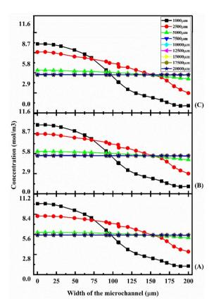
Fig. 15 Concentration across the Y-shaped herringbone serpentine channel micromixer at 1  $\mu$ L min<sup>-1</sup> (A), 5  $\mu$ L min<sup>-1</sup> (B), and 10  $\mu$ L min<sup>-1</sup> (C) with a diffusion co-efficient of 15.3  $\times$  10<sup>-11</sup> m<sup>2</sup> s<sup>-1</sup>
