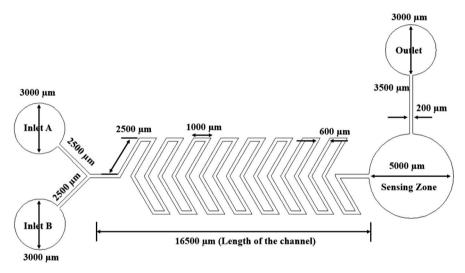
Fig. 2 Y-shaped herringbone serpentine channel micromixer.
