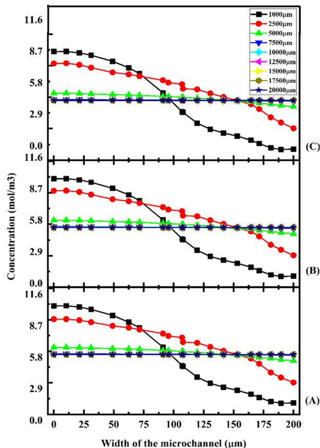
Fig. 16 Concentration across the Y-shaped herringbone serpentine channel micromixer at  $1 \mu\text{L min}^{-1}$  (A),  $5 \mu\text{L min}^{-1}$  (B), and  $10 \mu\text{L min}^{-1}$  (C) with a diffusion co-efficient of  $15.3 \times 10^{-12} \text{ m}^2 \text{ s}^{-1}$ .
