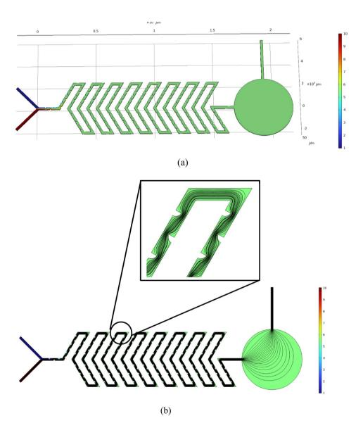
Fig. 6 Simulated result of Y-shaped herringbone serpentine channel micromixer with obstacles: (a) concentration field and (b) streamline distribution at  $5000 \mu m$ .
