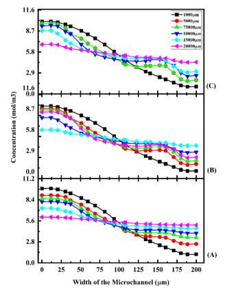
Fig. 12 Concentration across the Y-shaped straight channel micromixer at 1  $\mu$ L min<sup>-1</sup> (A), 5  $\mu$ L min<sup>-1</sup> (B), and 10  $\mu$ L min<sup>-1</sup> (C) with a diffusion co-efficient of  $15.3 \times 10^{-11}$  m<sup>2</sup> s<sup>-1</sup>
