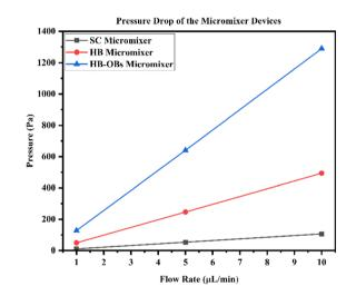
Fig. 29 Pressure drops vs. flow rates in the micromixer devices.
