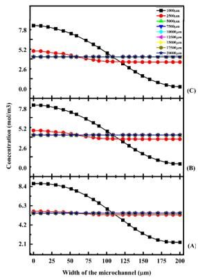
Fig. 19 Concentration across the Y-shaped herringbone serpentine channel micromixer with obstacles at  $1 \,\mu\text{L min}^{-1}$  (A),  $5 \,\mu\text{L min}^{-1}$  (B), and 10  $\mu L$  min<sup>-1</sup> (C) with a diffusion co-efficient of 15.3  $\times$  10<sup>-12</sup> m<sup>2</sup> s<sup>-1</sup>
