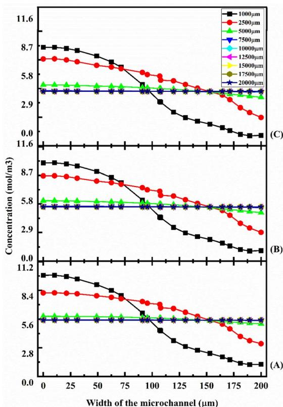
Fig. 15 Concentration across the Y-shaped herringbone serpentine channel micromixer at  $1 \mu\text{L min}^{-1}$  (A),  $5 \mu\text{L min}^{-1}$  (B), and  $10 \mu\text{L min}^{-1}$  (C) with a diffusion co-efficient of  $15.3 \times 10^{-11} \text{ m}^2 \text{ s}^{-1}$ .
