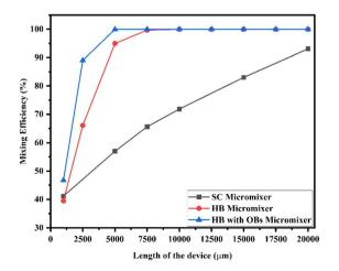
Fig. 22 Mixing efficiency across the micromixer devices at  $1 \mu L min^{-1}$ with a diffusion co-efficient of  $15.3 \times 10^{-12}$  m<sup>2</sup> s<sup>-1</sup>.
