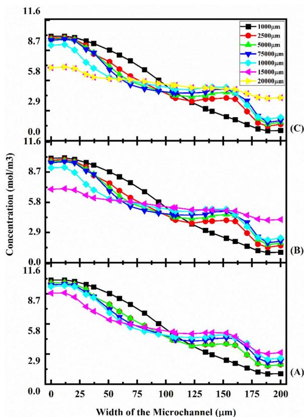
Fig. 13 Concentration across the Y-shaped straight channel micromixer at  $1 \mu\text{L min}^{-1}$  (A),  $5 \mu\text{L min}^{-1}$  (B), and  $10 \mu\text{L min}^{-1}$  (C) with a diffusion coefficient of  $15.3 \times 10^{-12} \text{ m}^2 \text{ s}^{-1}$ .
