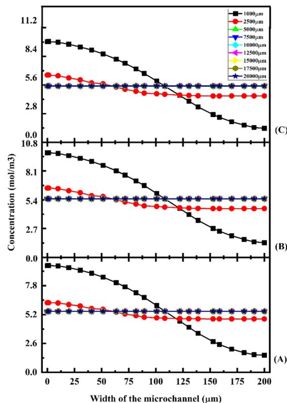
Fig. 18 Concentration across the Y-shaped herringbone serpentine channel micromixer with obstacles at  $1 \mu\text{L min}^{-1}$  (A),  $5 \mu\text{L min}^{-1}$  (B), and  $10 \mu\text{L min}^{-1}$  (C) with a diffusion co-efficient of  $15.3 \times 10^{-11} \text{ m}^2 \text{ s}^{-1}$ .
