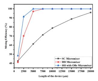
Fig. 21 Mixing efficiency across the micromixer devices at  $1 \mu L min^{-1}$ with a diffusion co-efficient of  $15.3 \times 10^{-11} \, \text{m}^2 \, \text{s}^{-1}$ .
