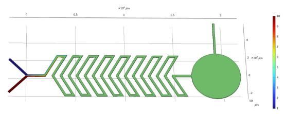
Fig. 5 Simulated result of Y-shaped herringbone serpentine channel micromixer.
