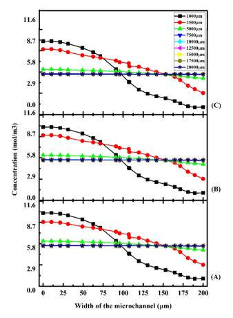
Fig. 16 Concentration across the Y-shaped herringbone serpentine channel micromixer at 1  $\mu$ L min<sup>-1</sup> (A), 5  $\mu$ L min<sup>-1</sup> (B), and 10  $\mu$ L min<sup>-1</sup> (C) with a diffusion co-efficient of 15.3  $\times$  10  $^{-12}$  m $^2$  s $^{-1}$
