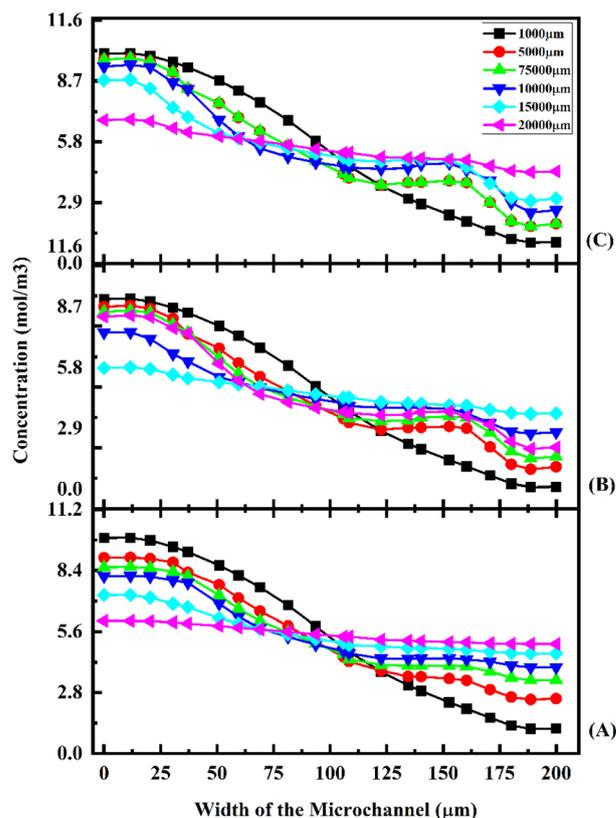
Fig. 12 Concentration across the Y-shaped straight channel micromixer at  $1 \mu\text{L min}^{-1}$  (A),  $5 \mu\text{L min}^{-1}$  (B), and  $10 \mu\text{L min}^{-1}$  (C) with a diffusion co-efficient of  $15.3 \times 10^{-11} \text{ m}^2 \text{ s}^{-1}$ .
