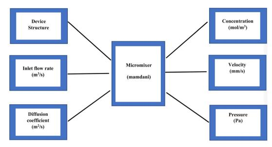
Fig. 7 Fuzzy logic model of the micromixer.
