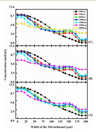
Fig. 13 Concentration across the Y-shaped straight channel micromixer at 1  $\mu$ L min<sup>-1</sup> (A), 5  $\mu$ L min<sup>-1</sup> (B), and 10  $\mu$ L min<sup>-1</sup> (C) with a diffusion co-efficient of 15.3  $\times$  10<sup>-12</sup> m<sup>2</sup> s<sup>-1</sup>.
