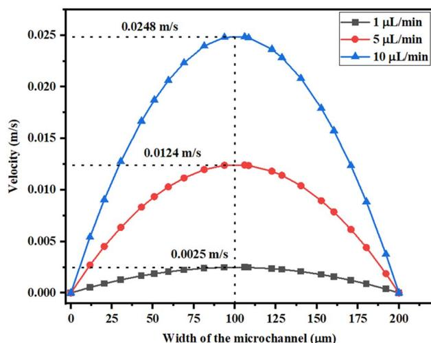
Fig. 8 Velocity across the Y-shaped straight channel micromixer.
