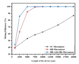
Fig. 24 Mixing efficiency across the micromixer devices at 5  $\mu$ L min<sup>-1</sup> with a diffusion co-efficient of 15.3  $\times$  10<sup>-11</sup> m<sup>2</sup> s<sup>-1</sup>.
