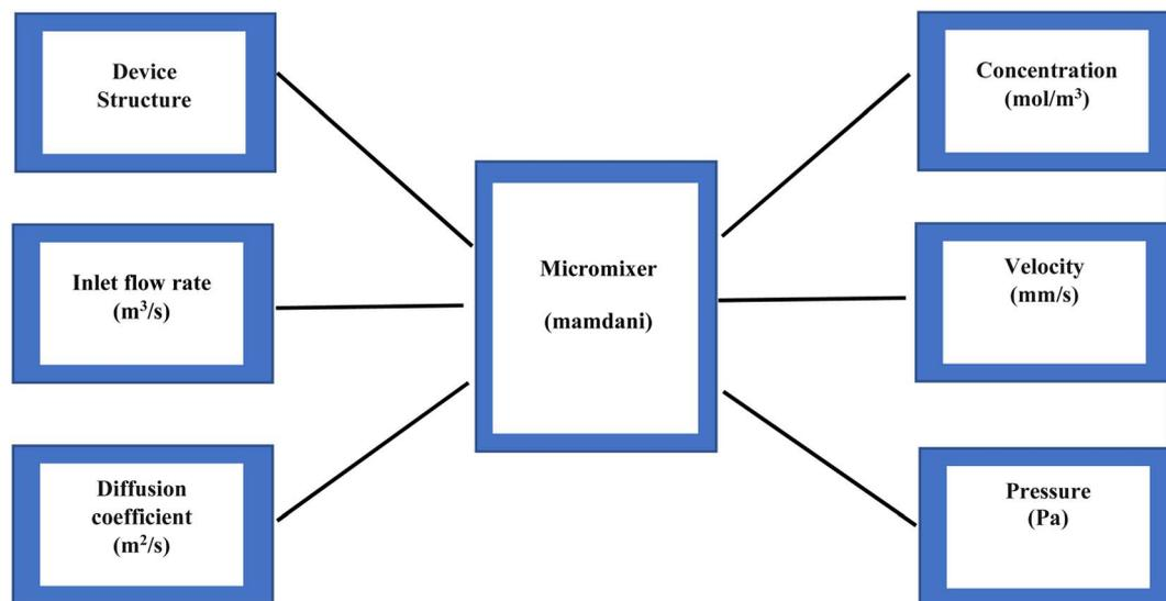
Fig. 7 Fuzzy logic model of the micromixer.
