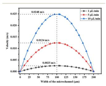
Fig. 8 Velocity across the Y-shaped straight channel micromixer.
