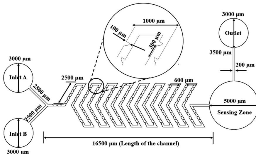
Fig. 3 Y-shaped herringbone serpentine channel micromixer with obstacles.
