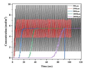
Fig. 32 Time domain study of Y-shaped herringbone serpentine channel micromixer at 1  $\mu$ L min<sup>-1</sup> with a diffusion co-efficient of 15.3  $\times$  10<sup>-10</sup> m<sup>2</sup> s<sup>-1</sup>.
