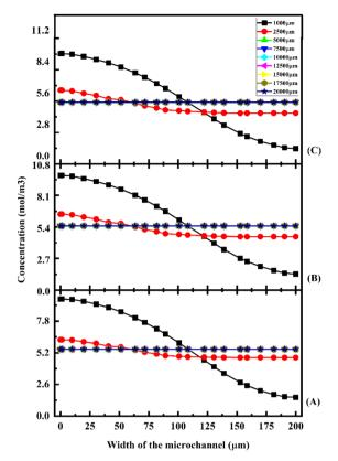
Fig. 18 Concentration across the Y-shaped herringbone serpentine channel micromixer with obstacles at  $1\,\mu\text{L}\,\text{min}^{-1}$  (A),  $5\,\mu\text{L}\,\text{min}^{-1}$  (B), and  $10\,\mu\text{L}\,\text{min}^{-1}$  (C) with a diffusion co-efficient of  $15.3\times10^{-11}\,\text{m}^2\,\text{s}^{-1}$ .
