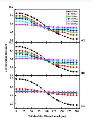
Fig. 11 Concentration across the Y-shaped straight channel micromixer at 1  $\mu$ L min<sup>-1</sup> (A), 5  $\mu$ L min<sup>-1</sup> (B), and 10  $\mu$ L min<sup>-1</sup> (C) with a diffusion co-efficient of  $15.3 \times 10^{-10} \text{ m}^2 \text{ s}^{-1}$
