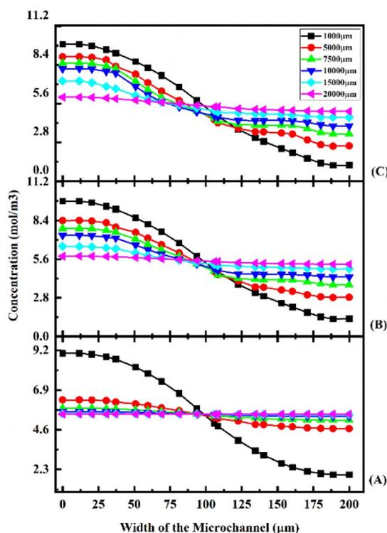
Fig. 11 Concentration across the Y-shaped straight channel micromixer at  $1 \mu\text{L min}^{-1}$  (A),  $5 \mu\text{L min}^{-1}$  (B), and  $10 \mu\text{L min}^{-1}$  (C) with a diffusion co-efficient of  $15.3 \times 10^{-10} \text{ m}^2 \text{ s}^{-1}$ .
