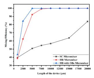
Fig. 28 Mixing efficiency across the micromixer devices at 10  $\mu$ L min<sup>-1</sup> with a diffusion co-efficient of 15.3  $\times$  10<sup>-12</sup> m<sup>2</sup> s<sup>-1</sup>.
