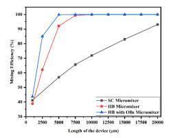
Fig. 26 Mixing efficiency across the micromixer devices at 10  $\mu$ L min<sup>-1</sup> with a diffusion co-efficient of 15.3  $\times$  10<sup>-10</sup> m<sup>2</sup> s<sup>-1</sup>.
