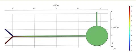
Fig. 4 Simulated result of Y-shaped straight channel micromixer.
