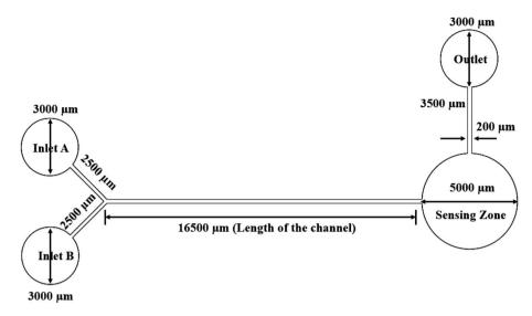
Fig. 1 Y-shaped straight channel micromixer.
