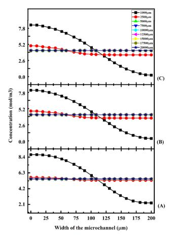
Fig. 17 Concentration across the Y-shaped herringbone serpentine channel micromixer with obstacles at  $1\,\mu\text{L}\,\text{min}^{-1}$  (A),  $5\,\mu\text{L}\,\text{min}^{-1}$  (B), and 10  $\mu\text{L}\,\text{min}^{-1}$  (C) with a diffusion co-efficient of 15.3  $\times$  10 $^{-10}$  m² s $^{-1}$ .
