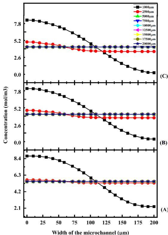
Fig. 19 Concentration across the Y-shaped herringbone serpentine channel micromixer with obstacles at  $1 \mu\text{L min}^{-1}$  (A),  $5 \mu\text{L min}^{-1}$  (B), and  $10 \mu\text{L min}^{-1}$  (C) with a diffusion co-efficient of  $15.3 \times 10^{-12} \text{ m}^2 \text{ s}^{-1}$ .
