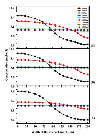
Fig. 14 Concentration across the Y-shaped herringbone serpentine channel micromixer at 1  $\mu L$  min $^{-1}$  (A), 5  $\mu L$  min $^{-1}$  (B), and 10  $\mu L$  min $^{-1}$  (C) with a diffusion co-efficient of 15.3  $\times$  10 $^{-10}$  m $^2$  s $^{-1}$ .
