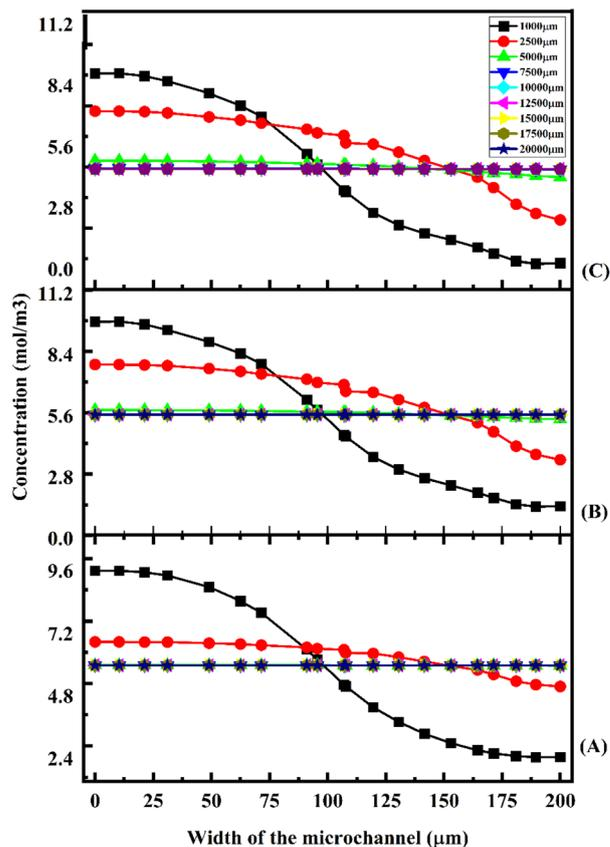
Fig. 14 Concentration across the Y-shaped herringbone serpentine channel micromixer at  $1 \mu\text{L min}^{-1}$  (A),  $5 \mu\text{L min}^{-1}$  (B), and  $10 \mu\text{L min}^{-1}$  (C) with a diffusion coefficient of  $15.3 \times 10^{-10} \text{ m}^2 \text{ s}^{-1}$ .
