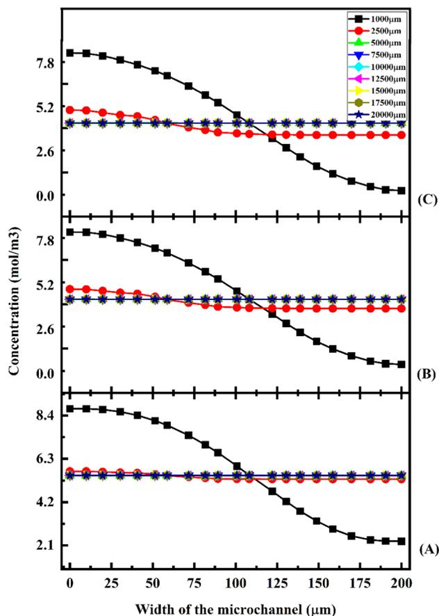
Fig. 17 Concentration across the Y-shaped herringbone serpentine channel micromixer with obstacles at  $1 \mu\text{L min}^{-1}$  (A),  $5 \mu\text{L min}^{-1}$  (B), and  $10 \mu\text{L min}^{-1}$  (C) with a diffusion co-efficient of  $15.3 \times 10^{-10} \text{ m}^2 \text{ s}^{-1}$ .
