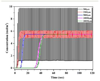
Fig. 33 Time domain study of Y-shaped herringbone serpentine channel micromixer with obstacles at 1  $\mu$ L min<sup>-1</sup> with a diffusion coefficient of 15.3  $\times$  10<sup>-10</sup> m<sup>2</sup> s<sup>-1</sup>.
