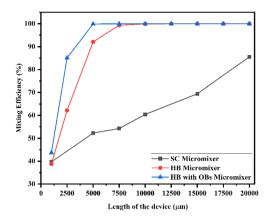
Fig. 25 Mixing efficiency across the micromixer devices at 5  $\mu$ L min<sup>-1</sup> with a diffusion co-efficient of 15.3  $\times$  10<sup>-12</sup> m<sup>2</sup> s<sup>-1</sup>.
