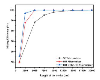
Fig. 20 Mixing efficiency across the micromixer devices at 1  $\mu$ L min<sup>-1</sup> with a diffusion co-efficient of 15.3  $\times\,10^{-10}~\text{m}^2~\text{s}^{-1}$
