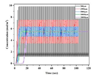
Fig. 31 Time domain study of Y-shaped straight channel micromixer at 1  $\mu L$   $min^{-1}$  with a diffusion co-efficient of 15.3  $\times$   $10^{-10}~m^2~s^{-1}$
