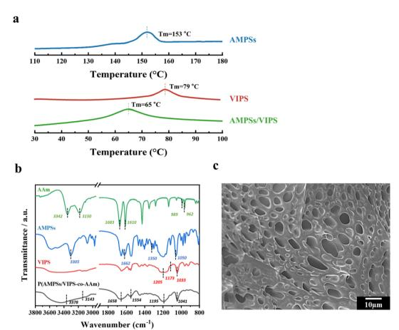
Fig. 2 (a) DSC curves of AMPSs, VIPS, and AMPSs/VIPS pair. (b) FTIR spectra of AAm, AMPSs, VIPS, and the P(AMPSs/VIPS-co-AAm) hydrogel. (c) SEM images showing the porous structure of the P(AMPSs/VIPS-co-AAm) hydrogel.
