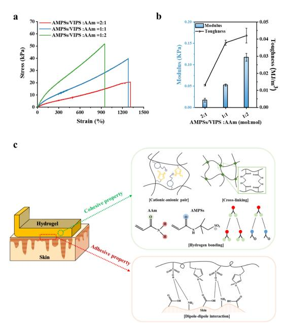
Fig. 3 (a) Tensile curves of the P(AMPSs/VIPS-co-AAm) hydrogel with different mole ratios of AAm and (b) the corresponding Young's modulus and toughness. (c) A representative mechanism associated with increased internal cohesive and interfacial adhesive properties
