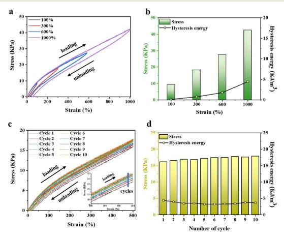
Fig. 5 (a)Tensile cyclic test of the P(AMPSs/VIPS-co-AAm) hydrogel with increasing strain (100%, 300%, 600%, 1000%) and (b) corresponding stress and hysteresis energy. (c) Ten successive tensile loading cycles at 500% strain without resting time. (d) The corresponding stress and hysteresis energy.
