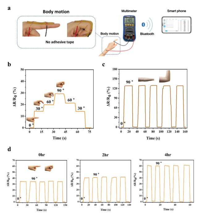
Fig. 7 (a) Real-time resistance-variation measurement using Bluetooth electronic devices. The real-time sensing of the P(AMPSs/VIPS-co-AAm) hydrogel in detecting human body motions: (b) finger bending at various angles (0° to 30°, 60°, and 90°) and (c) elbow bending (0° and 90°). (d) The relative resistance change upon repeated finger bending (0° and 90°) as a function of dehydration time.
