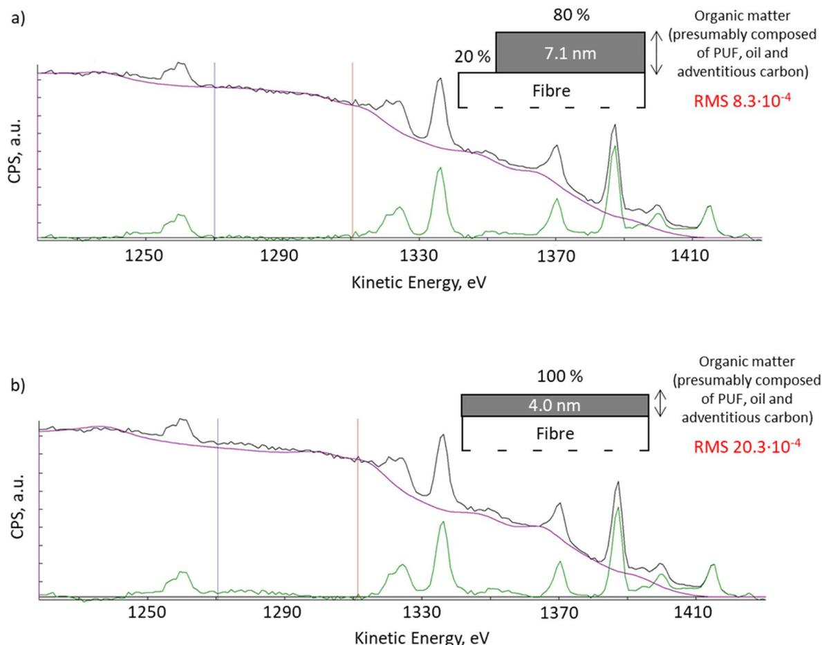
Fig. 2 XPS spectra QUASES fitting using model: (a) with 80% of the surface covered with 7.1 nm organic layer and 20% of the uncoated surface; (b) uniform organic layer of 4.0 nm thick (Okhrimenko *et al.*, 2018).<sup>20</sup>
