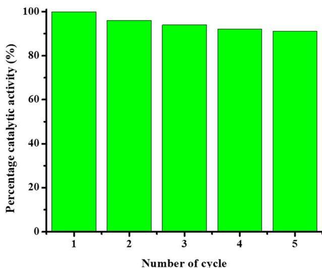
Fig. 13 The catalytic activity percentage of Ag/Ni-P(NMA-MAA) system used for catalytic degradation of MOR [conditions: Ag/Ni-P(NMA-MAA) = 85.71  $\mu\text{g mL}^{-1}$ , concentration of MOR = 0.080 mM, NaBH<sub>4</sub> = 9.65 mM].
