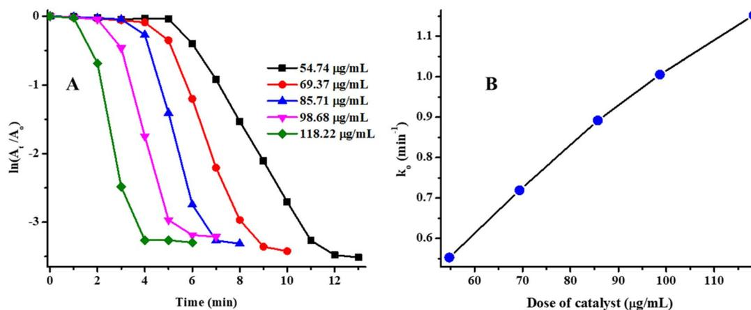
Fig. 9 Degradation of MOR dye (A) time vs.  $\ln(A_t/A_0)$  plot under various concentrations of Ag/Ni-P(NMA-MAa) [conditions:  $\text{NaBH}_4 = 9.65 \text{ mM}$ , pH = 5.56, concentration of MeOr = 0.080 mM, Ag/Ni-P(NMA-MAa) = (54.74–118.22)  $\mu\text{g mL}^{-1}$ ] and (B) catalytic dose vs.  $k_0$  at 26 °C.
