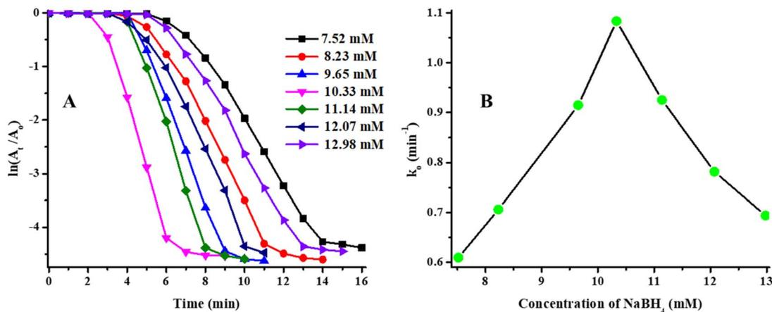
Fig. 11 Effect of concentration of  $\text{NaBH}_4$  on catalytic degradation of MOR at 26 °C (A)  $\ln(A_t/A_0)$  vs.  $T$  function for degradation of MOR (0.080 mM) in the presence of  $\text{NaBH}_4$  (7.52–12.98 mM) and Ag/Ni-P(NMA-MAA) ( $85.71 \mu\text{g mL}^{-1}$ ), (B) the  $k_0$  vs.  $\text{NaBH}_4$  concentration dependent graph.
