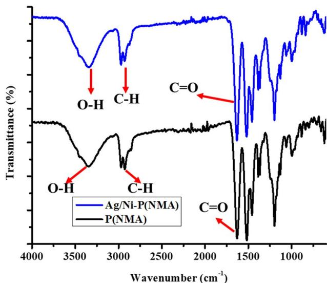
Fig. 2 FTIR spectra of synthesized P(NMA-MAA) and Ag/Ni-P(NMA-MAA).
