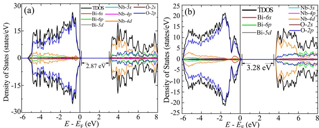
Fig. 10 TDOS and its projection onto different orbitals in Bi, Nb, and O for (a)  $\alpha$ -BNO ( $\alpha_{\text{HF}} = 2\%$ ) and (b)  $\beta$ -BNO ( $\alpha_{\text{HF}} = 20\%$ ) using HSE06 functional.
