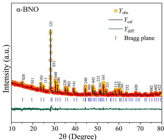
Fig. 1 Rietveld refined XRD patterns on top of experimentally observed data for  $\alpha$ -BNO. The yellow circles are the experimental data points ( $Y_{\text{obs}}$ ), the black solid line represents the calculated refined pattern  $Y_{\text{cal}}$ , the bottom green curve  $Y_{\text{diff}}$  shows the difference between the experimental  $Y_{\text{obs}}$  and calculated  $Y_{\text{cal}}$  values.
