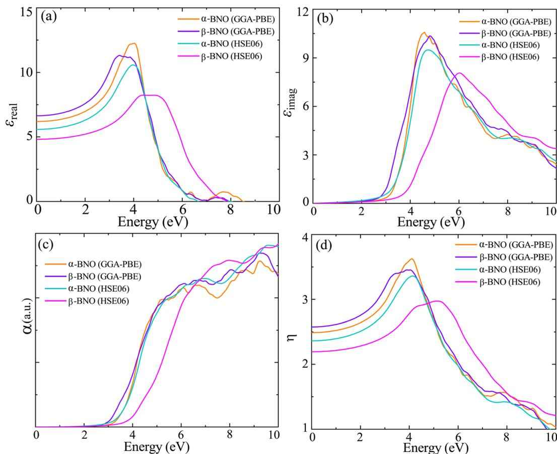
Fig. 13 Optical properties. (a) Real part of dielectric constant  $\varepsilon_{\text{real}}$ , (b) imaginary part of the dielectric constant  $\varepsilon_{\text{imag}}$ , (c) absorption coefficient  $\alpha$ , (d) refractive index  $\eta$  a function photon energy  $E$  calculated from GGA-PBE and HSE06 averaged over three different polarization  $E_x$ ,  $E_y$  and  $E_z$  in case of  $\alpha$ -BNO ( $\alpha_{\text{HF}} = 2\%$ ) and  $\beta$ -BNO ( $\alpha_{\text{HF}} = 20\%$ ) functional.
