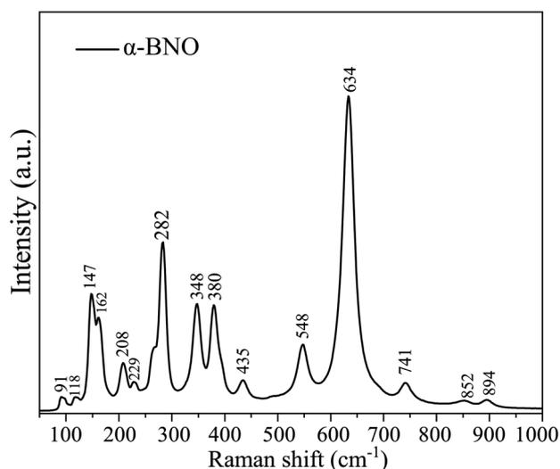
**Fig. 4** Room temperature Raman spectra of  $\alpha$ -BNO.
