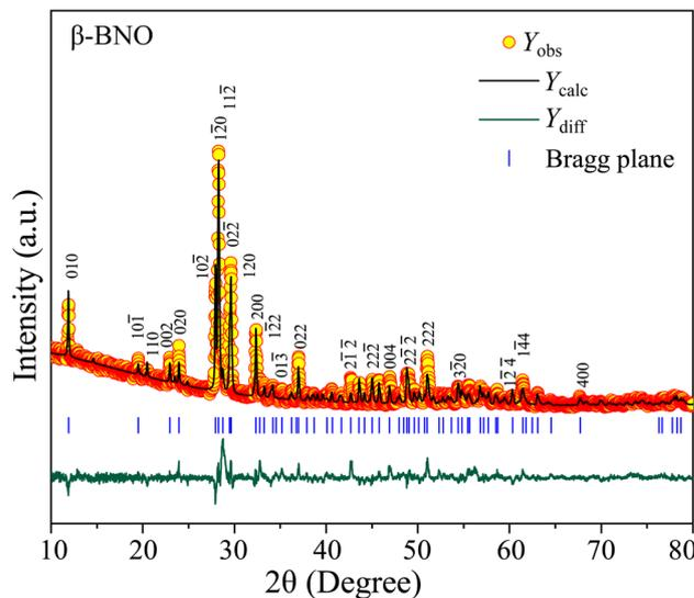
Fig. 2 Rietveld refined XRD patterns on top of experimentally observed data for  $\beta$ -BNO. The yellow circles are the experimental data points ( $Y_{\text{obs}}$ ), the black solid line represents the calculated refined pattern  $Y_{\text{cal}}$ , the bottom green curve  $Y_{\text{diff}}$  shows the difference between the experimental  $Y_{\text{obs}}$  and calculated  $Y_{\text{cal}}$  values.
