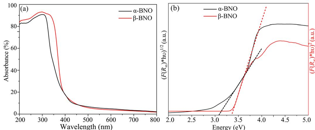
Fig. 7 (a) UV-Vis diffuse absorption spectra. (b) Band gap estimation from Tauc plots for  $\alpha$ -BNO and  $\beta$ -BNO.
