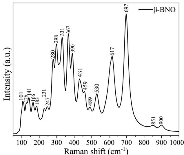
Fig. 5 Room temperature Raman spectra of  $\beta$ -BNO.Table 2 RT experimental (Exp.) and DFT (LDA norm-conserving pseudo-potential) based Raman peaks of both  $\alpha$ -BNO and  $\beta$ -BNO
