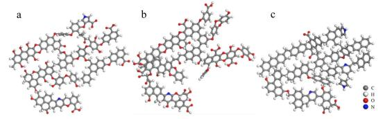
Fig. 5 Molecular structure model of coals (a) A:  $C_{174}H_{116}N_2O_{40}$ , (b) B:  $C_{161}H_{94}N_2O_{50}$ , and (c) C:  $C_{183}H_{140}N_4O_{11}$  (gray: carbon atom, white: hydrogen atom, red: oxygen atom, and blue: nitrogen atom).
