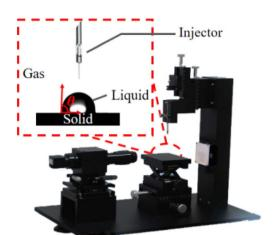
Fig. 1 Schematic diagram of contact angle measurement.
