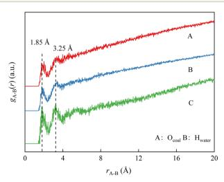
Fig. 8 RDF for oxygen atoms on the coal surface with the hydrogen atom of water.
