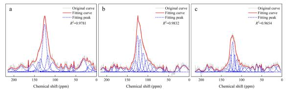
Fig. 2 Curve-fitting <sup>13</sup>C NMR spectra of Coals (a) A, (b) B, and (c) C.
