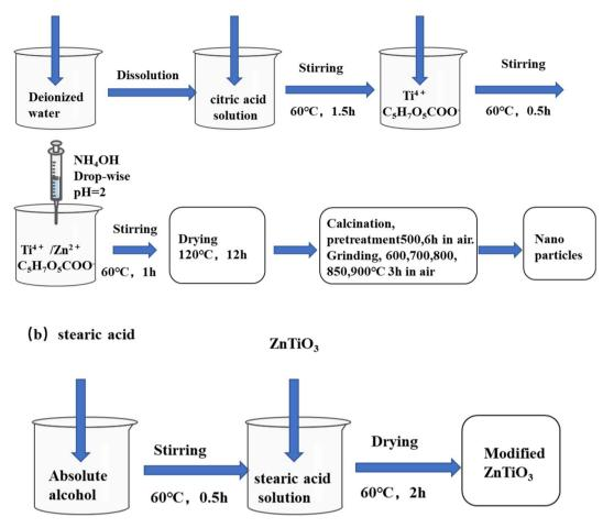
Synthesis of nano ZT (a) sol-gel synthesis, (b) hydrophobically modified by stearic acid.
