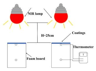
Fig. 7 Insulation test device.
