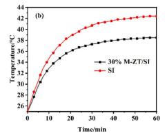
Fig. 8 The temperature (a) the inner surface of films, (b) the interior air of the foam boxes.
