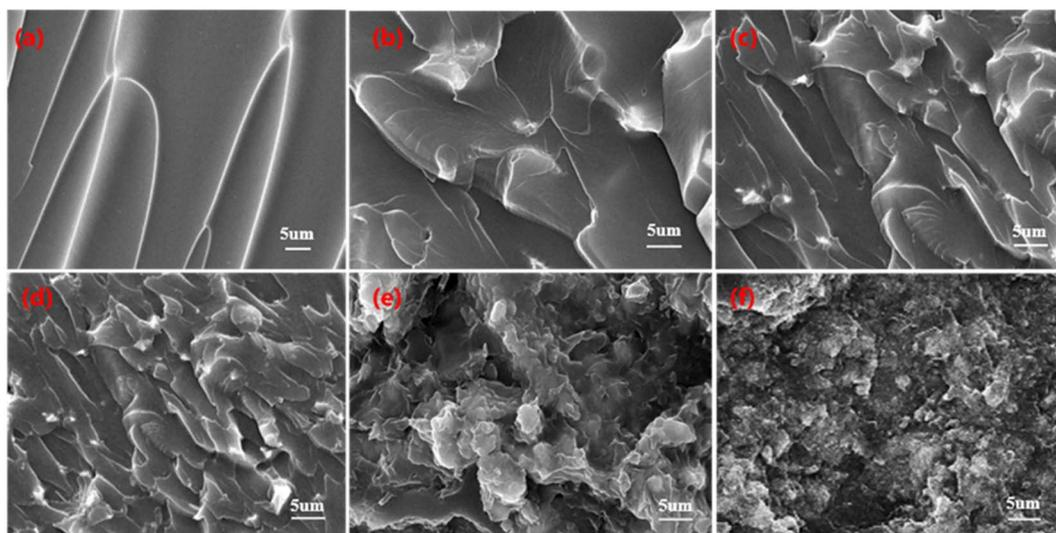
Fig. 3 SEM micrographs of fractured surfaces for SI and ZT/SI composite films. (a) SI, (b) 5 wt% M-ZT, (c) 10 wt% M-ZT, (d) 15 wt% M-ZT, (e) 30 wt% M-ZT, (f) 30 wt% ZT.
