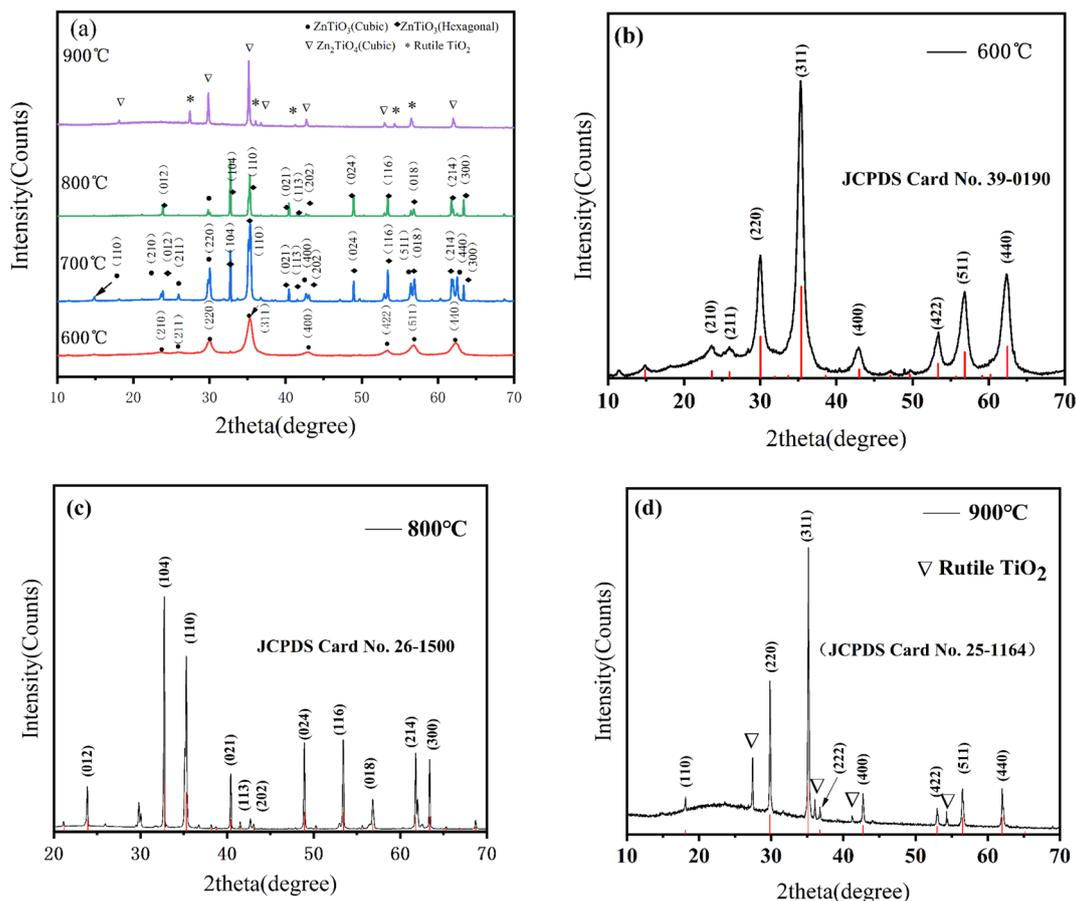
Fig. 2 XRD patterns of ZT calcined at different temperatures.
