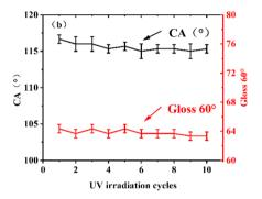
Weathering test of coatings, (a) high-low temperature cycles test, (b) UV radiation resistance.
