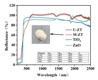
Fig. 5 Solar reflectance spectra of U-ZT, M-ZT, TiO<sub>2</sub>, and ZnO.
