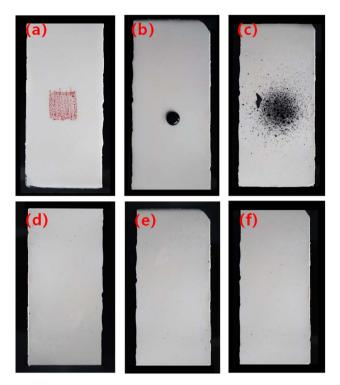
Fig. 11 Anti-graffiti tests. (a) Oily red marker, (b) water-based black ink, (c) solvent-based black acrylic spray paint; (d-f) respectively for the coating after wiping.
