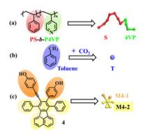
Fig. 3 Coarse-grained models of the system. (a) PS-b-P4VP; (b) CO<sub>2</sub>-toluene; and (c) 4. Color scheme: S, red; 4VP, green; solvent beads, violet; M4-1, orange; M4-2, yellow.
