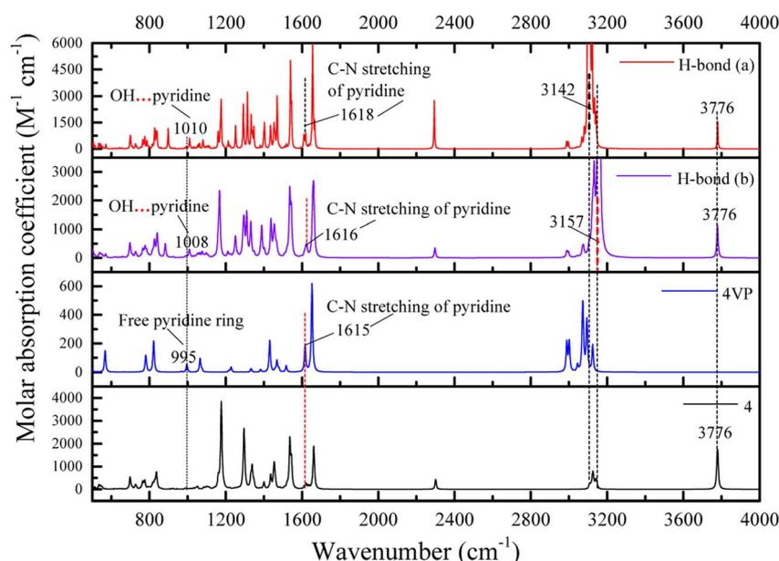
Fig. 7 DFT calculated IR spectra for the hydrogen bonding between P4VP and **4** of the SAFCs.
