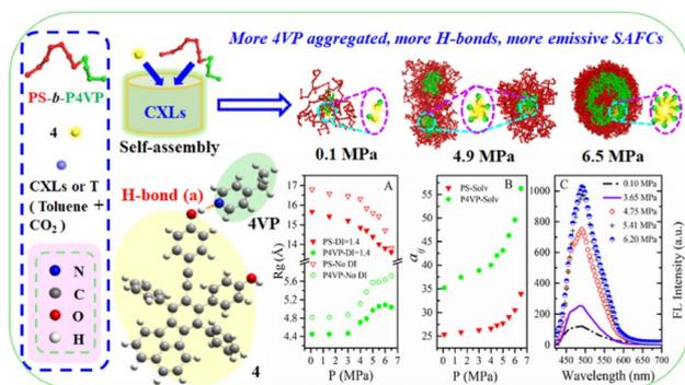
Fig. 2 The DPD simulated structural information and experimental FL data of copolymer blends PS<sub>240</sub>-*b*-P4VP<sub>40</sub>/**4** in CO<sub>2</sub>-toluene at 313.2 K and varied pressures.
