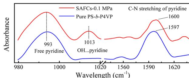
Fig. 8 The experimental IR spectra of pure PS-*b*-P4VP and the SAFCs of PS-*b*-P4VP/**4** in CO<sub>2</sub>-expanded toluene (313.2 K/0.1 MPa for 72 h).
