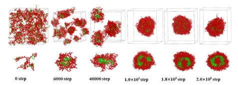
Fig. 4 Sequential snapshots of the micelle formation of copolymer blends  $PS_{240}$ -b- $P4VP_{40}$ /4 at different simulation time in  $CO_2$ -expanded toluene at 313.2 K and 6.0 MPa. Copolymer blends  $PS_{240}$ -b- $P4VP_{40}$  with DI = 1.4 (mass fraction of 75%  $PS_{240}$ -b- $P4VP_{40}$  + 10%  $PS_{360}$ -b- $P4VP_{60}$  + 15%  $PS_{120}$ -b- $P4VP_{20}$ ). The images below the box are the cross-section views. The color scheme is the same as in Fig. 3. Solvent beads are hidden.
