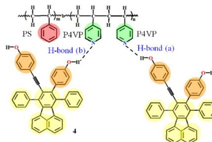
Fig. 1 Hydrogen bonding between PS-*b*-P4VP and **4** (dashed lines represent the hydrogen bonding). H-bond (a) stands for the hydrogen bonds between ethynylphenolic OH group of **4** and pyridyl nitrogen atom of P4VP segments, and H-bond (b) between phenolic OH of **4** and nitrogen atom of P4VP.
