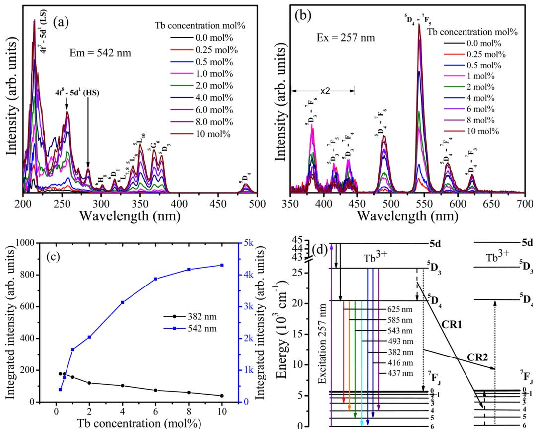
Fig. 6 PL spectra of undoped and  $\text{Tb}^{3+}$  doped  $\text{CaF}_2$  nanoparticles. (a) Excitation spectra monitored for emission at 542 nm. (b) Emission spectra excited at 257 nm. (c) Integrated intensity of the bands at 382 nm and 542 nm as a function of  $\text{Tb}^{3+}$  concentration. (d) Energy diagram representation of  $\text{Tb}^{3+}$  ions in  $\text{CaF}_2$  host as well as the cross-relaxation paths.
