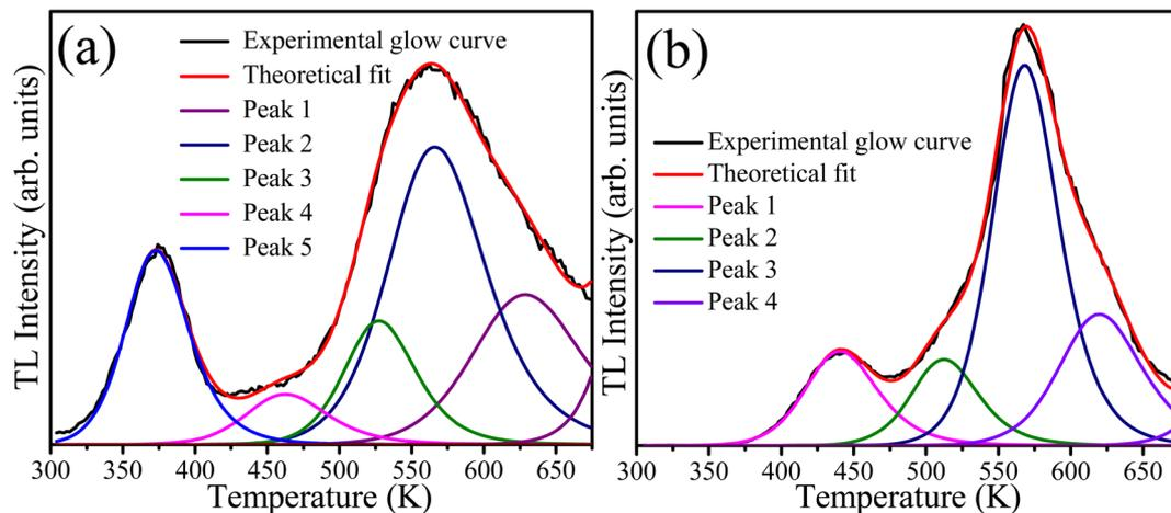
Fig. 11 Deconvoluted TL glow curves of the sample with 10 mol% of Tb ions (a) unirradiated and (b) irradiated with 254 nm UV light for 46 hours.
