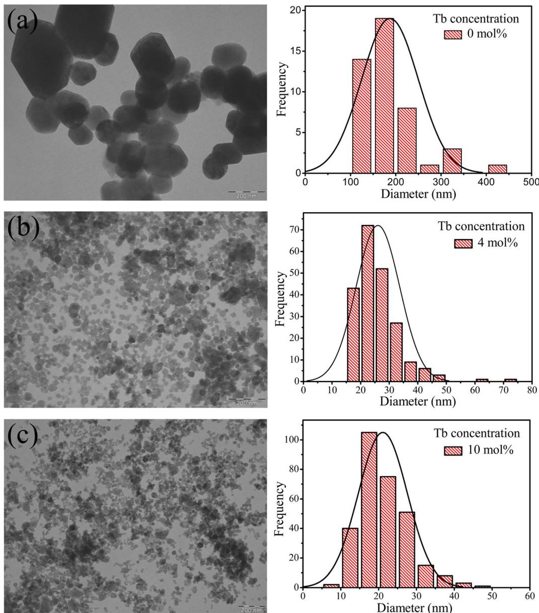
Fig. 2 TEM images of CaF<sub>2</sub> nanoparticles doped with different Tb<sup>3+</sup> contents (a) 0 mol%, (b) 4 mol% and (c) 10 mol%. Corresponding histograms represent the particles size distributions obtained from the TEM images.
