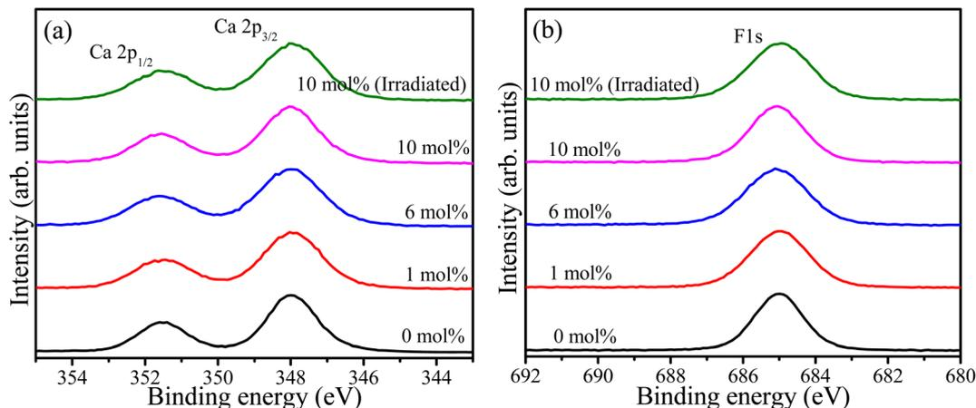
Fig. 3 XPS high resolution spectra of (a) Ca 2p and (b) F 1s of the CaF<sub>2</sub> doped with different Tb concentrations.
