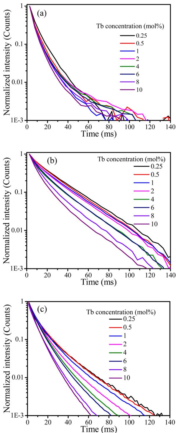
Fig. 7 Decay curves of the  $\text{CaF}_2$  doped with different concentration of Tb ions excited at 257 nm for the emission band at (a) 382 nm and (b) 542 nm, (c) excited at 486 nm for the band at 542 nm.
