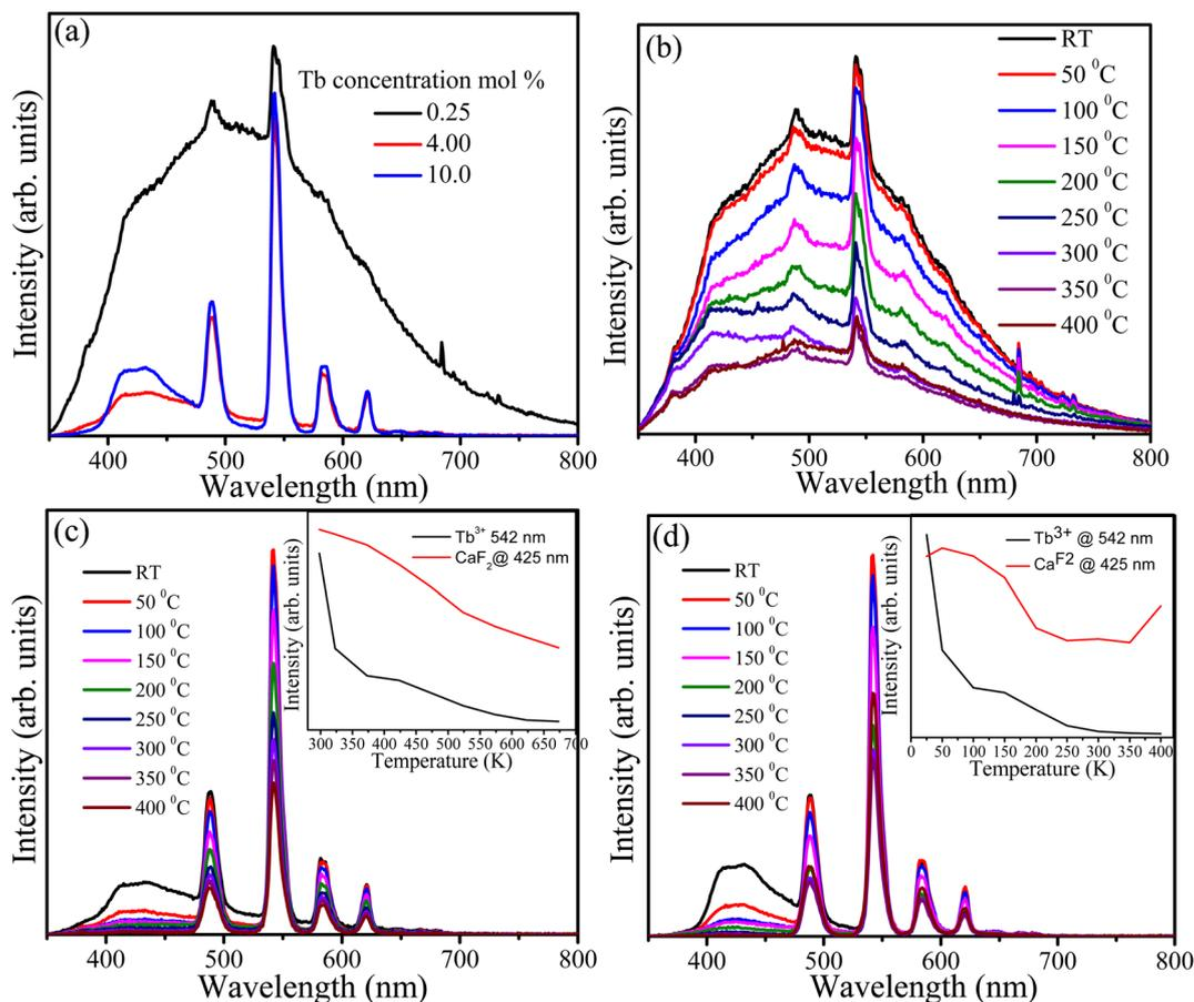
Fig. 9 PL spectra of the  $\text{CaF}_2$  doped with different Tb concentrations (a), and temperature-dependent PL of the same samples (b) 0.25 mol%, (c) 4 mol% and (d) 10 mol%, the insets are the PL integrated intensity of the 542 nm band and the broad band ranges from 400 nm to 476 nm. All samples were excited at 325 nm by using He–Cd laser.
