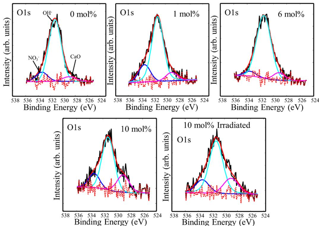
Fig. 4 XPS high resolution spectra of O 1s impurity in CaF<sub>2</sub> doped with different Tb concentrations.
