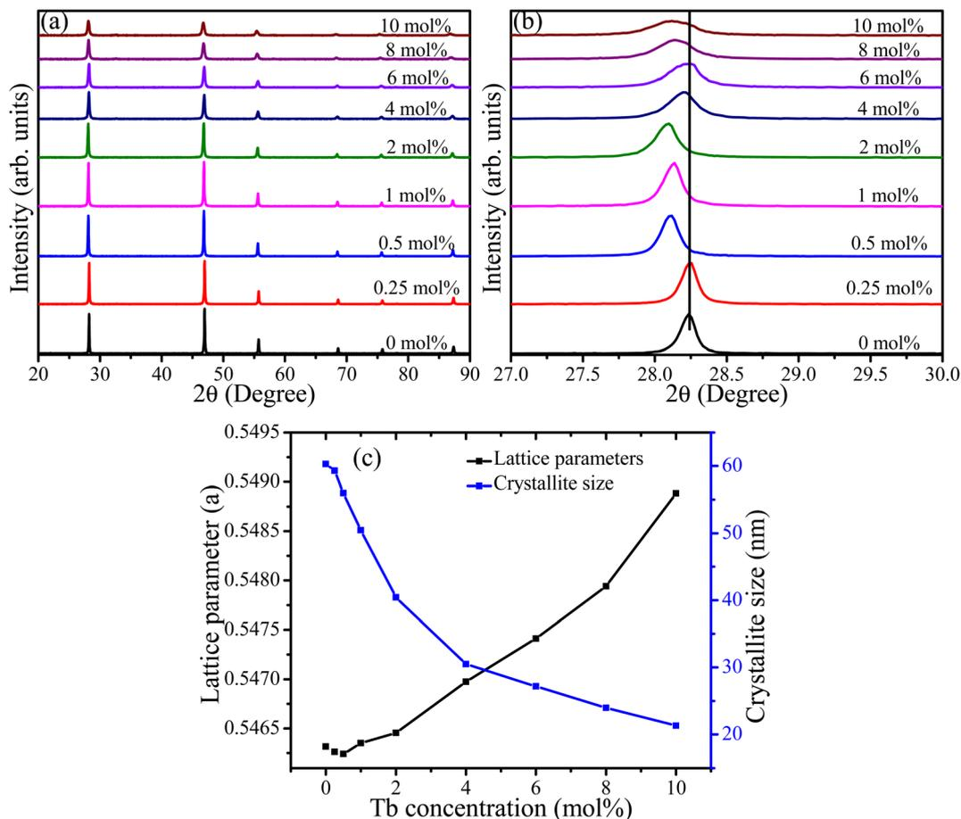
Fig. 1 (a) XRD patterns of CaF<sub>2</sub> nanoparticles doped with different concentrations of Tb<sup>3+</sup> ions, (b) zoomed-in region of the 111 peak, and (c) the calculated lattice parameters and crystallite sizes.
