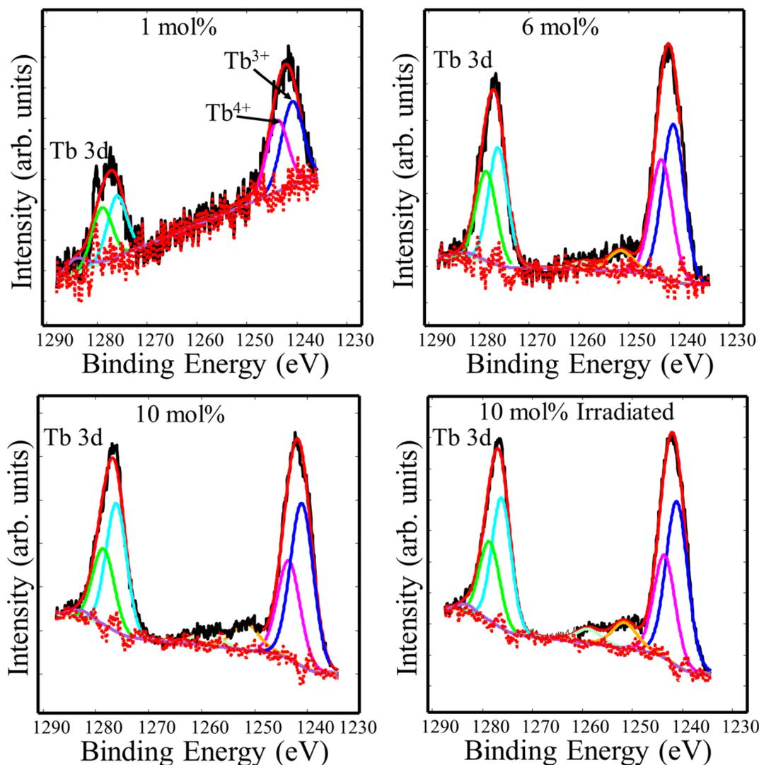
Fig. 5 XPS high resolution spectra of Tb 3d of the CaF<sub>2</sub> doped with different Tb concentrations.
