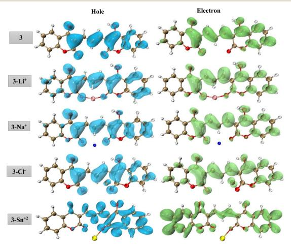
Fig. 10 Real-space representation of hole (blue) and electron (green) distributions for the main transitions of 3 and its complexes with  $Sn^{2+}$ ,  $Li^+$ ,  $Na^+$ , and  $Cl^-$  (isovalue = 0.001).
