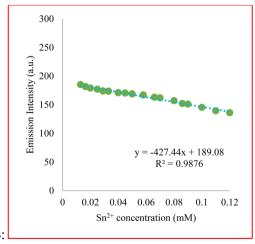
Fig. 2 (A) Fluorescence spectra of compound 3 ( $2.0 \times 10^{-4}$  M) with the addition of various concentrations of Sn<sup>2+</sup> (0–0.2 mM,  $\lambda_{ex}$  = 480 nm). (B) The SnCl<sub>2</sub> concentration effect on fluorescence quenching.
