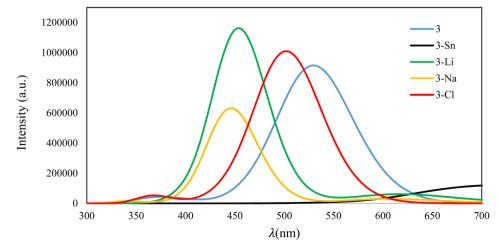
Fig. 9 Fluorescence emission of 3 and its complexes with Sn<sup>2+</sup>, Li<sup>+</sup>, Na<sup>+</sup>, and Cl<sup>-</sup> ions in EtOH–H<sub>2</sub>O (2/3) solvent.
