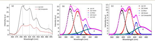
Fig. 3 PL spectra: (a) the optical properties analysis spectra for zinc oxide and silver–copper–zinc composite, (b and c) the deconvoluted zinc oxide and silver–copper–zinc composite spectra, respectively. The intensity reduction for the composites than ZnO indicates a reduction in the electron–hole recombination process. The deconvoluted spectra for the composite show intensity reduction than zinc oxide (see the ellipse curve), which confirms its greater visible light absorption capacity.
