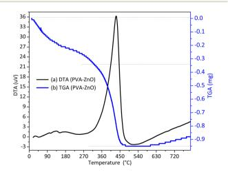
Fig. 1 TGA-DTA thermograms: the thermal decomposition behavior of poly(vinyl alcohol)/fuel-zinc nitrate complex; the two decomposition points are due to the surface/crystal adsorbed water molecules and total decomposition of PVA polymer.
