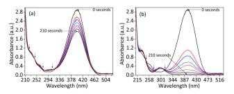
Fig. 8 4-NP catalytic reduction plots of (a) ZnO NPs and (b) silvercopper-zinc composite: The NCs show complete reduction of the 4nitrophenol to the 4-aminophenol within 210 seconds.
