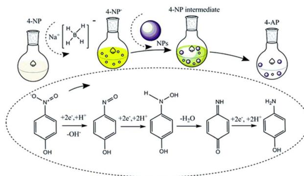
Fig. 9 Possible understanding of the conversion of 4-nitrophenol to 4-aminophenol using  $\text{NaBH}_4$  and metal NPs as an  $\text{H}_2$  source and catalyst, respectively. Reproduced/Adapted from ref. 1 with permission from The Royal Society of Chemistry.
