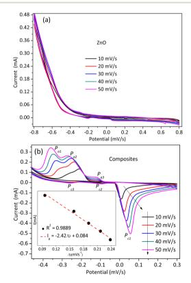
Fig. 7 The CV voltammogram: the CV analysis for (a) zinc oxide and (b) silver–copper–zinc composite: the inset is peak current *versus* square root of potential linear plot. No clear redox peak was detected for zinc oxide, and there is a redox peak for the composites, indicating proton intercalation and de-intercalation due to porosity. The fitting of the linear plot indicates diffusion-controlled charge transfer processes.
