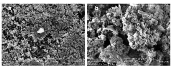
Fig. 4 SEM images: SEM morphological analysis images of (a) zinc oxide and (b) silver–copper–zinc composite. The composite SEM image showed greater porosity, probably the enhanced combustion and gas evolution ability of copper and silver precursors in the presence of fuel/surfactant.
