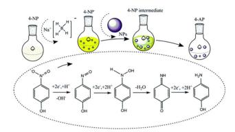
Fig. 9 Possible understanding of the conversion of 4-nitrophenol to 4-aminophenol using NaBH<sub>4</sub> and metal NPs as an H<sub>2</sub> source and catalyst, respectively. Reproduced/Adapted from ref. 1 with permission from The Royal Society of Chemistry.
