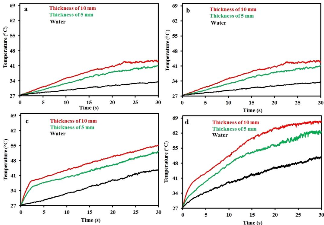
Fig. 7 Temperature changes with time under the light illumination for water and CMB foam with 5 and 10 mm thickness under the light intensity of (a) 800, (b) 1000, (c) 1200, and (d) 1400 W m<sup>-2</sup>.
