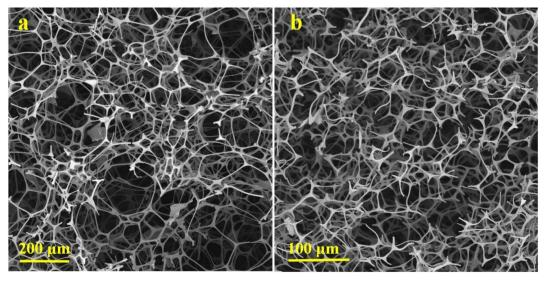
Fig. 2 SEM micrographs of (a) MF and (b) carbonized MF at 800 °C.
