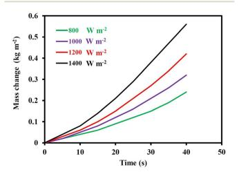
Fig. 8 Mass changes with time for CMB with 10 mm thickness under the light intensities of 800, 1000, 1200, and 1400 W  $m^{-2}$ .
