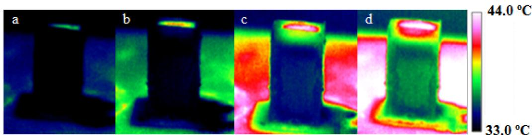
Fig. 6 Infrared images of CMB sample as the temperature response under light irradiation with an intensity of 1400 W m<sup>-2</sup> after (a) 30 s, (b) 90 s, (c) 180 s and (d) 270 s.
