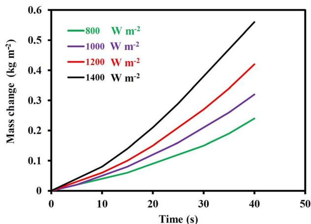
Fig. 8 Mass changes with time for CMB with 10 mm thickness under the light intensities of 800, 1000, 1200, and 1400 W m<sup>-2</sup>.
