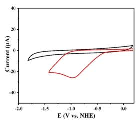
Fig. 4 Cyclic voltammogram of p-methoxy aryldiazonium tetra-fluoroborates salt 2a (red, 1 mM) and blank (black). Supporting electrolyte LiClO<sub>4</sub> (0.1 M); scan rate 0.1 V s<sup>-1</sup>.
