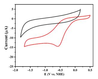
Fig. 6 Cyclic voltammogram of p-fluoro aryldiazonium tetra-fluoroborates salt **2d** (red, 1 mM) and blank (black). Supporting electrolyte LiClO<sub>4</sub> (0.1 M); scan rate 0.1 V s<sup>-1</sup>.
