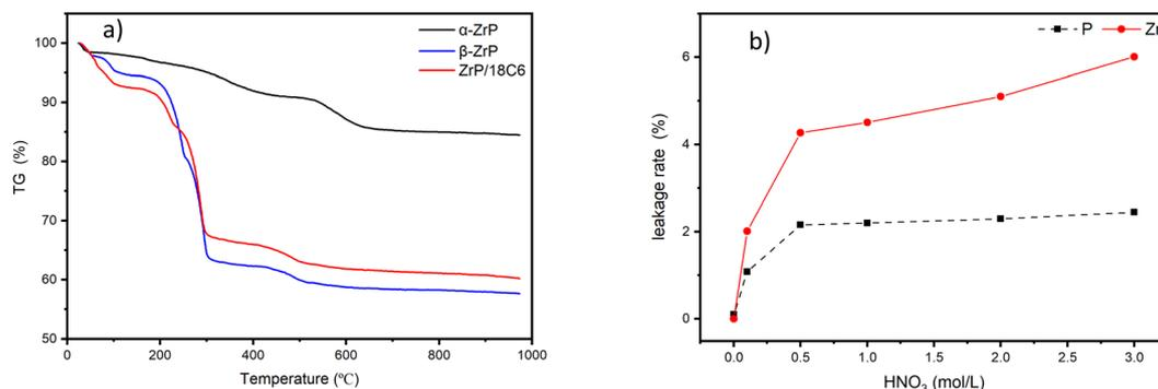
Fig. 5 Stability investigation of adsorbents. (a) TGA curves for  $\alpha$ -ZrP,  $\beta$ -ZrP, and ZrP/18C6 at the temperature from 30 °C to 950 °C. (b) Leakage rates of P and Zr for ZrP/18C6 at different  $\text{HNO}_3$  concentrations for 24 h.
