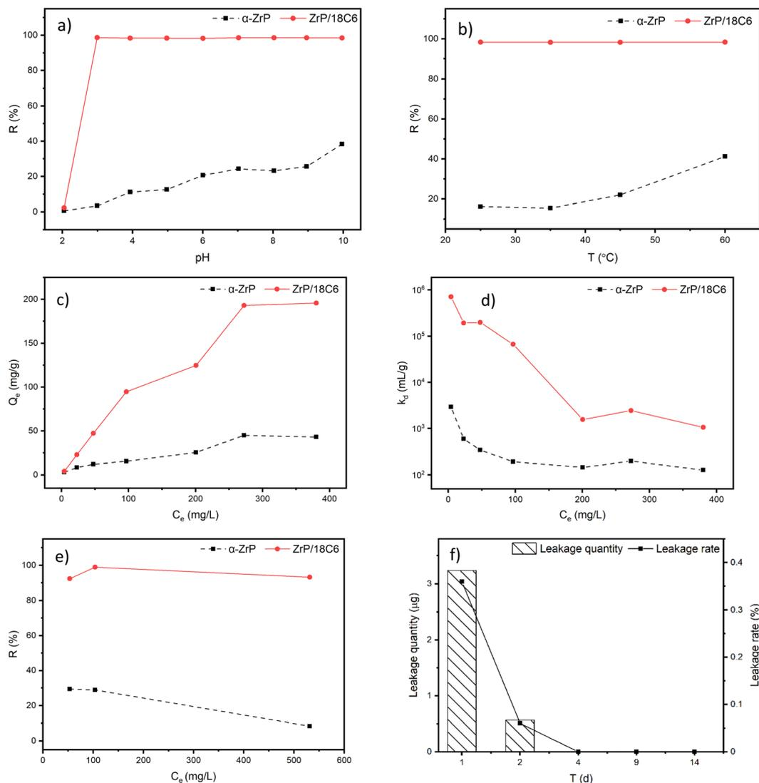
Fig. 7 (a) Effect of pH in the solution. (b) Effect of temperature in the solution. (c and d) Effect of  $Sr^{2+}$  concentration. (e) Effect of competing ions concentration. (f) The leakage amount of  $Sr^{2+}$  from ZrP/18C6 immersed water after  $Sr^{2+}$  adsorption.
