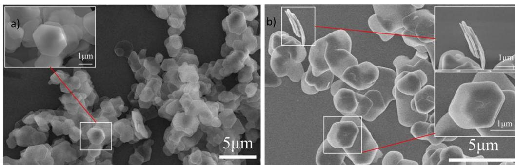
Fig. 4 SEM images of adsorbents, (a)  $\alpha$ -ZrP, (b) ZrP/18C6.
