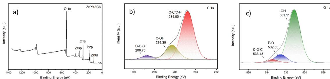
Fig. 3 XPS spectra of ZrP/18C6. (a) Full. (b) C 1s. (c) O 1s.
