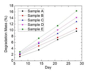
Fig. 7 Mass degradation of PCL-HA-collagen scaffold sample
