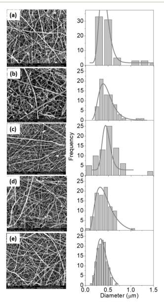
Fig. 4 SEM results (right) and fiber diameter distribution histogram (left) for samples with different ratio of PCL: HA: collagen; A (50: 45: 5), B (50:40:10), C (50:35:15), D (50:30:20), and E (50:25:25).
