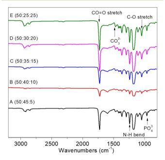
Fig. 3 FTIR spectrum results of PCL: HA: collagen scaffold.
