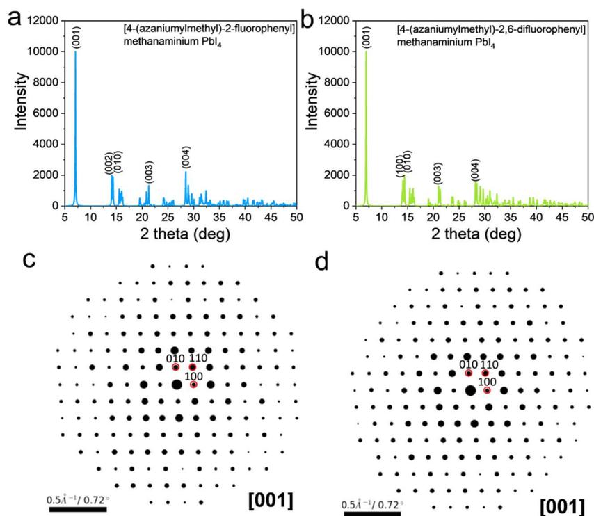
Fig. 3 The X-ray and electron diffraction patterns of [4-(azaniumylmethyl)-2-fluorophenyl] methanaminium  $\text{PbI}_4$  and [4-(azaniumylmethyl)-2,6-difluorophenyl] methanaminium  $\text{PbI}_4$ . (a and b) The X-ray diffraction patterns. ( $\lambda = 1.54 \text{ \AA}$ ) (c and d) The electron diffraction patterns ( $\lambda = 0.025 \text{ \AA}$ ).
