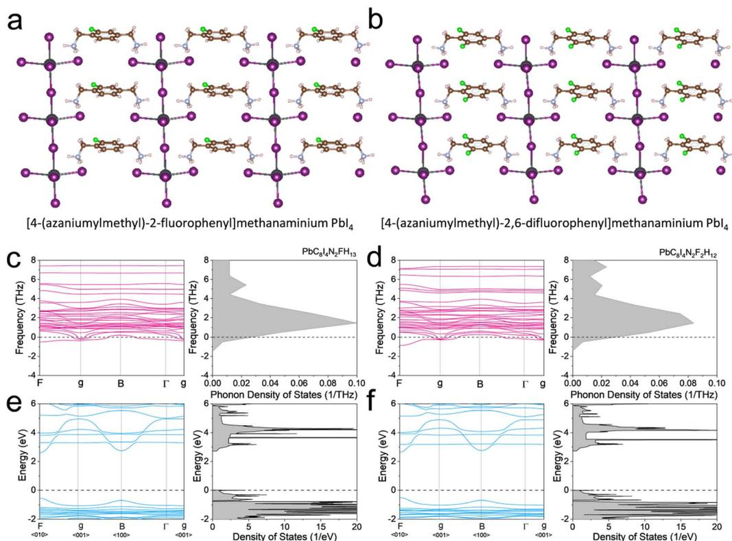
Fig. 2 The crystal structure, phonon band diagrams, and electron band diagrams of [4-(azaniumylmethyl)-2-fluorophenyl] methanaminium  $\text{PbI}_4$  and [4-(azaniumylmethyl)-2,6-difluorophenyl] methanaminium  $\text{PbI}_4$ . (a and b) The crystal structures (c and d) The phonon band diagrams. (e and f) The electron band diagrams.
