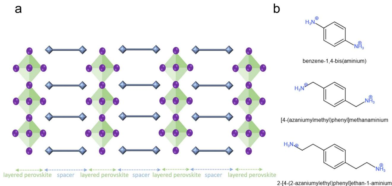
**Fig. 1** The two-dimensional Dion–Jacobson perovskite and different spacer cations. (a) The 2D DJ layer structures are composed of a diammonium organic spacer layer (blue) and a 2D metal halide perovskite layer. (b) The typical two-diammonium aromatic spacer cations.
