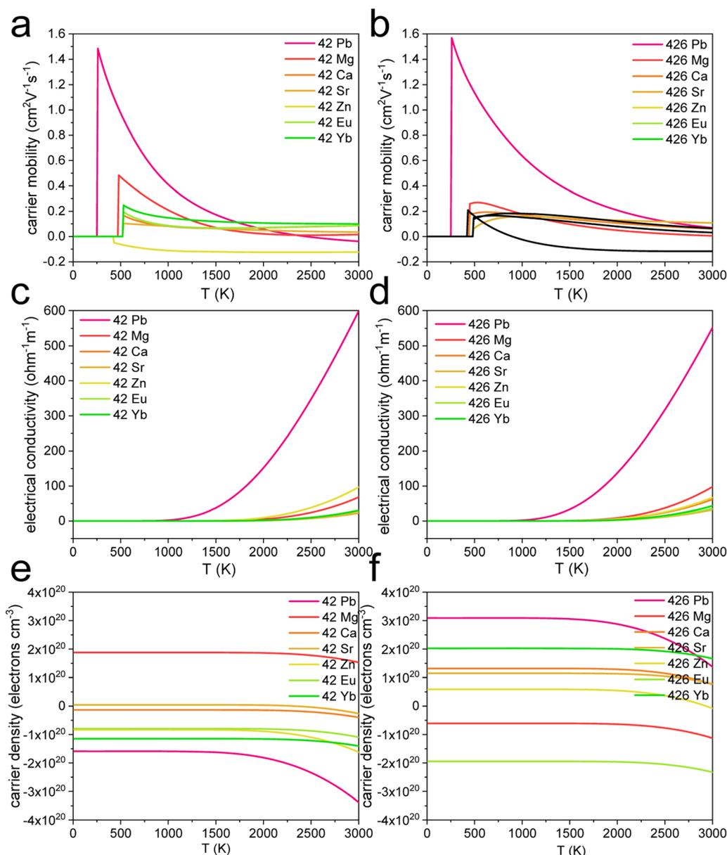
Fig. 4 The carrier mobility, electrical conductivity, and carrier density of [4-(azaniumylmethyl)-2-fluorophenyl] methanaminium  $\text{XI}_4$  and [4-(azaniumylmethyl)-2,6-difluorophenyl] methanaminium  $\text{XI}_4$ . (X = Pb, Mg, Ca, Sr, Zn, Eu, and Yb) (a and b) The carrier mobilities. (c and d) The electrical conductivities. (e and f) The carrier densities.
