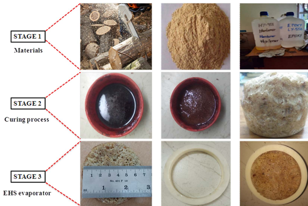
Fig. 2 Fabrication of the circular type epoxy/hardener/sawdust composite.
