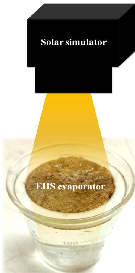
Fig. 3 Solar steam generation experimental setup.
