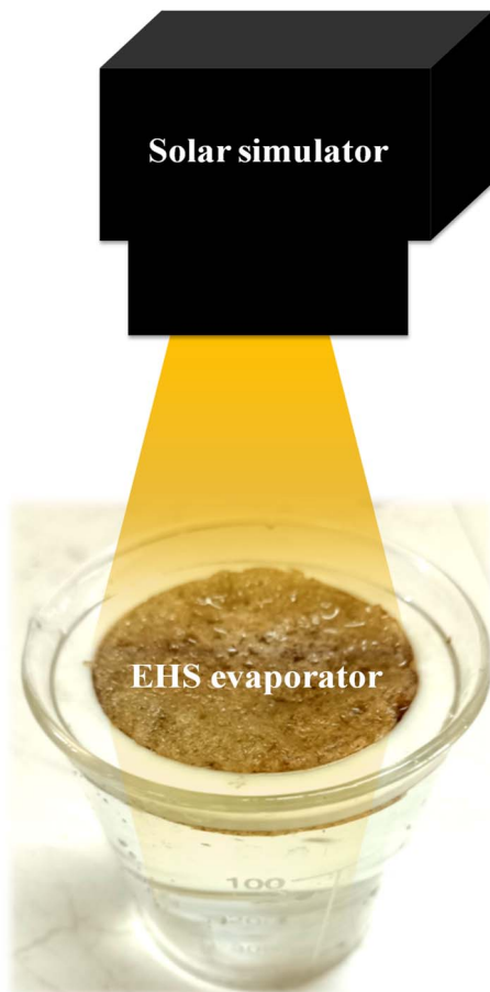
Fig. 3 Solar steam generation experimental setup.
