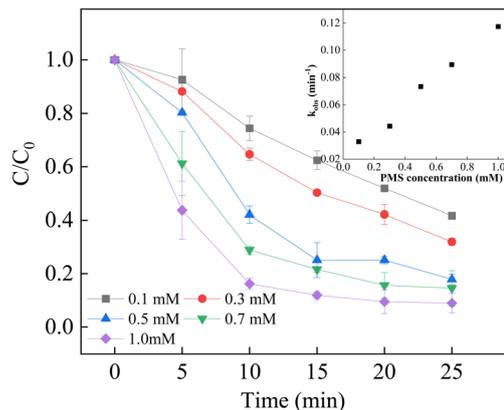
Fig. 7 Effect of PMS concentration on BPA degradation. Reaction conditions: [BPA] = 0.05 mM, [PMS] = 0.1–1.0 mM, [LCO] = 0.5 g L<sup>-1</sup>, initial PH = 6.8.
