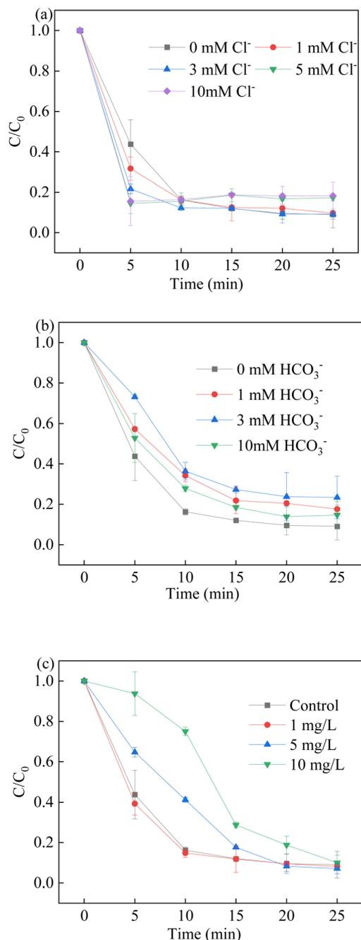
Fig. 9 Effect of co-existing ions (a)  $Cl^-$ ; (b)  $HCO_3^-$  and (c) natural organic matter on BPA degradation. Reaction conditions: [BPA] = 0.05 mM, [PMS] = 1.0 mM, [LCO] = 0.5 g L<sup>-1</sup>, initial pH = 6.8.
