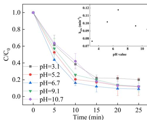
Fig. 8 Effect of initial pH on BPA degradation. Reaction conditions: [BPA] = 0.05 mM, [PMS] = 1.0 mM, [LCO] = 0.5 g L<sup>-1</sup>, initial PH = 3.1–9.1.
