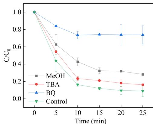
Fig. 10 Effect of radical scavengers on BPA degradation. Reaction conditions: [BPA] = 0.05 mM, [PMS] = 1.0 mM, [LCO] = 0.5 g L<sup>-1</sup>, initial PH = 6.8, [scavengers] = 0.2 M.
