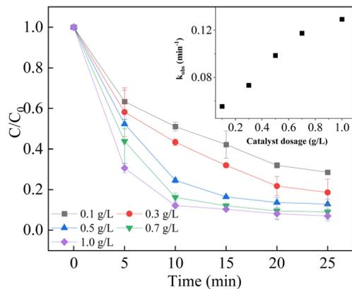
Fig. 6 Effect of catalyst dosage on BPA degradation. Reaction conditions: [BPA] = 0.05 mM, [PMS] = 1.0 mM, [LCO] = 0.1–1.0 g L<sup>-1</sup>, initial PH = 6.8.
