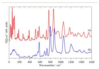
Fig. 5 Comparison of the calculated (a) and experimental (b) INS spectra of polythiophene.
