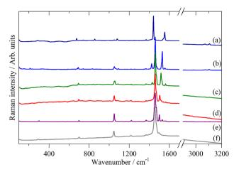
Fig. 3 FT-Raman spectra of the oligothiophenes and polythiophene. (a) 2T, (b) 3T, (c) 4T, (d) 6T, (e) 8T and (f) PT
