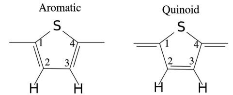
Fig. 11 Illustration of the benzenoid and quinoid structures in PT. Adapted from ref. 66 under a Creative Commons Attribution 4.0 International License.
