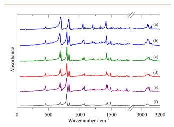
Fig. 2 Infrared spectra of the oligothiophenes and polythiophene. (a) 2T, (b) 3T, (c) 4T, (d) 6T, (e) 8T and (f) PT.
