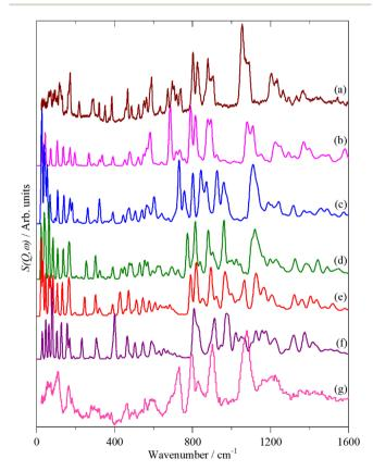
Fig. 13 Observed and calculated INS spectra of doped 4T. (a) Experimental neutral molecule spectrum, calculated spectra of (b) neutral, (c) +1, (d) +2, (e) +3, (f) +4 and (g) experimental  $I_2$ -doped molecule spectrum.
