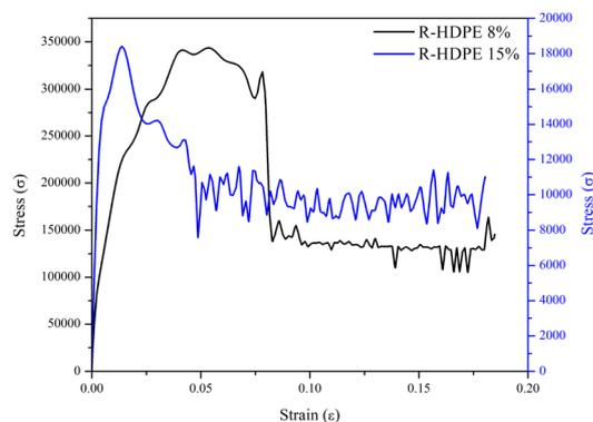
Fig. 6 Stress–strain curves of the HDPE membranes.
