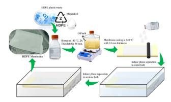
Fig. 1 Preparation scheme of the HDPE membrane.
