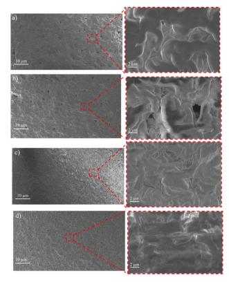
Fig. 4 Surfaces of the HDPE membranes: (a) R-HDPE 8%, (b) R-HDPE 10%, (c) R-HDPE 13%, and (d) R-HDPE 15%.
