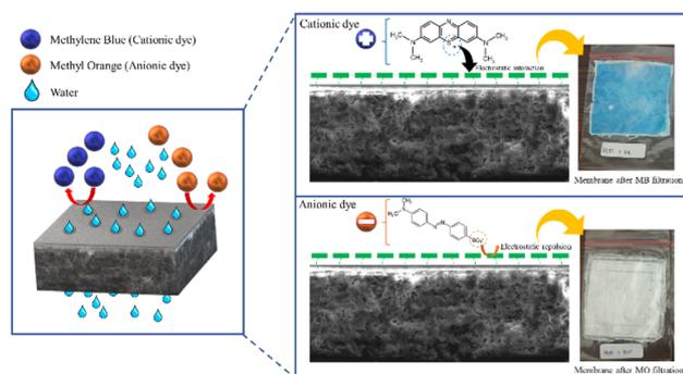
Fig. 10 Dye removal scheme.
