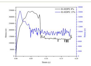
Fig. 6 Stress-strain curves of the HDPE membranes.
