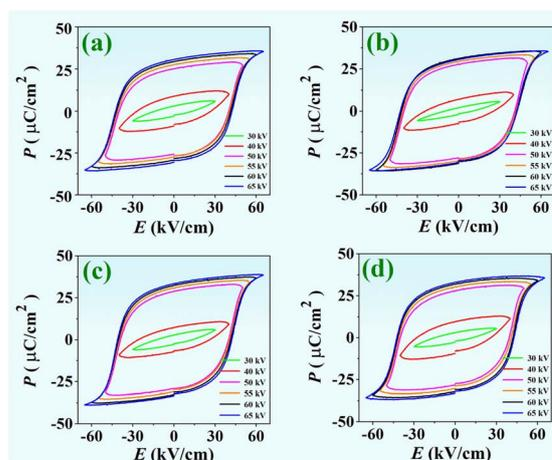
Fig. 8 Polarization–electric field ( $P$ – $E$ ) hysteresis loop of the BNKT/0.01ZnO ceramics annealed at  $950 \text{ }^\circ\text{C}$  with different annealing times, measured at RT under various electric field of 30–65  $\text{kV cm}^{-1}$ , where (a) 0 h, (b) 4 h, (c) 8 h, and (d) 12 h.
