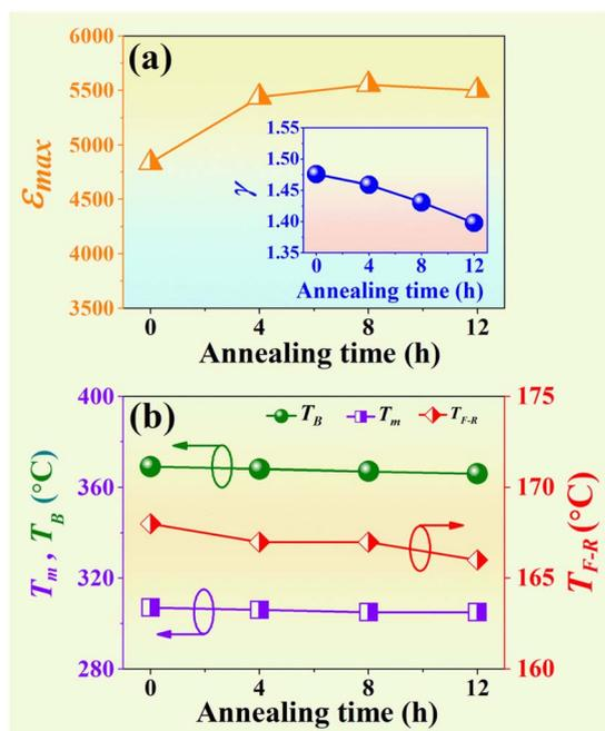
**Fig. 6** Plot of (a)  $\epsilon_{max}$  as a function of annealing time (inset: the  $\gamma$  value as various annealing times), and (b)  $T_m$ ,  $T_B$ , and  $T_{F-R}$  values as a function of annealing time.
