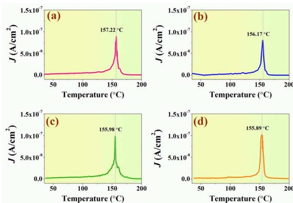
Fig. 7 Plots current density–temperature ( $J$ – $T$ ) from the TSDC technique of the BNKT/0.01ZnO ceramics annealed at 950 °C with different annealing times, where (a) 0 h, (b) 4 h, (c) 8 h, and (d) 12 h.
