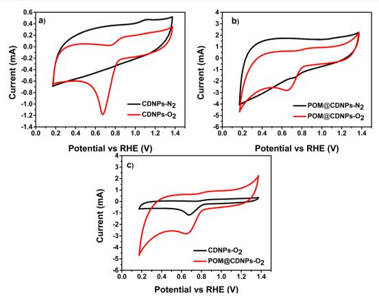
Fig. 7 CVs of (a) CDNPs and (b) POM@CDNPs in both  $N_2$ - and  $O_2$ -saturated electrolytes and (c) a comparison for both samples in  $O_2$ -saturated electrolyte recorded at a scan rate of 50 mV s<sup>-1</sup>.
