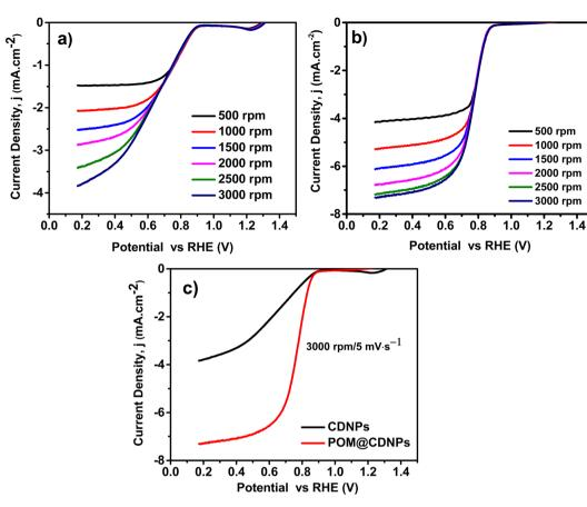
Fig. 8 LSVs of (a) CDNPs, and (b) POM@CDNPs recorded at different speeds from 500 to 3000 rpm, and (c) a comparison of the LSVs for the electro-catalysts recorded at 3000 rpm and a scan rate of 5 mV s<sup>-1</sup>.
