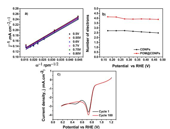
Fig. 9 (a) Linear Koutecky-Levich plots K-L plots of POM@CDNPs at different potentials from 0.5 to 0.8 V derived from LSV, (b) the number of electrons values of CDNPs and POM@CDNPs, and (c) the 1st and 100th cycles of POM@CDNPs recorded at 3000 rpm at a scan rate of 50 mV s<sup>-1</sup>
