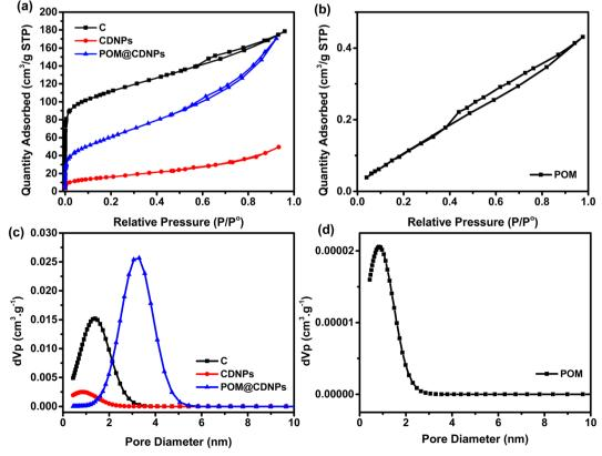
Fig. 3 (a) and (b) N<sub>2</sub> adsorption/desorption isotherms for the prepared materials and (c) and (d) their corresponding pore diameters.
