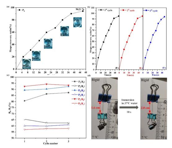
Fig. 4 (a) The shape recovery ratio of elastomer  $P_2$ . (b) The shape recovery ratio of the obtained sample  $P_2$  within three cycles. (c)  $R_r$  and  $R_f$  curves of polymers  $P_1-P_3$ . (d) The shape changes of  $P_2$  as a response to body temperature.
