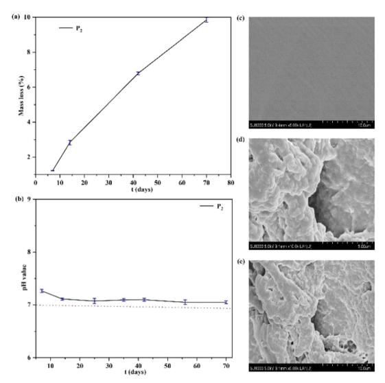
Fig. 5 (a) The mass loss curve of polymer  $P_2$  with increasing number of days. (b) The pH curve of polymer  $P_2$  with increasing number of days. (c, d and e) SEM images ( $\times$ 5.0 K,  $\times$ 10.0 K) of polymer  $P_2$  before and after degradation at 37 °C.
