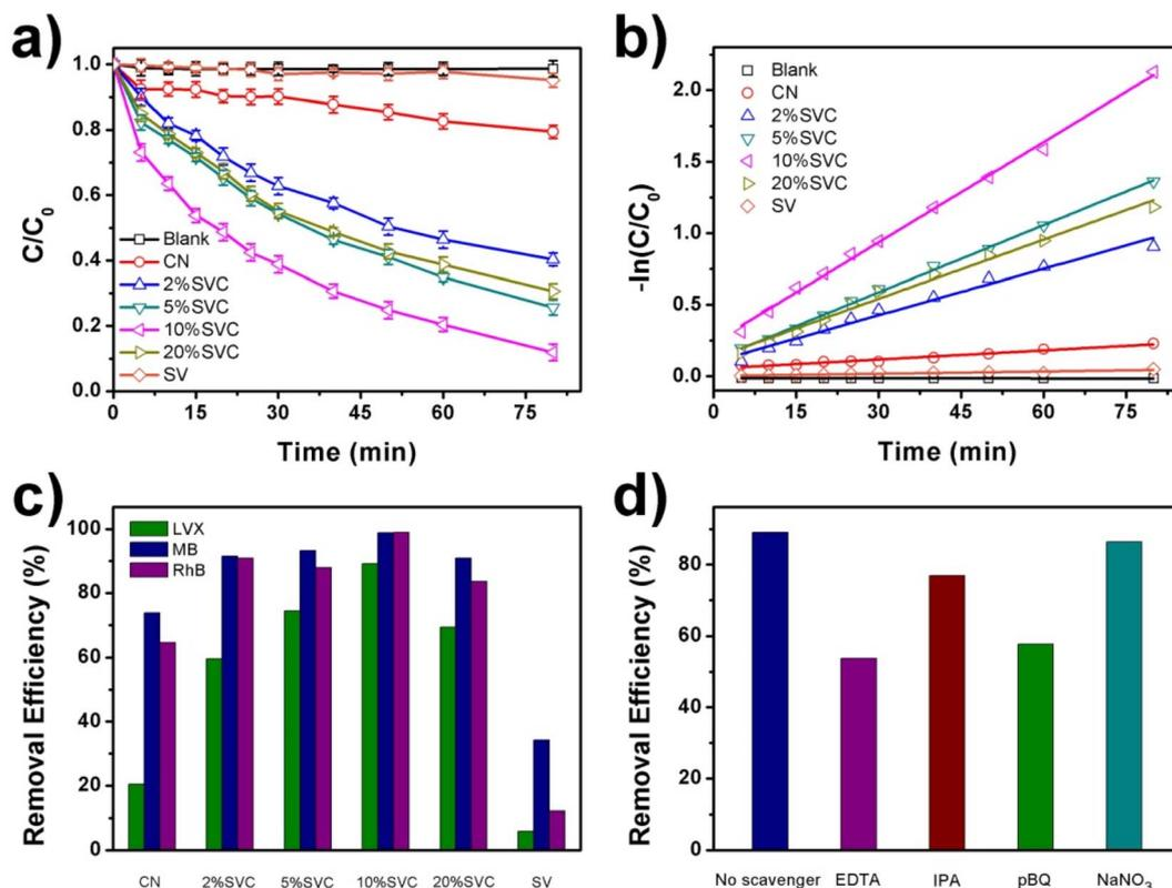
Fig. 7 (a) Photocatalytic degradation of LVX over CN, SVCs and SV under visible light irradiation, (b) corresponding first-order kinetics fitting plots, (c) removal efficiency of LVX, MB and RhB over 10%SVC and (d) the effect of radical scavengers on the photocatalytic degradation of LVX over 10%SVC [experimental conditions:  $V = 200$  mL;  $LVX = 12.0$  mg  $L^{-1}$ ; catalyst dosage =  $0.5$  g  $L^{-1}$ ].
