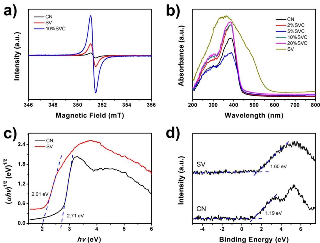
Fig. 6 (a) EPR spectra of CN, SV and 10%SVC, (b) UV-vis diffuse reflectance spectra of CN, SV and SVCs, (c) XPS VB spectra and (d) band gap energies of CN and SV.
