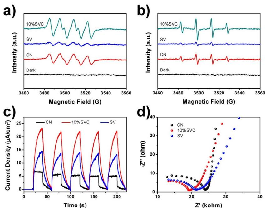
Fig. 8 ESR spectra of (a) DMPO··O<sub>2</sub><sup>-</sup> in methanol and (b) DMPO··OH in water with the presence of CN, 10%SVC and SV, (c) TPC spectra and (d) EIS Nyquist plots of CN, 10%SVC and SV.
