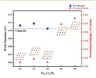
Fig. 2 The work functions and the formation enthalpies of Fe(110) surface doped with three Cr atoms and one Ni atom. The illustrations show the corresponding atomic structures of the first layer of Fe(110) surface. The yellow atoms, blue atoms and white atoms represent Fe, Cr and Ni, respectively. The dashed line indicates the work function of the clean Fe surface.
