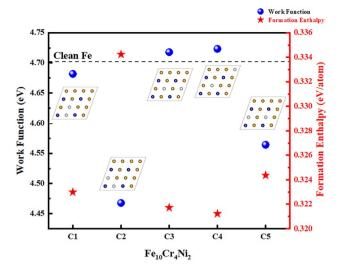
Fig. 4 The work functions and the formation enthalpies of Fe(110) surface doped with four Cr atoms and two Ni atoms. The illustrations show the corresponding atomic structures of the first layer of Fe(110) surface.
