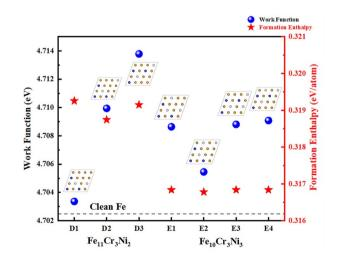
Fig. 5 The work functions and the formation enthalpies of Fe(110) surface doped with three Cr atoms and two Ni atoms (D1, D2, D3), four Cr atoms and two Ni atoms (E1, E2, E3, E4). The illustrations show the corresponding atomic structures of the first layer of Fe(110) surface.
