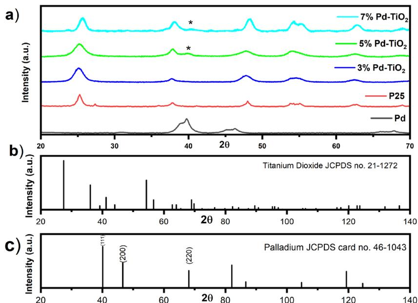
Fig. 2 (a) XRD patterns of Pd-metal, TiO<sub>2</sub> P25, 3% Pd–TiO<sub>2</sub>, 5% Pd–TiO<sub>2</sub> and 7% Pd–TiO<sub>2</sub> nanoparticles, (b) pattern of JCPDS no. 21-1272 and (c) JCPDS card no. 46-1043 respectively.
