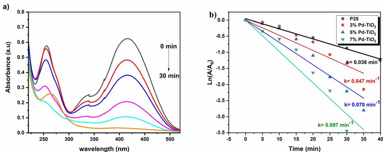
Fig. 6 (a) UV-vis absorption spectra of  $5 \times 10^{-5}$  M RY15 aqueous solution as a function of photoirradiation time with  $0.1 \text{ g L}^{-1}$  of 5 wt% Pd– $\text{TiO}_2$  photocatalyst, (b) the 1st order rate kinetics of the photocatalytic degradation reactions of RY15 using different plasmonic Pd– $\text{TiO}_2$  photocatalysts compared with P25 under UV-vis simulated sunlight illumination.
