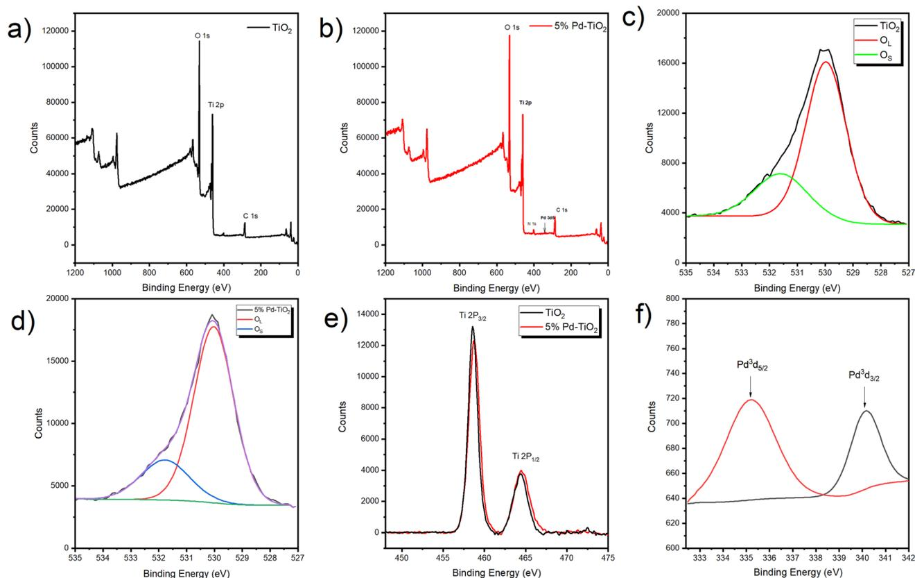
Fig. 3 XPS analysis of elements present in P25 and 5% Pd-TiO<sub>2</sub> (a and b) survey, (c and d) oxygen, (e) Ti, and (f) Pd.
