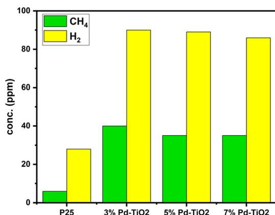
Fig. 8 Bar presentation for the generated amounts of CH<sub>4</sub> and H<sub>2</sub> gases in ppm after 4 h of illumination.
