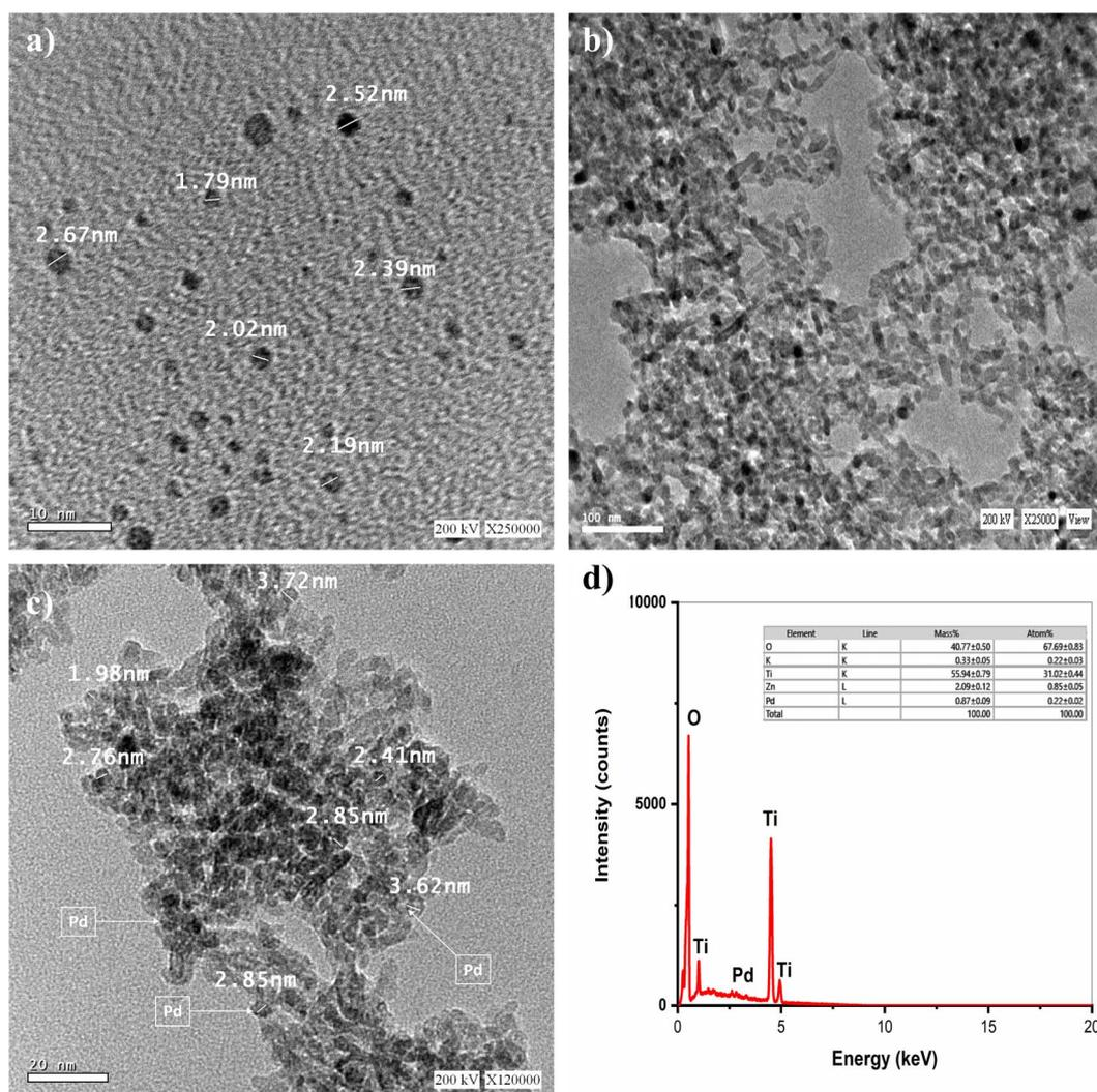
Fig. 1 HR-TEM images of: (a) Pd-metal; (b) TiO<sub>2</sub> P25; (c) 5% Pd-TiO<sub>2</sub>; (d) EDX-analysis of 5% Pd-TiO<sub>2</sub>.
