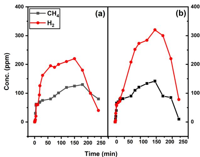
Fig. 9 Methane and hydrogen generation rates in ppm as a function of irradiation time produced from the photocatalytic destruction of RY15 dye pollutants using P25 and 5% Pd–TiO<sub>2</sub> photocatalysts.
