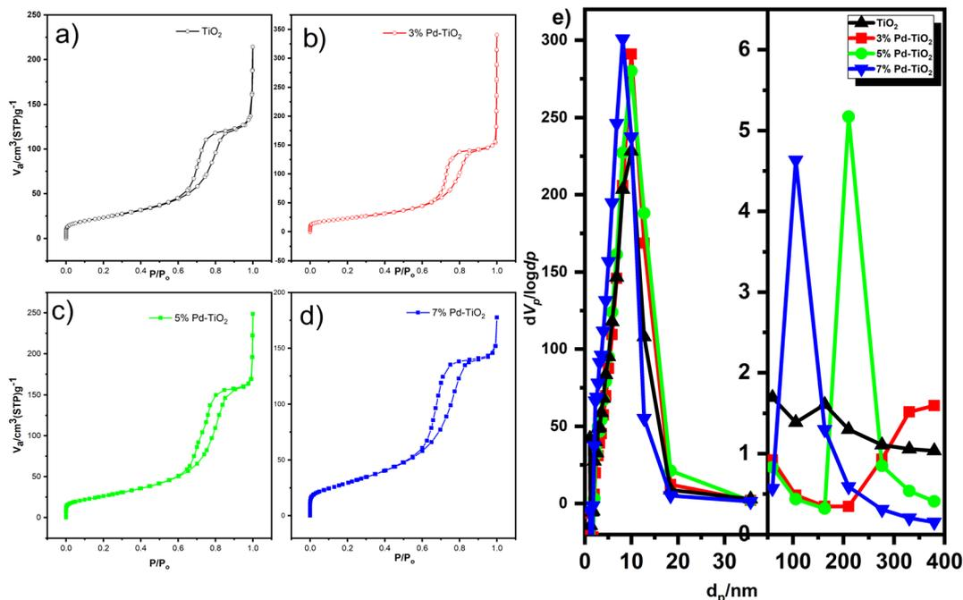
Fig. 5 Adsorption–desorption isotherms (a)  $\text{TiO}_2$  (b) 3% Pd– $\text{TiO}_2$  (c) 5% Pd– $\text{TiO}_2$  (d) 7% Pd– $\text{TiO}_2$ ; and (e) pore size distribution of prepared  $\text{TiO}_2$ , 3 wt% Pd– $\text{TiO}_2$ , 5 wt% Pd– $\text{TiO}_2$  and 7 wt% Pd– $\text{TiO}_2$  photocatalysts.
