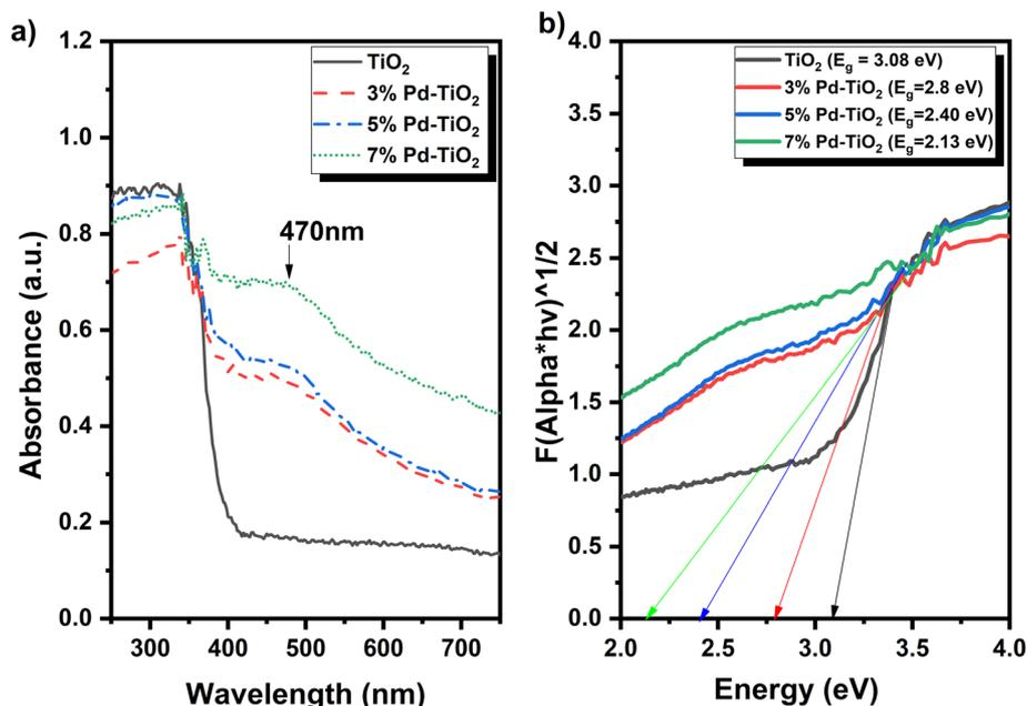
Fig. 4 (a) UV-vis absorption spectra; and (b) band gap energies of P25, 3 wt% Pd-TiO<sub>2</sub>, 5 wt% Pd-TiO<sub>2</sub> and 7 wt% Pd-TiO<sub>2</sub> photocatalysts.
