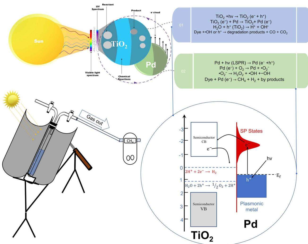
Fig. 10 A mechanistic schematic diagram of the occurred reactions in the photoreaction.
