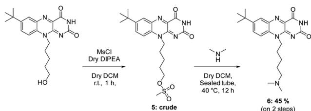
Scheme 2 Synthesis of *t*BdRF-NMe<sub>2</sub>.
