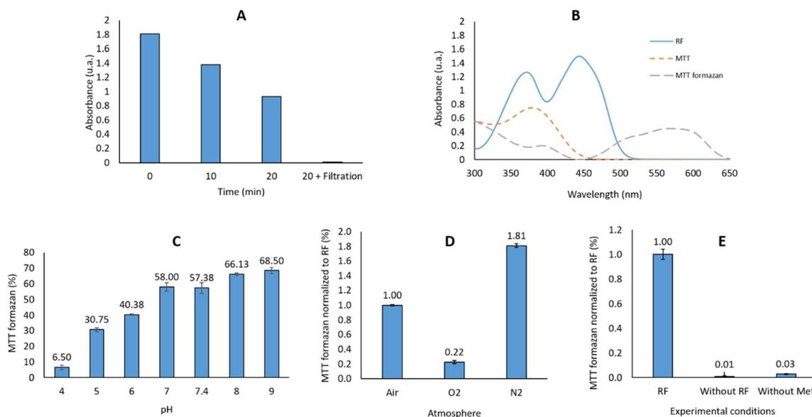
Fig. 2 (A) Absorbance at 560 nm after 0, 10 & 20 min of pause, and after filtration on 0.2  $\mu\text{m}$  filters; (B) UV-Vis spectra of RF (12.8 mM in water), MTT (10.9 mM in water) and MTT-formazan (2.19 mM in THF/water 1/1); (C) influence of the pH on the reaction output; (D) influence of the atmosphere on the reaction output; (E) control reactions: without RF or without methionine.
