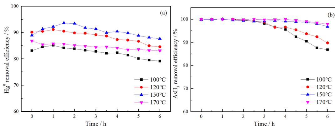
Fig. 4 The effects of the different reaction temperatures on removal efficiencies of  $\text{Hg}^0$  (a) and  $\text{AsH}_3$  (b) over  $\text{Fe}_5\text{Ce}_5\text{Ti}$  catalysts (total gas flow:  $800 \text{ mL min}^{-1}$ , catalyst filling capacity: 200 mg,  $\text{Hg}^0$ :  $400 \mu\text{g m}^{-3}$ ,  $\text{AsH}_3$ : 50 ppm,  $\text{O}_2$ : 1 vol%, CO: 80 vol%, reaction temperature: 100–170 °C).
