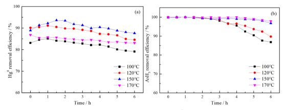
Fig. 4 The effects of the different reaction temperatures on removal efficiencies of  $Hg^0$  (a) and  $AsH_3$  (b) over  $Fe_5Ce_5Ti$  catalysts (total gas flow: 800 mL min<sup>-1</sup>, catalyst filling capacity: 200 mg,  $Hg^0$ : 400  $\mu$ g m<sup>-3</sup>,  $AsH_3$ : 50 ppm,  $O_2$ : 1 vol%, CO: 80 vol%, reaction temperature: 100–170 °C).
