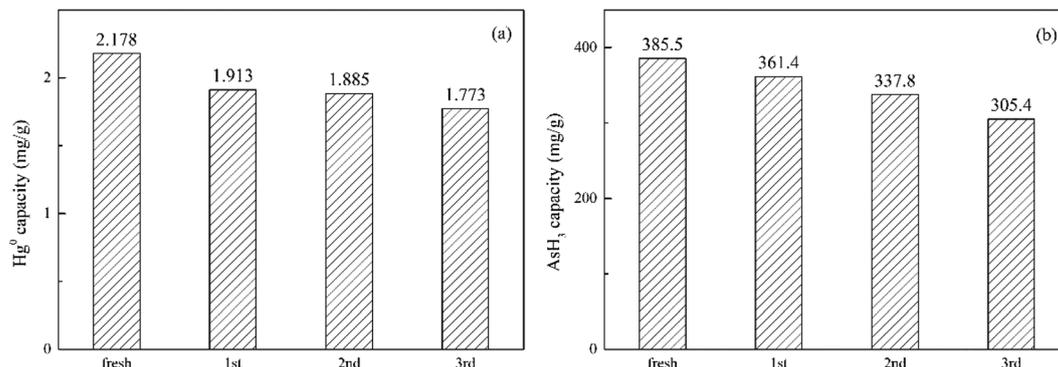
Fig. 9 Hg<sup>0</sup> and AsH<sub>3</sub> adsorption tests after regeneration (total gas flow: 800 mL min<sup>-1</sup>, catalyst filling capacity: 200 mg, Hg<sup>0</sup>: 400 μg m<sup>-3</sup>, AsH<sub>3</sub>: 50 ppm, O<sub>2</sub>: 1 vol%, CO: 80 vol%, reaction temperature: 150 °C).
