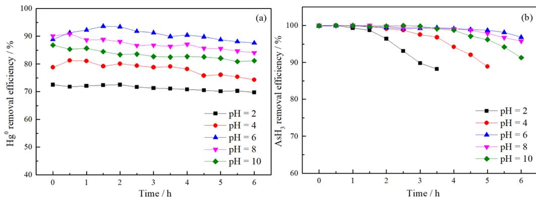
Fig. 3 The effects of the sol pH on the removal efficiencies of Hg<sup>0</sup> (a) and AsH<sub>3</sub> (b) over Fe<sub>5</sub>Ce<sub>5</sub>Ti catalysts (total gas flow: 800 mL min<sup>-1</sup>, catalyst filling capacity: 200 mg, Hg<sup>0</sup>: 400 μg m<sup>-3</sup>, AsH<sub>3</sub>: 50 ppm, O<sub>2</sub>: 1 vol%, CO: 80 vol%, reaction temperature: 150 °C).
