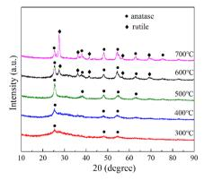
Fig. 7 XRD patterns of  $Fe_5Ce_5Ti$  catalysts at different calcination temperatures.
