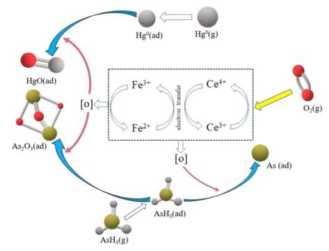
Fig. 10 Reaction mechanism for the removal of Hg<sup>0</sup> and AsH<sub>3</sub>.
