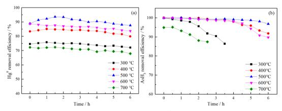
Fig. 2 The effects of the calcination temperature on the removal efficiencies of  $Hg^0$  (a) and  $AsH_3$  (b) over  $Fe_5Ce_5Ti$  catalysts (total gas flow: 800 mL min<sup>-1</sup>, catalyst filling capacity: 200 mg,  $Hg^0$ : 400  $\mu$ g m<sup>-3</sup>,  $AsH_3$ : 50 ppm,  $O_2$ : 1 vol%, CO: 80 vol%, reaction temperature: 150 °C).
