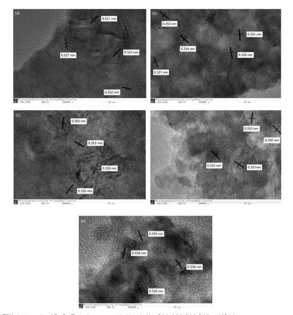
Fig. 6 HR-TEM photographs of  $Fe_5Ce_5Ti$  catalysts prepared with sol pH = 2 (a), 4 (b), 6 (c), 8 (d) and 10 (e).
