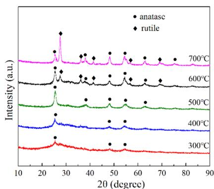
Fig. 7 XRD patterns of  $\text{Fe}_5\text{Ce}_5\text{Ti}$  catalysts at different calcination temperatures.
