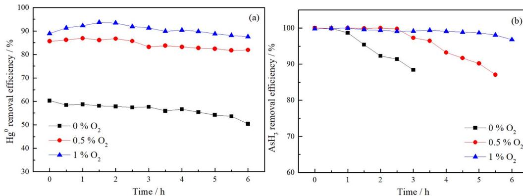
Fig. 5 The effects of O<sub>2</sub> concentration on the removal efficiencies of Hg<sup>0</sup> (a) and AsH<sub>3</sub> (b) over Fe<sub>5</sub>Ce<sub>5</sub>Ti catalysts (total gas flow: 800 mL min<sup>-1</sup>, catalyst filling capacity: 200 mg, Hg<sup>0</sup>: 400 μg m<sup>-3</sup>, AsH<sub>3</sub>: 50 ppm, O<sub>2</sub>: 0–1 vol%, CO: 80 vol%, reaction temperature: 150 °C).
