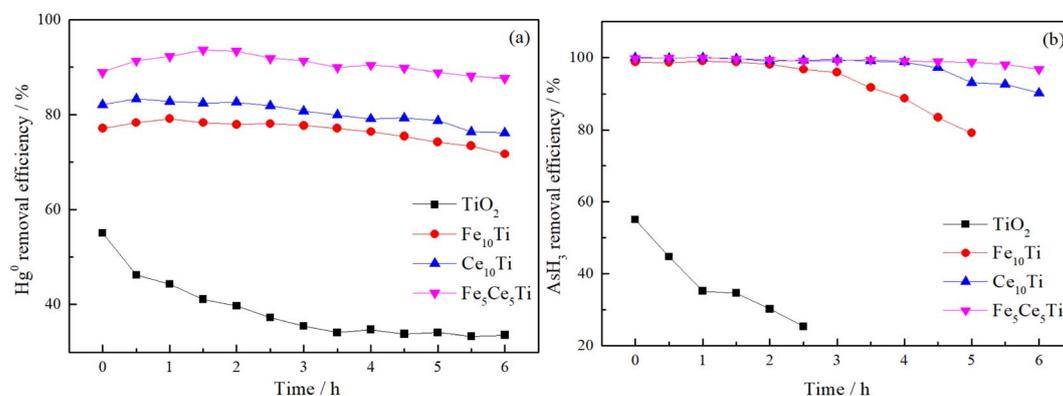
Fig. 1 The effects of active components on the removal efficiencies of Hg<sup>0</sup> (a) and AsH<sub>3</sub> (b) over Fe<sub>x</sub>Ce<sub>y</sub>Ti catalysts (total gas flow:  $800 \text{ mL min}^{-1}$ , catalyst filling capacity: 200 mg, Hg<sup>0</sup>:  $400 \mu\text{g m}^{-3}$ , AsH<sub>3</sub>: 50 ppm, O<sub>2</sub>: 1 vol%, CO: 80 vol%, reaction temperature: 150 °C).
