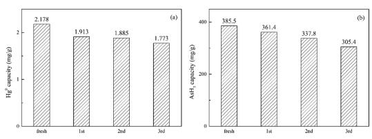
Fig. 9  $Hg^0$  and AsH<sub>3</sub> adsorption tests after regeneration (total gas flow: 800 mL min<sup>-1</sup>, catalyst filling capacity: 200 mg,  $Hg^0$ : 400  $\mu$ g m<sup>-3</sup>, AsH<sub>3</sub>: 50 ppm, O<sub>2</sub>: 1 vol%, CO: 80 vol%, reaction temperature: 150 °C).
