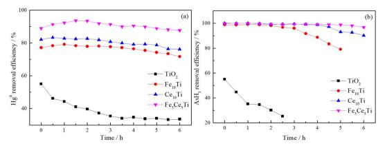
Fig. 1 The effects of active components on the removal efficiencies of  $Hg^0$  (a) and  $AsH_3$  (b) over  $Fe_xCe_yTi$  catalysts (total gas flow: 800 mL min<sup>-1</sup>, catalyst filling capacity: 200 mg,  $Hg^0$ : 400  $\mu$ g m<sup>-3</sup>,  $AsH_3$ : 50 ppm,  $O_2$ : 1 vol%, CO: 80 vol%, reaction temperature: 150 °C).
