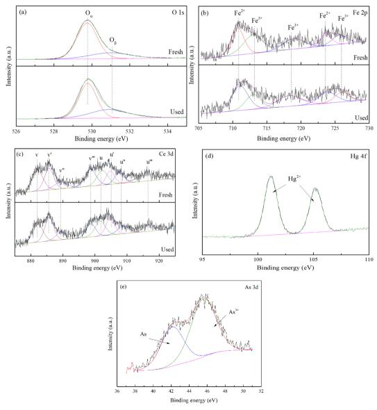
Fig. 8 XPS spectra of O 1s (a), Fe 2p (b), Ce 3d (c), Hq 4f (d) and As 3d (e) for fresh and used Fe<sub>5</sub>Ce<sub>5</sub>Ti catalysts.
