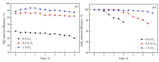
Fig. 5 The effects of  $O_2$  concentration on the removal efficiencies of  $Hg^0$  (a) and  $AsH_3$  (b) over  $Fe_5Ce_5Ti$  catalysts (total gas flow: 800 mL min<sup>-1</sup>, catalyst filling capacity: 200 mg,  $Hg^0$ : 400  $\mu g$  m<sup>-3</sup>,  $AsH_3$ : 50 ppm,  $O_2$ : 0–1 vol%, CO: 80 vol%, reaction temperature: 150 °C).
