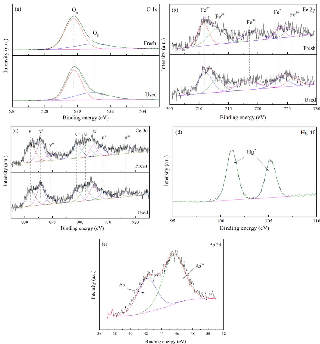
Fig. 8 XPS spectra of O 1s (a), Fe 2p (b), Ce 3d (c), Hg 4f (d) and As 3d (e) for fresh and used Fe<sub>5</sub>Ce<sub>5</sub>Ti catalysts.
