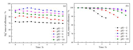
Fig. 3 The effects of the sol pH on the removal efficiencies of  $Hg^0$  (a) and  $AsH_3$  (b) over  $Fe_5Ce_5Ti$  catalysts (total gas flow: 800 mL min<sup>-1</sup>, catalyst filling capacity: 200 mg,  $Hg^0$ : 400  $\mu$ g m<sup>-3</sup>,  $AsH_3$ : 50 ppm,  $O_2$ : 1 vol%, CO: 80 vol%, reaction temperature: 150 °C).
