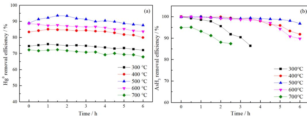
Fig. 2 The effects of the calcination temperature on the removal efficiencies of Hg<sup>0</sup> (a) and AsH<sub>3</sub> (b) over Fe<sub>5</sub>Ce<sub>5</sub>Ti catalysts (total gas flow: 800 mL min<sup>-1</sup>, catalyst filling capacity: 200 mg, Hg<sup>0</sup>: 400 μg m<sup>-3</sup>, AsH<sub>3</sub>: 50 ppm, O<sub>2</sub>: 1 vol%, CO: 80 vol%, reaction temperature: 150 °C).
