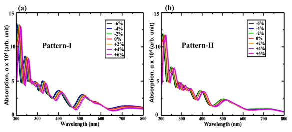
Fig. 10 Strain-induced absorption properties for (a) pattern-I and (b) pattern-II of 2D ZnO/SiC vdW HBLs.
