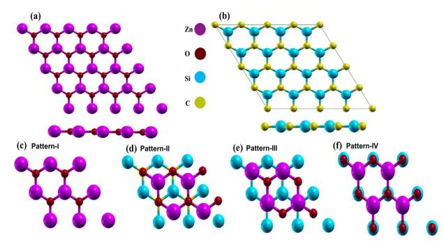
Fig. 1 Relaxed structures of (a) 2D-ZnO, (b) 2D-SiC, (c) pattern-II, (d) pattern-III, (e) pattern-III, and (f) pattern-IV. Violet, deep red, cyan, and golden yellow spheres represent Zn, O, Si, and C, respectively.
