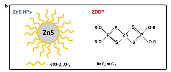
Fig. 1 (a) Pictures showing overall ZnS nanoparticle synthesis process, including setup, conditions, and processing. (b) Model structures of the ZnS NPs and ZDDP. The R represents an alkyl group in ZDDPs.
