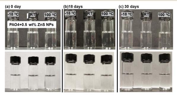
Fig. 2 Pictures showing PAO4 + 0.5 wt% ZnS NPs (a) initial state and after being kept at -18 °C, RT and 100 °C for (b) 18 days and (c) 30 days. Black and white backgrounds were used to visualize the oil transparency.
