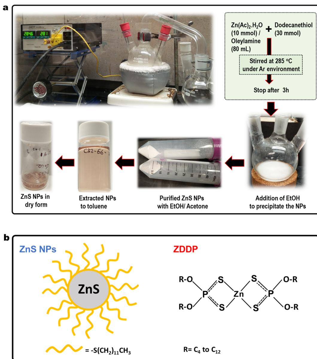
Fig. 1 (a) Pictures showing overall ZnS nanoparticle synthesis process, including setup, conditions, and processing. (b) Model structures of the ZnS NPs and ZDDP. The R represents an alkyl group in ZDDPs.
