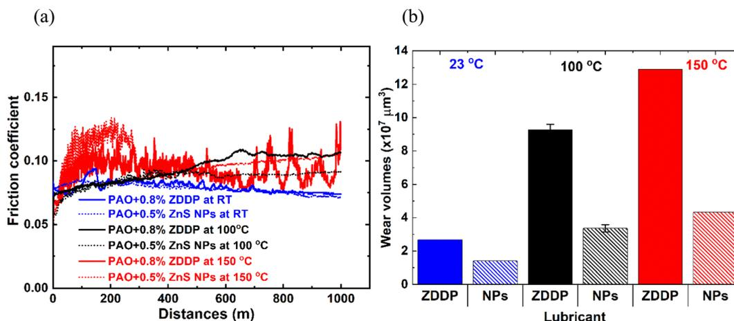
Fig. 5 Friction (a) and wear (b) performance of ZDDP and ZnS NPs at different temperatures, RT (23 °C), 100, and 150 °C.
