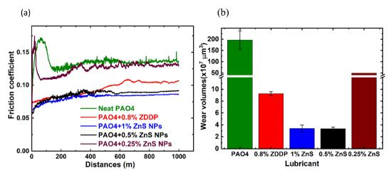
Fig. 4 Friction (a) and wear (b) performance of PAO4 and ZDDP compared to the ZnS NPs at 100 °C.
