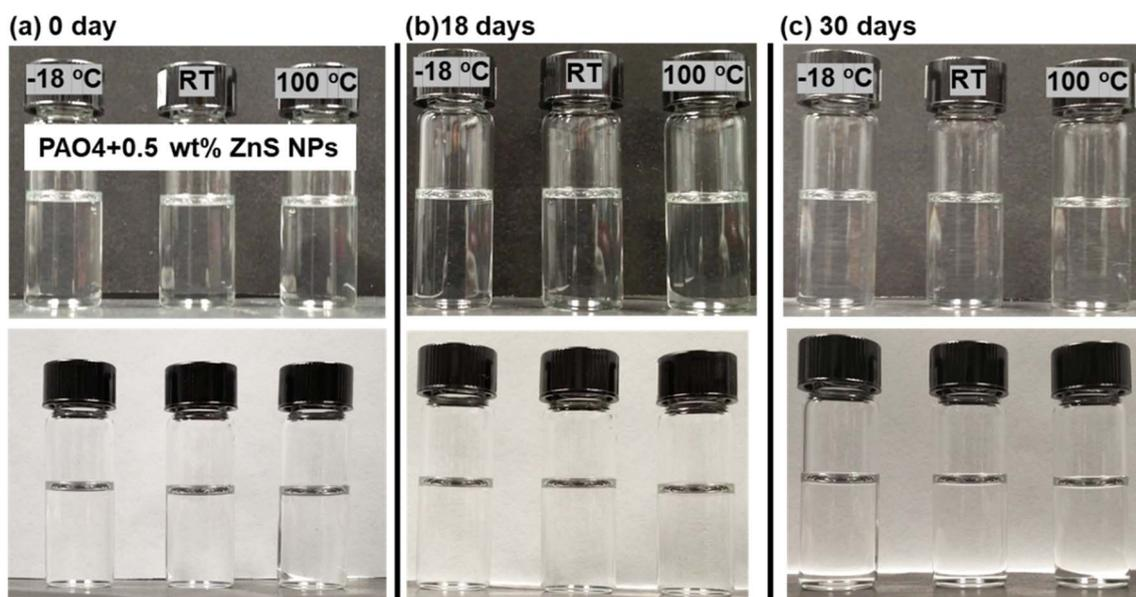
Fig. 2 Pictures showing PAO4 + 0.5 wt% ZnS NPs (a) initial state and after being kept at  $-18$  °C, RT and 100 °C for (b) 18 days and (c) 30 days. Black and white backgrounds were used to visualize the oil transparency.
