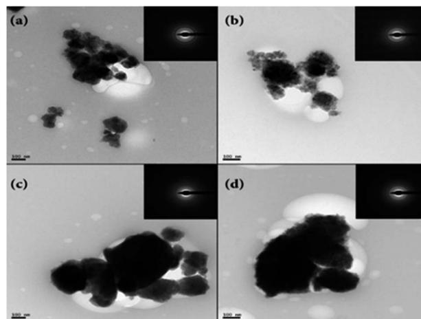
Fig. 4 TEM images and their corresponding SAED pattern of ball-milled (a)  $Mg_{0.8}Ti_{0.2}$  (b)  $Mg_{0.6}Ti_{0.2}Sc_{0.2}$  (c)  $Mg_{0.6}Ti_{0.2}Zr_{0.2}$  and (d)  $Mg_{0.6}Ti_{0.2}Nb_{0.2}$  alloy powders.
