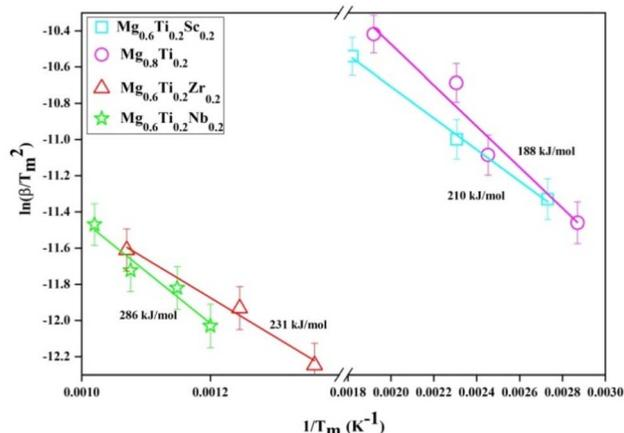
Fig. 7 Kissinger analysis of ball milled  $\text{Mg}_{0.8}\text{Ti}_{0.2}$ ,  $\text{Mg}_{0.6}\text{Ti}_{0.2}\text{Sc}_{0.2}$ ,  $\text{Mg}_{0.6}\text{Ti}_{0.2}\text{Zr}_{0.2}$  and  $\text{Mg}_{0.6}\text{Ti}_{0.2}\text{Nb}_{0.2}$  alloy powders.
