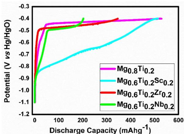
Fig. 10 Discharge curve of  $\text{Mg}_{0.8}\text{Ti}_{0.2}$ ,  $\text{Mg}_{0.6}\text{Ti}_{0.2}\text{Sc}_{0.2}$ ,  $\text{Mg}_{0.6}\text{Ti}_{0.2}\text{Zr}_{0.2}$  and  $\text{Mg}_{0.6}\text{Ti}_{0.2}\text{Nb}_{0.2}$  electrode materials.
