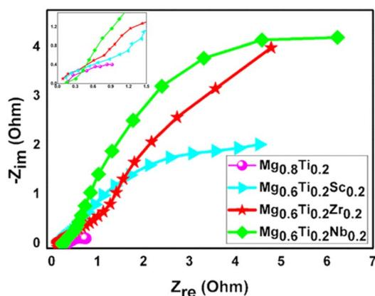
Fig. 9 Nyquist plots of  $\text{Mg}_{0.8}\text{Ti}_{0.2}$ ,  $\text{Mg}_{0.6}\text{Ti}_{0.2}\text{Sc}_{0.2}$ ,  $\text{Mg}_{0.6}\text{Ti}_{0.2}\text{Zr}_{0.2}$  and  $\text{Mg}_{0.6}\text{Ti}_{0.2}\text{Nb}_{0.2}$  alloys.
