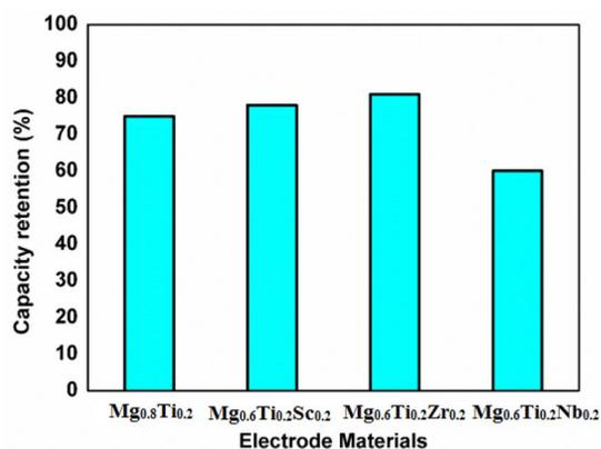
Fig. 12 Capacity retentions of  $\text{Mg}_{0.8}\text{Ti}_{0.2}$ ,  $\text{Mg}_{0.6}\text{Ti}_{0.2}\text{Sc}_{0.2}$ ,  $\text{Mg}_{0.6}\text{Ti}_{0.2}\text{Zr}_{0.2}$  and  $\text{Mg}_{0.6}\text{Ti}_{0.2}\text{Nb}_{0.2}$  alloys.
