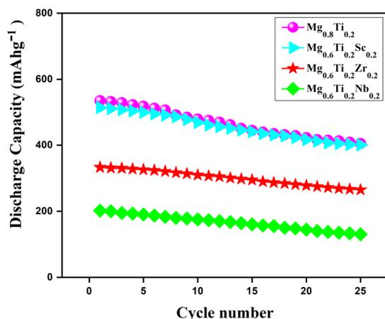
Fig. 11 Discharge capacity vs. cycle number of  $\text{Mg}_{0.8}\text{Ti}_{0.2}$ ,  $\text{Mg}_{0.6}\text{Ti}_{0.2}\text{Sc}_{0.2}$ ,  $\text{Mg}_{0.6}\text{Ti}_{0.2}\text{Zr}_{0.2}$  and  $\text{Mg}_{0.6}\text{Ti}_{0.2}\text{Nb}_{0.2}$  electrode materials.
