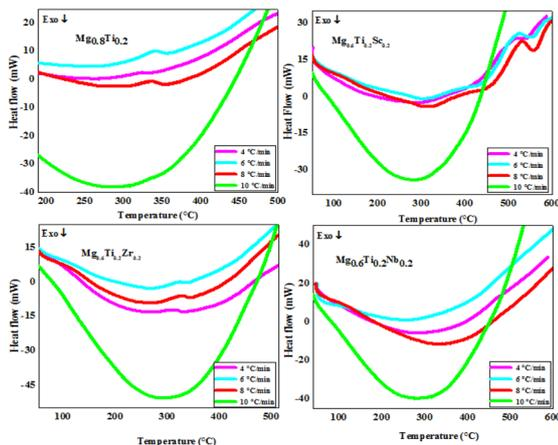
Fig. 6 DTA curves of ball milled (a)  $\text{Mg}_{0.8}\text{Ti}_{0.2}$  (b)  $\text{Mg}_{0.6}\text{Ti}_{0.2}\text{Sc}_{0.2}$  (c)  $\text{Mg}_{0.6}\text{Ti}_{0.2}\text{Zr}_{0.2}$  and (d)  $\text{Mg}_{0.6}\text{Ti}_{0.2}\text{Nb}_{0.2}$  alloy powders at different heating rates.
