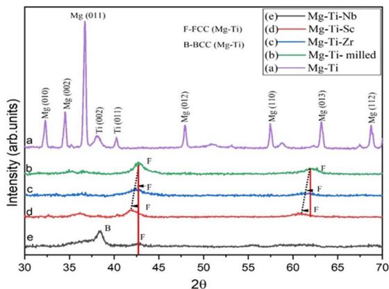
Fig. 1 Powder diffraction patterns of 30 h milled (a) pristine Mg<sub>0.8</sub>Ti<sub>0.2</sub> (b) Mg<sub>0.8</sub>Ti<sub>0.2</sub> (c) Mg<sub>0.6</sub>Ti<sub>0.2</sub>Sc<sub>0.2</sub> (d) Mg<sub>0.6</sub>Ti<sub>0.2</sub>Zr<sub>0.2</sub> (e) Mg<sub>0.6</sub>Ti<sub>0.2</sub>Nb<sub>0.2</sub> alloy powders.
