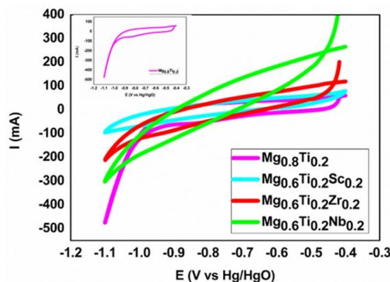
Fig. 8 Cyclic voltammetry curve of  $\text{Mg}_{0.8}\text{Ti}_{0.2}$ ,  $\text{Mg}_{0.6}\text{Ti}_{0.2}\text{Sc}_{0.2}$ ,  $\text{Mg}_{0.6}\text{Ti}_{0.2}\text{Zr}_{0.2}$  and  $\text{Mg}_{0.6}\text{Ti}_{0.2}\text{Nb}_{0.2}$  alloys.
