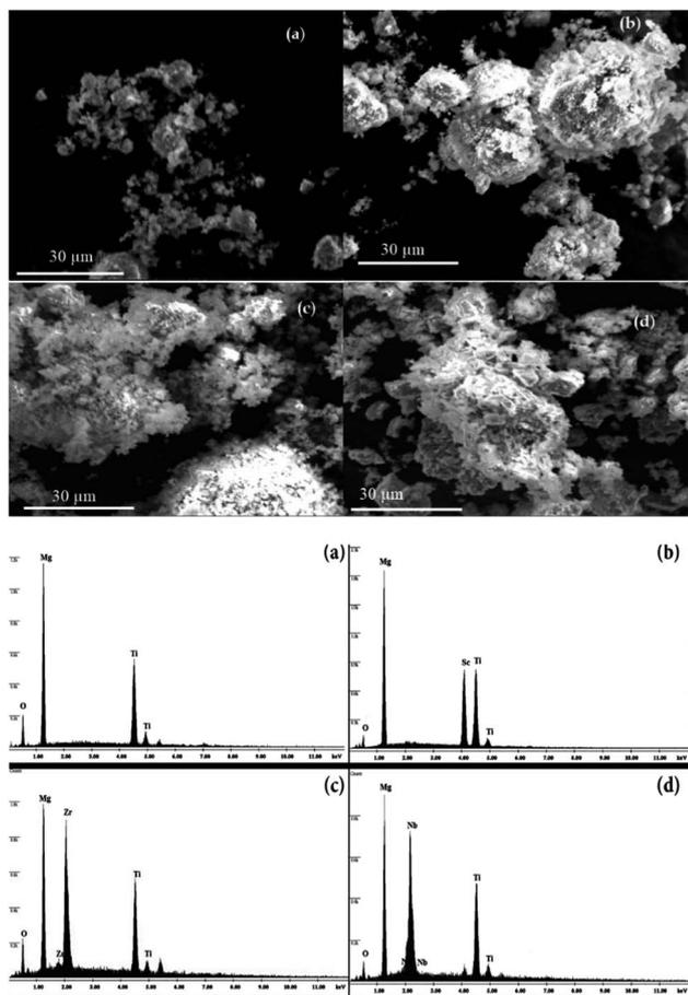
Fig. 3 SEM and their corresponding EDS images of ball-milled (a)  $Mg_{0.8}Ti_{0.2}$  (b)  $Mg_{0.6}Ti_{0.2}Sc_{0.2}$  (c)  $Mg_{0.6}Ti_{0.2}Zr_{0.2}$  and (d)  $Mg_{0.6}Ti_{0.2}Nb_{0.2}$  alloy powders.
