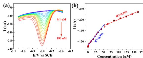
Fig. 7 (a) DPV curves of 4-NP with increasing concentration (0.1–180  $\mu\text{M}$ ) in 0.2 M PBS (pH = 6.4); (b) calibration plot of 4-NP versus concentration. Potential window:  $-0.6$  to  $-1.05 \text{ V}$ . Scan rate:  $50 \text{ mV s}^{-1}$ .
