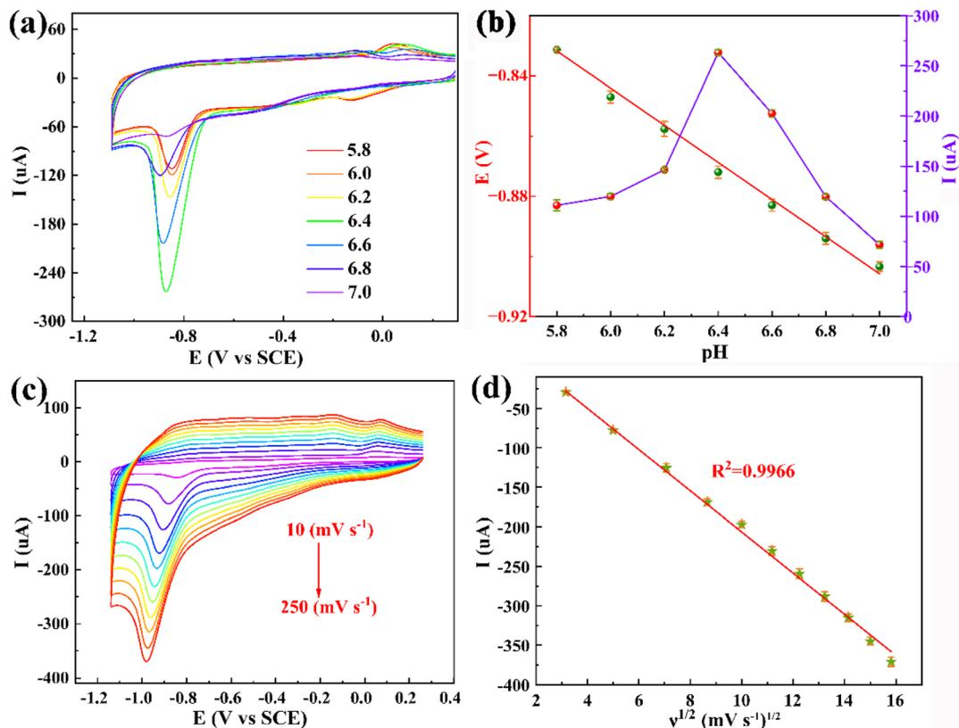
Fig. 6 (a) CVs of 0.1 mM 4-NP at PDPP-GO/GCE at various pH from 5.8 to 7.0, the scan rate is  $50 \text{ mV s}^{-1}$ ; (b) linear relationship of  $E_{\text{pc}}$  versus pH value and the plot of  $I_{\text{pc}}$  versus pH value. (c) CVs of the PDPP-GO/GCE for 0.1 mM 4-NP in 0.2 M PBS at various scan rates: 10–250  $\text{mV s}^{-1}$ , (d) the plots of cathodic peak currents vs.  $v^{1/2}$ . Potential window: 0.25–1.13 V.
