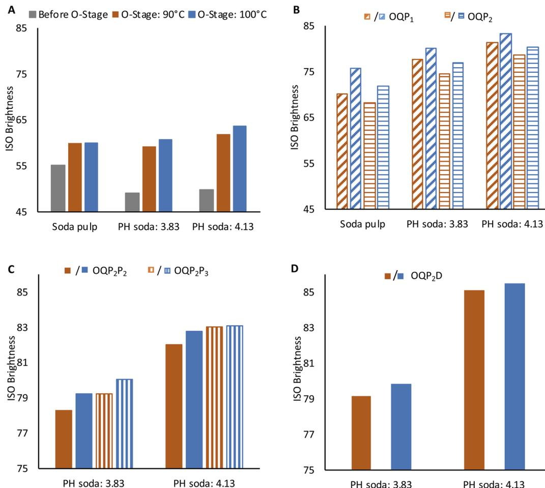
Fig. 4 ISO brightness of pulps before and after oxygen (O) bleaching (A) after OQP<sub>1</sub> and OQP<sub>2</sub> (B), after OQP<sub>2</sub>P<sub>2</sub> and OQP<sub>2</sub>P<sub>3</sub> (C) and after OQP<sub>2</sub>D (D) (temperature of O-stage in the sequences are indicated by ■ for 90 °C and ■ for 100 °C).
