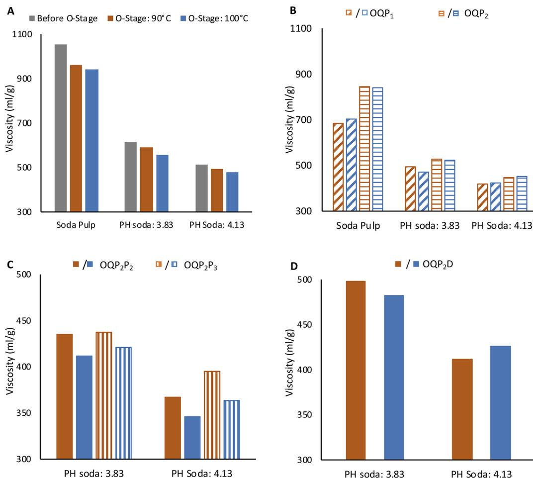
Fig. 3 CUEN viscosity of pulps before and after oxygen (O) bleaching (A) after OQP<sub>1</sub> and OQP<sub>2</sub> (B), after OQP<sub>2</sub>P<sub>2</sub> and OQP<sub>2</sub>P<sub>3</sub> (C) and after OQP<sub>2</sub>D (D) (temperature of O-stage in the sequences are indicated by orange for 90 °C and blue for 100 °C).
