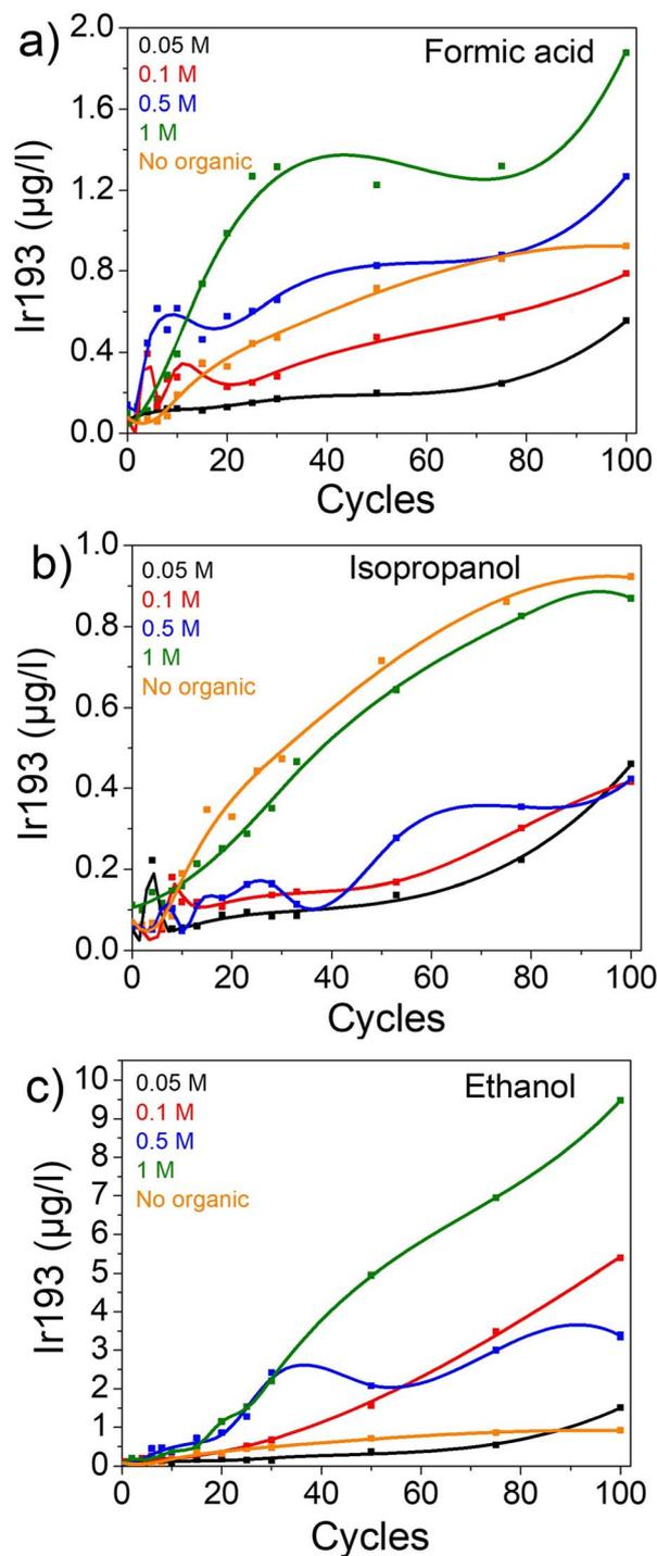
Fig. 1 Dissolution of iridium in different concentrations of organics in 0.1 M HClO<sub>4</sub>. (a) In formic acid. (b) In isopropanol. (c) In ethanol.
